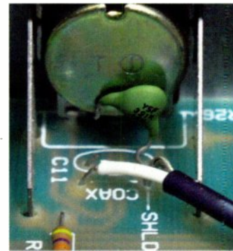
Figure-3: The Master Volume control and its lowpass filter C11.
