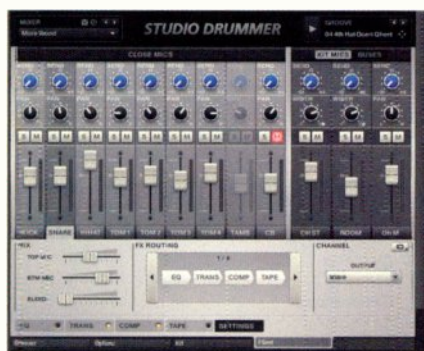
Fig. 2: Studio Drummer's integrated mixer adjusts levels and panning, inserts effects, and includes a solo and mute for each channel.
