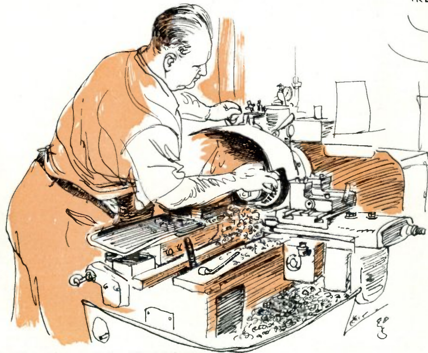
CLOSE LIMITS MUST BE MAINTAINED THROUGHOUT THE SOME 150 MACHINING OPERATIONS NECESSARY TO MAKE THE SOME 374 PARTS THAT MAKE THE AVERAGE F. H. P. MOTOR
