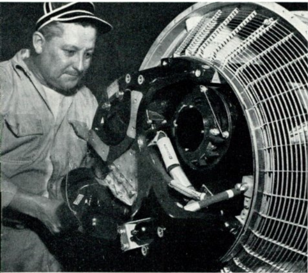
The finishing touches are put on the front end of a J-47. An improvement has recently been made in the screen through which air enters the engine.
