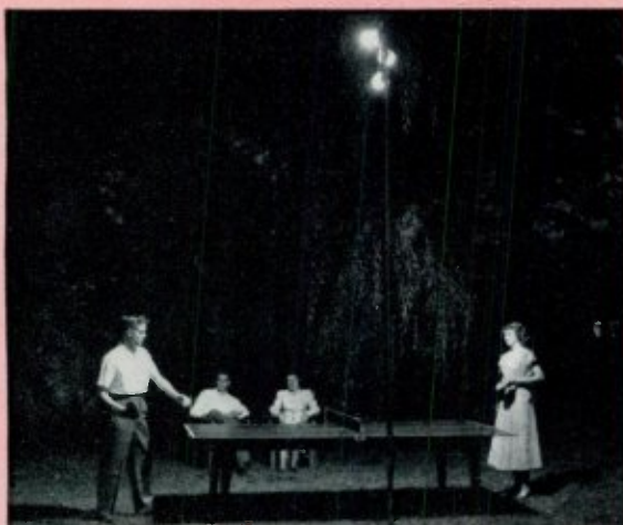
For table tennis, three 300-watt reflector floodlamps on the standard 12-foot pole give 40-70 footcandles on table.
