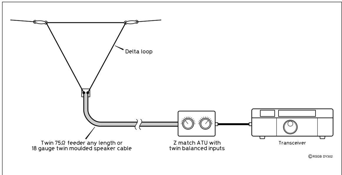
Fig 1: Multiband version of the delta loop connected to the ASTU using 75Ω twin feeder.
