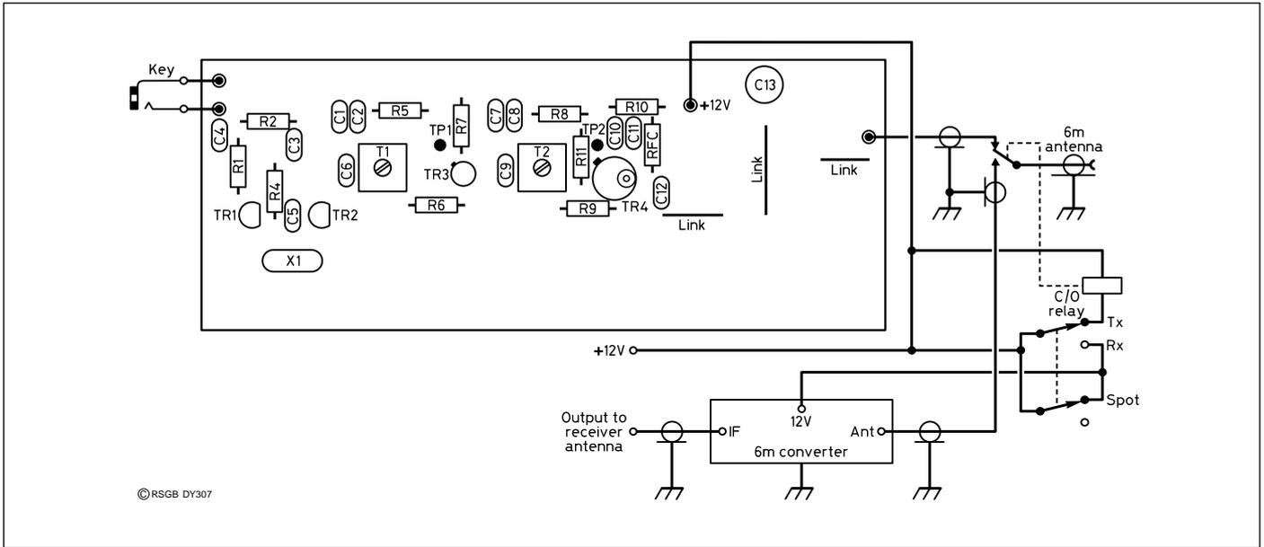
Fig 2: Layout of the components and antenna changeover relay. This is also shown with the 6m converter; see text.
