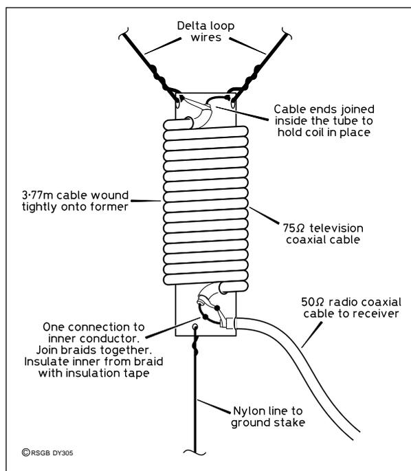
**Fig 4: Detail of the 20metre band coaxial balun.**
