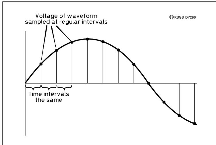
Fig 3: Sampling an analogue waveform.
