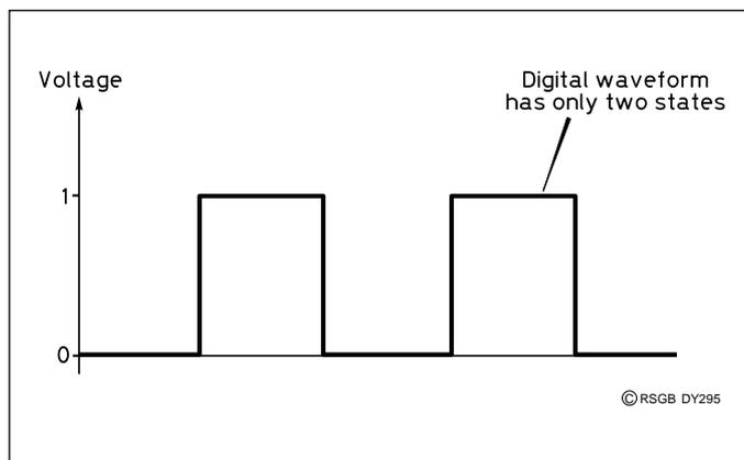
Fig 2: A Digital waveform - serial data.
