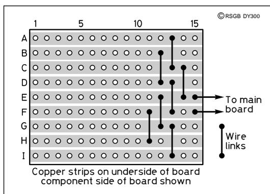
Fig 2: Layout of the main board.
