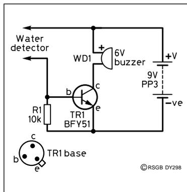
Fig 1: Circuit diagram of the water level detector.
