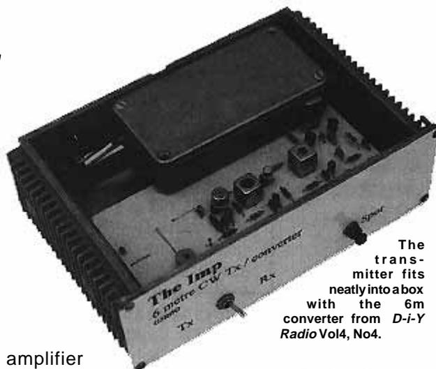
The transmitter fits neatly into a box with the 6m converter from *D-i-Y Radio Vol4, No4*.
