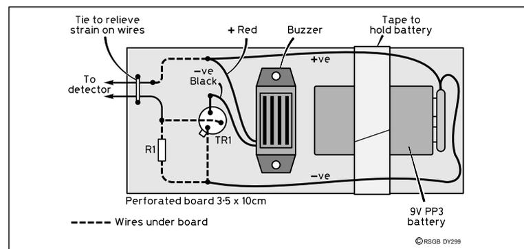
Fig 3: Water detector constructed from stripboard.
