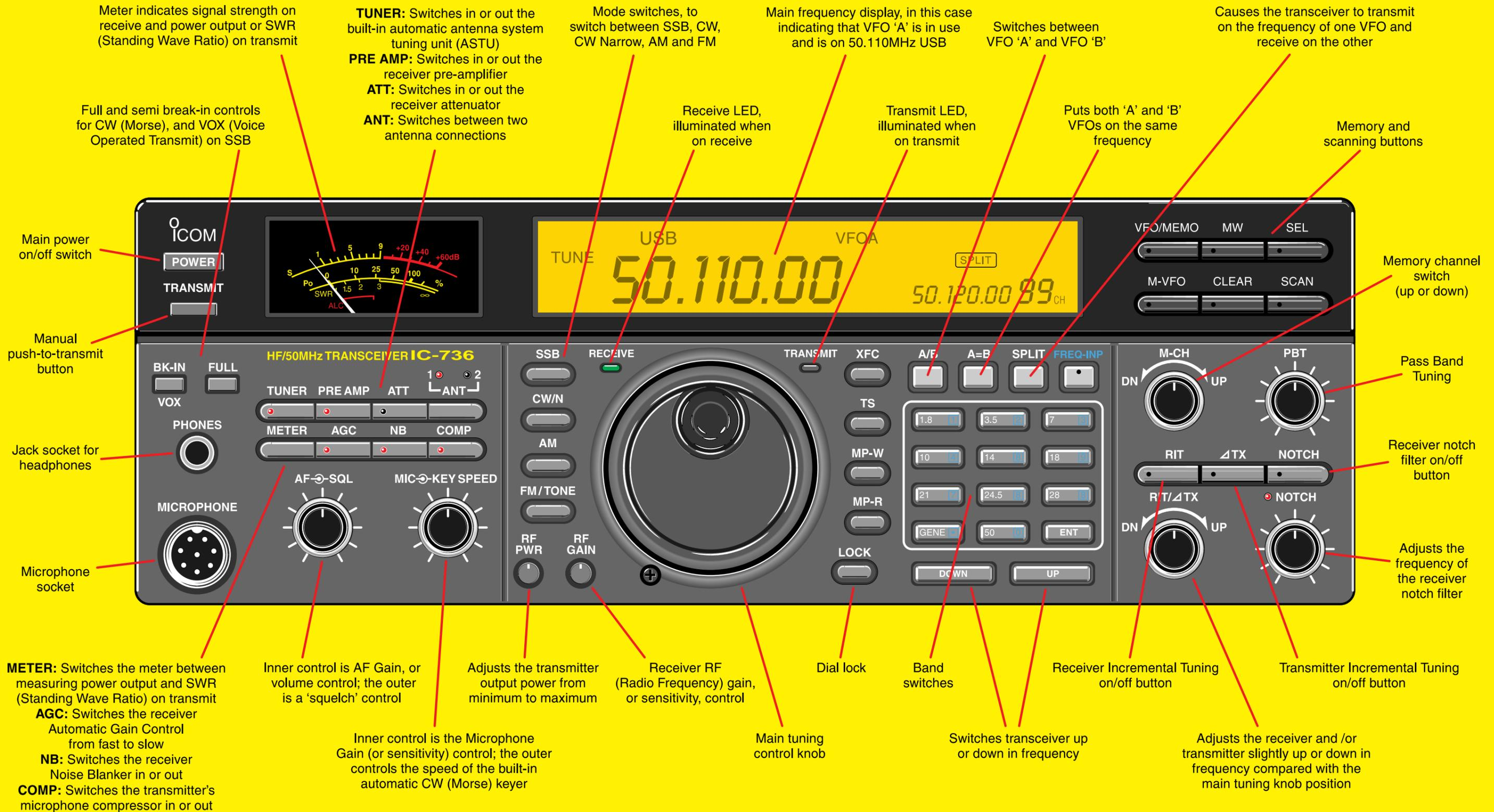
Many HF and VHF transceivers can look very complicated at first glance. However, all the controls have a logical function, and these are described above with the aid of the drawing of an Icom IC-736 transceiver, which covers all the HF bands (1.8 - 28MHz) plus the 6m (50MHz) band.
