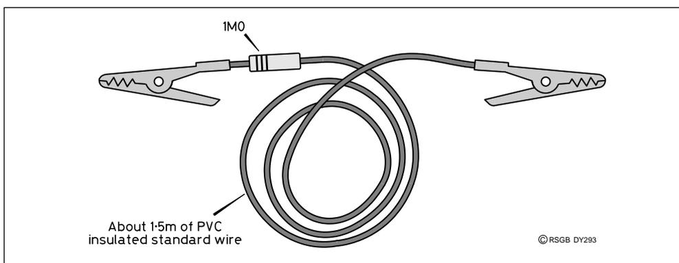
**Fig 3: A home made anti-static earth lead.**
