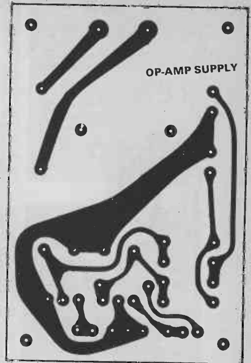
Component positioning and foil pattern for a suitable power supply (60 x 90 mm).
