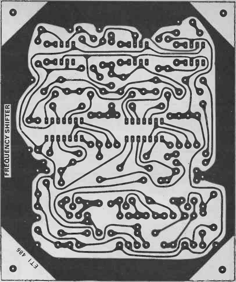
Fig. 4. Oscilloscope showing output of IC3 (upper) and IC4 (lower); signal is 100 Hz, note phase difference. Below, full size foil pattern for the shifter (120 x 100 mm).
