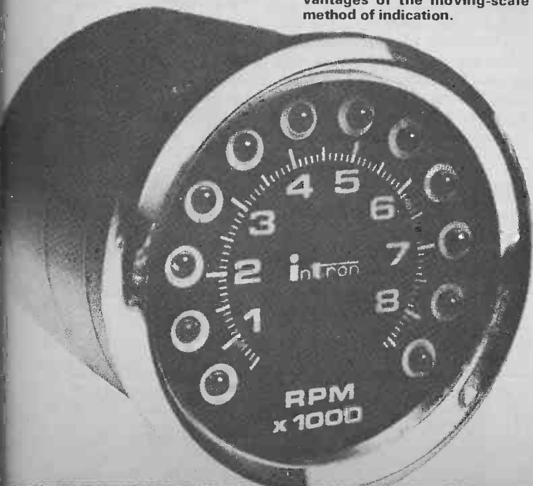
Fig 7. Needle indicators will soon disappear from the dash panel. They will be replaced by solid-state light-emitting diode "scales" that preserve the advantages of the moving-scale method of indication.
