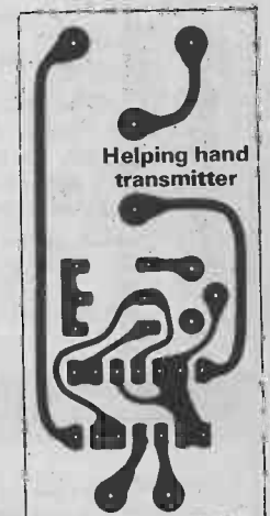
Above is the foil pattern of the transmitter and to the right that of the receiver, both shown full size.
