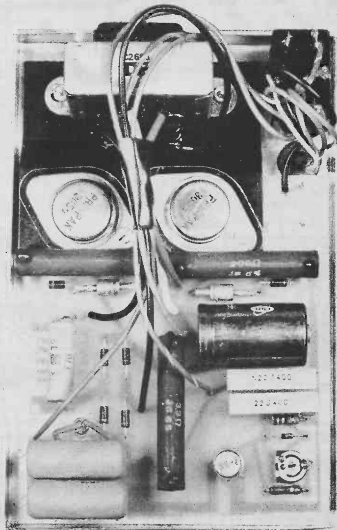
View of the completed system. Note the insulating washers under each of the two transistors.
