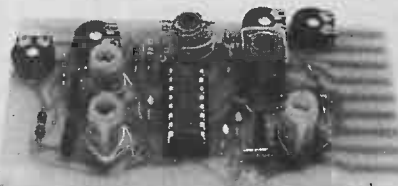
The EF5400, a 4 stage varicap tunerhead, tuning 88-108MHz with a bias swing of just 2 - 8 volts DC. A single IC provides all functions, including PIN diode AGC drive, balanced mixer, RF amplifier. All this and edge connection too! £9.75 built.
