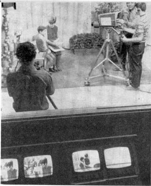
Cable operators now generate their own live programs on one channel. This TeleMation-equipped studio cablecasts black and white.
