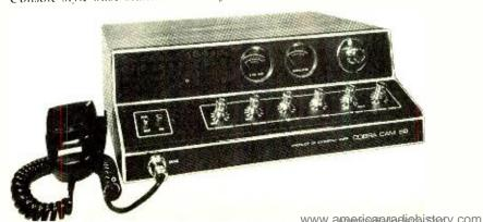
THE Dynascan Corp. Cobra CAM 89 is a somewhat different kind of AM base-station CB transceiver as a result of its console-like design and greater number of controls than is usually the norm. Except for the channel selector, the controls are located in a row across the front panel's lower half that slopes away at about a 30° angle. These controls are for microphone gain (DYNAMIKE), VOLUME and
