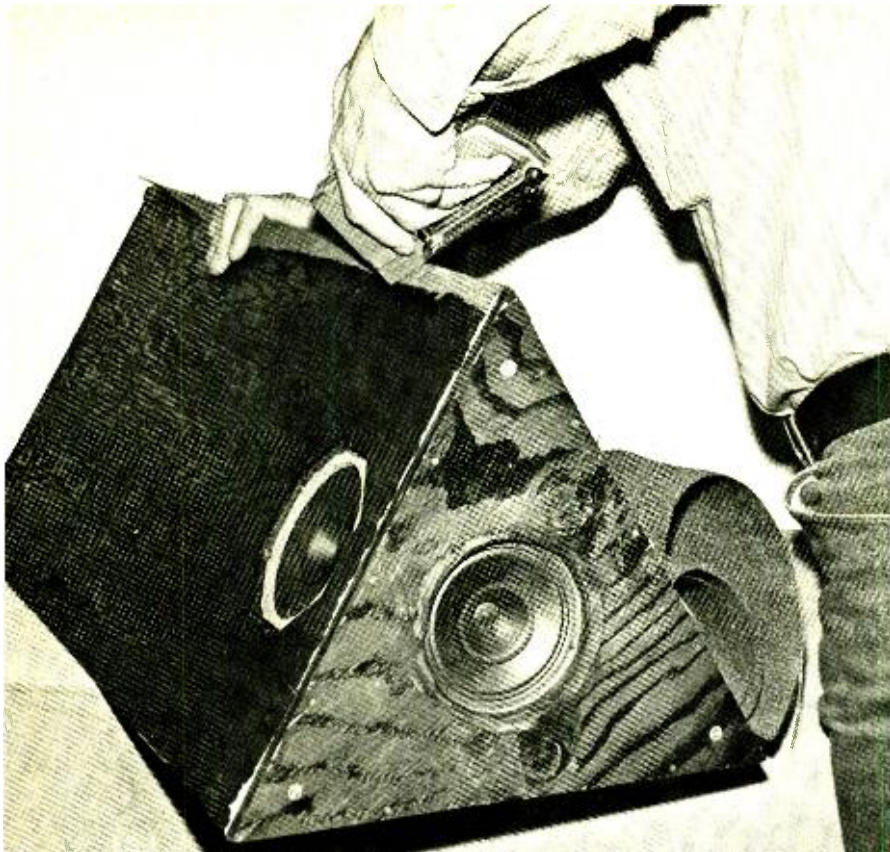
Fig. 6. Start installing wrap-around grille by stapling it to the rear corner.
