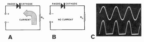
Fig. 1. Forward-biased diode (A) conducts current while reverse-biased diode (B) does not. In (C), upper trace is ac input, lower trace is pulsating dc across load.
