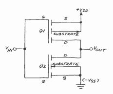
Fig. 1. Basic CMOS gate.
