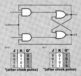
Fig. 14. The JK flip-flop is a clocked RS flip-flop that allows a logic 1 to be simultaneously applied to both inputs. Shown here is a NOR gate version with truth tables for Q = 0 and Q = 1.
