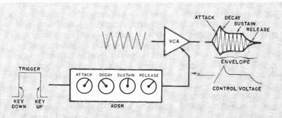
Fig. 5. The combination of a vca and ADSR.
