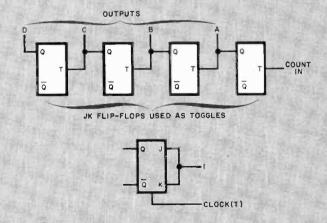
Fig. 16. A four-bit counter made from T flip-flops that will count from 0000 to 1111 and then recycle.
