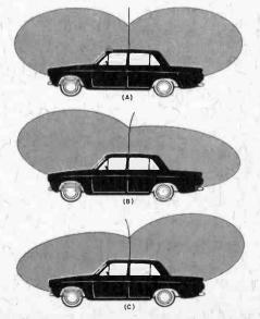
A full-size quarter-wave whip working against a good ground plane will easily cover the 40 CB channels while maintaining an acceptable match. However, a very short miniwhip will have difficulty presenting a matched impedance over even the original 23 channels. Most midsize whips can be used on 40 channels if tuned for the best impedance match at the center of the band.
