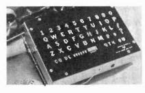
S.J. Engineering's Model SMCT simulated Morse-code: typewriter lets an aspiring ham radio operator learn and send Morse code simply by touching a built-in probe to selected letters and numerals. Once a
