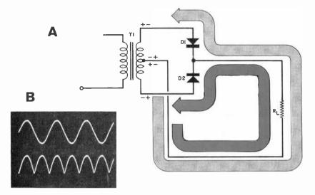
Fig. 2. At (A) is fullwave rectifier. Ac in primary of T1 is upper trace in (B), pulsating dc is at bo'tom.
