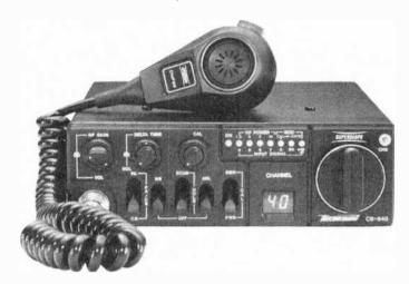
THE Superscope Aircommand 40-channel mobile AM CB transceiver departs from convention, as do a few others, by indicating relative signal strength, output power, etc., with a row of LED's instead of a meter. Another special feature is channel 9 scanning with individual squelch control and an audible alarm that sounds whenever a signal appears on channel 9.
