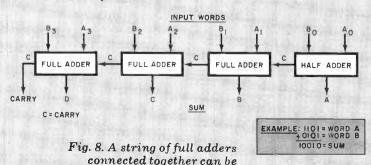
used to form a binary adder,
