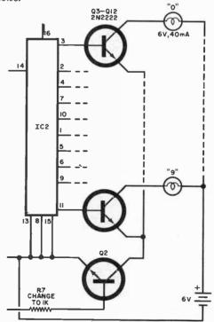
Fig. 5. Modifying the Wheel of Fortune for use with conventional 6 volt lamps.
