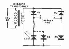
The LED will glow only when the iron is in the stand and making contact with the charger's output pins. Diodes D1 through D3 must be able to handle the maximum charging current. My "quick charge" iron draws about 440 mA maximum, so 1N4002's are suitable. A standard TIL-32 or similar LED can be used. Resistor R1 is selected to limit LED current to a safe value. My charger has a 3-volt secondary, so I used a 330ohm, 1/2-watt resistor.
