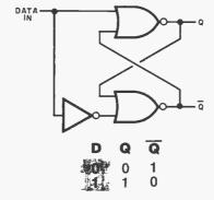
Fig. 13. A data, or D, flip-flop is made by adding an inverter to input of one flip-flop.
