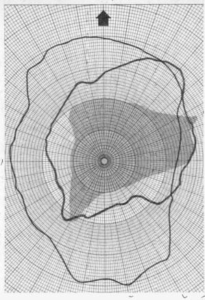
more away from each other, fed with properly phased feedlines, and there are no vertical conductors within a two-wavelength radius, some gain and a figure-eight radiation pattern (favoring fore and aft) will be obtained: CB'ers have attempted to take advantage of this by mounting twin whips on truck or camper
