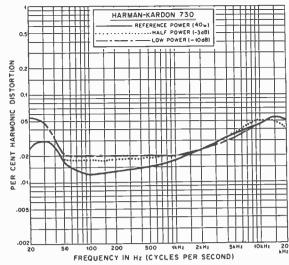
Harmonic distortion at three power levels.
