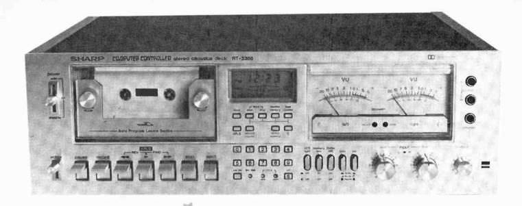
also identifies the specific tapes for which the deck was adjusted at the factory. They are Maxell UD (normal), Maxell UD-XL II (HIGH/70  $\mu$ s), and Sony Ferrichrome (LOW/70  $\mu$ s).
