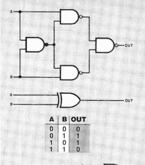
Fig. 5. The combinational circuit at top provides an Exclusive-OR, as shown in the middle. The truth table is below.
