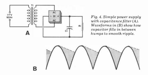
ploys the entire secondary potential, it produces an output potential (pulsating dc) of twice that of the ordinary full-wave rectifier using the same transformer. There is one catch, however. The bridge rectifier supply delivers only half the current of the full-wave rectifier for a given primary VA rating. There are occasions when it is possible to exceed this and draw nearly the full rated current from the transformer's secondary without causing damage, but this is not dependable in all cases.
