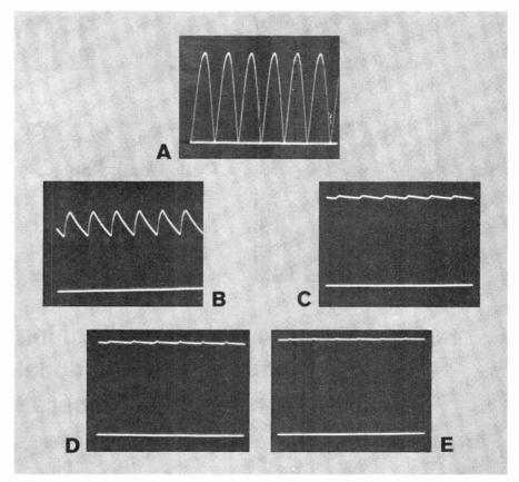
Fig. 5. How capacitors smooth waveform. Lower trace is zero volts. (A) is full-wave dc without filter; (B) has  $150-\mu F$  capacitor; (C)  $2000 \mu F$ ; (D)  $5000 \mu F$ ; (E)  $18,000 \mu F$ .
