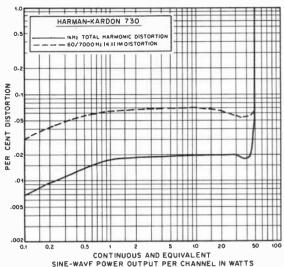
Total harmonic distortion and 60/7000-Hz distortion.
