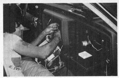
Installing a mobile CB rig is not usually a major undertaking. It can be challenging, though, when an AM/FM electric-powered antenna is replaced by a CB/AM/FM one since auto radio must be removed to make power connections.
