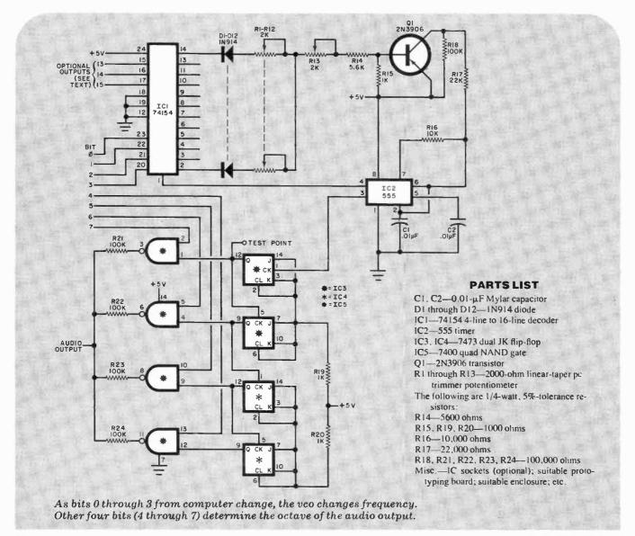
grammed to generate a mix of tones, up to a total of 16, for use as test and remote-control signals.
