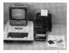
A Microproducts board interfaces an Apple II with an SWTP PR-40.
