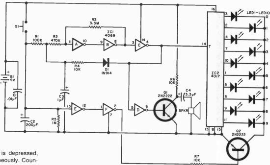
When the pushbutton is depressed, two things occur simultaneously. Counter *IC2* is reset to zero by the signal on pin 2, thus placing all of the *IC2* outputs at their low states (0 volts). Thus, none of the LED's can glow. The second action is an enable level signal (+9 volts) at pin 13 of *IC1*. This action allows the oscillator (the middle two gates) to start, thus producing an input signal to the counter IC through the last gate of *IC1*.
