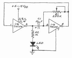
Fig. 2. Astable multivibrator. that a particular CMOS device is protected, play it safe and handle it carefully.
