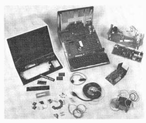
Hazeltine's Model 1500 computer terminal comes in semikit form as shown here and is easily assembled.
