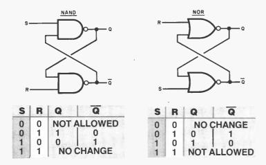
Fig. 11. Simplest flip-flop is made from two NAND's or two NOR's with truth tables as shown.
