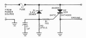
Fig. 9. Crowbar overvoltage protection circuit "fires" when 5-volt line exceeds breakdown voltage of zener diode.
