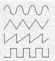
Fig. 2. Typical vco waveforms.
