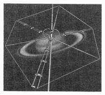
yield an omni-directional radiation pattern. The feed system is arranged so that equal power is applied to each dipole, via separate multipurpose balun coils. The method by which the power is equally divided and transferred to the dipole radiators is the heart of the Saturn's design.
