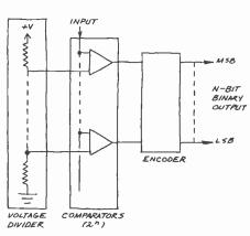
Fig. 1. Block diagram of parallel or flash A/D converter.
