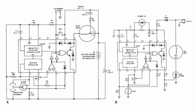
Fig. 3. Smoke detector circuits using National's LM1801: (A) ionization-chamber type, and (B) photoelectric type.
