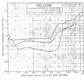
Percent harmonic distortion at three power levels at 8 ohms.
