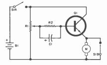
Fig. 4. Reader's dc motor control circuit with accelerator and braking action.
