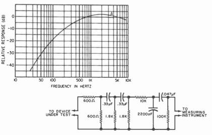
Fig. 5. The "A" weighting curve (top) reflects the ear's sensitivity vs. frequency at listening level of 70 phons. Circuit below provides "A" weighting and matches 60-ohm output to high-impedance instrument.
