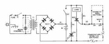
Fig. 1. Combination fire and burglar alarm circuit.
