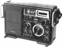
THE SOLID-STATE portable Model RF-2800 receiver from Panasonic provides continuous coverage of the 3.2-to-30-MHz shortwave bands and also covers the standard AM and FM broadcast bands. SW coverage is in five selectable bands.
