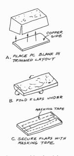
Fig. 5. Cover pc blank with trimmed artwork (A), fold flaps under (B), secure with tape (C).
