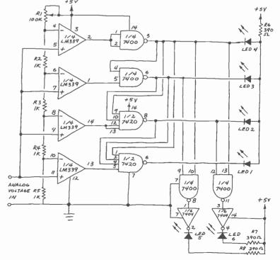
Fig. 5. An A/D converter with binary output is made by adding a 2-bit encoder as shown here.
