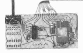
Two-chip, four-channel converter works with any 8-bit computer.
