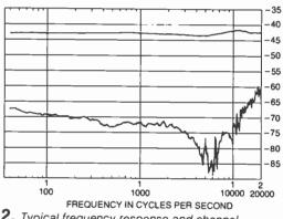
2. Typical frequency response and channel separation curves of the XSV/3000.
