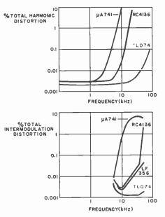
Fig. 1. TI's TL074 BIFET op amp generates less distortion than common bipolar linear IC's.
