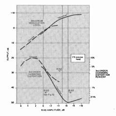
Fig. 2. Maximum modulation and harmonic distortion levels.
