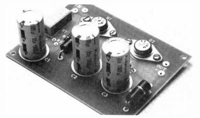
Photo shows layout of author's prototype filter.
