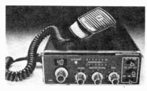
through the use of twin ceramic selectivity filters, switchable noise-blanker/ANL system. Controls include three-position range switch, delta tune switch, tone, CB/PA switch, and calibrated squelch. The Viking 260's cabinet is covered with leather-textured black vinyl (other colors available). \$199.95.
