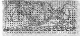
Photos of the front and back of the prototype project show how Wire-Wrapped connections were used. It was assembled on perforated board with copper solder pads and bus strips.
