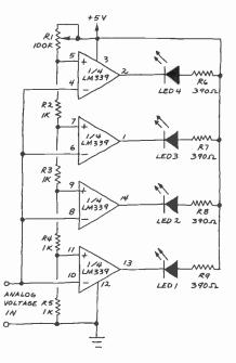
Fig. 3. LED thermometer-style bargraph readout.
