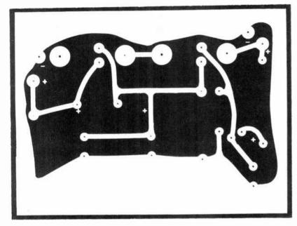
Fig. 2. Full-size foil pattern for filter pc board and component placement diagram are shown above.
