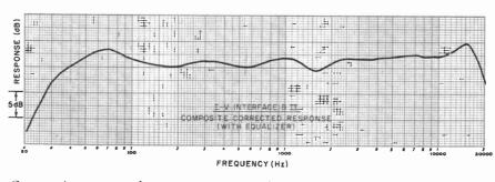
Composite corrected response curve with equalizer.
