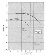
Fig. 1. Maximum output levels as function of bias.
