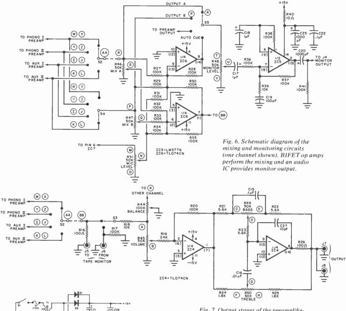
Fig. 7. Output stages of the preamplifier for one channel. Conventional bass and treble tone controls are included, as well as a tape monitor loop.
