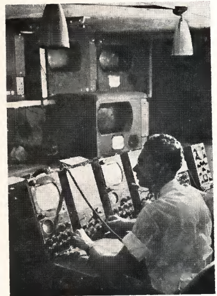
EACH camera control has an auxiliary color shading unit. Here a video man is shown operating this unit at CBS Studio 57.
