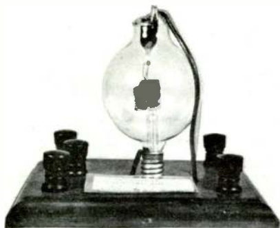
DE FOREST SPHERICAL AUDION SINGLE GRID & PLATE 1909
