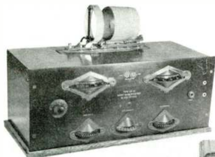
GREBE CR-18 10 TO 200 METERS ONE OF THE FIRST 10 METER RECEIVERS 1926 $100.00
