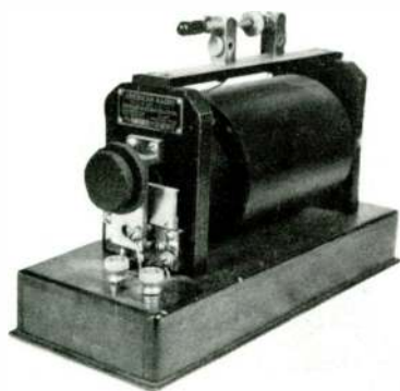
AMRAD TYPE C SPARK INDUCTION COIL MADE FOR U. S. ARMY IN 1918.
