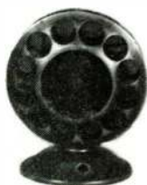
WESTERN ELECTRIC SINGLE BUTTON WITH STAND
