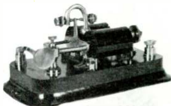
SENSITIVE RELAY USED WITH COHERER DET. 1910
