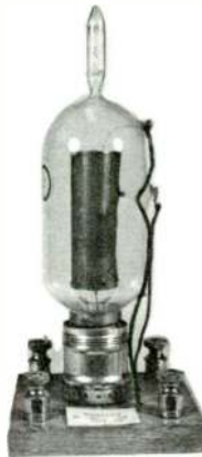
MARCONI TUBE MADE BY H. J. ROUND 1911
