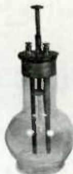
BICHROMATE BATTERY PLUNGER TYPE ABOUT 1900
