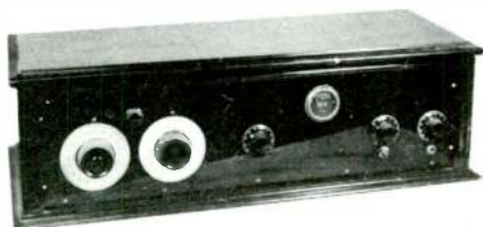
REMLER 9 TUBE SUPER 45 KC. IFs 1925 KIT $90.00
