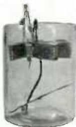
"CROWFOOT" GRAVITY BATTERY USED FOR TELEGRAPH AND WIRELESS 1905
