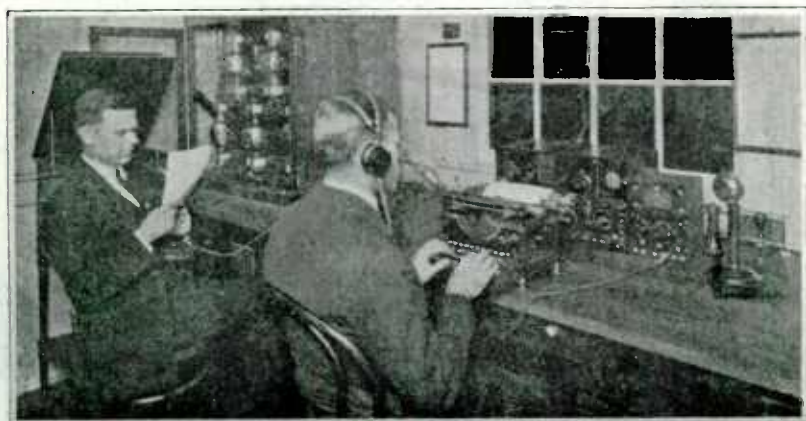
The "announcer" of a radio-phone broadcasting station, and the receiving operator. The announcer speaks into the microphone transmitter which he holds in his hand. Alongside of his is the radio-phone transmitting apparatus, with the vacuum tubes for generating and modulating the radio waves. This is WJZ, the Newark radiophone.
