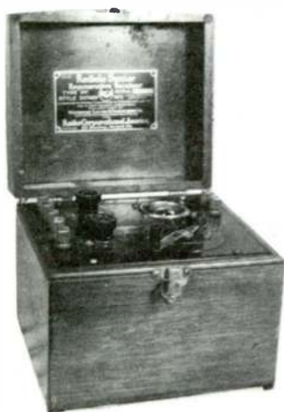
RADIOLA SENIOR TYPE RF REGEN. USES WD-11 TUBE MADE BY WESTINGHOUSE 1923 S.P. $65.00
