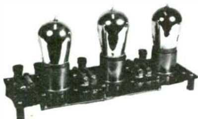
MUTER RES. COUP. AUDIO AMPLIFIER WITH TUBES $21.00
