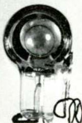
WESTERN ELECTRIC 239 A DETECTOR AMPLIFIER 1923
