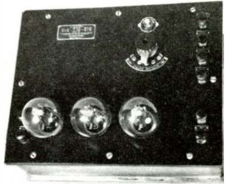
WESTERN ELECTRIC 7-A AMPLIFIER WITH 216-A TUBES
