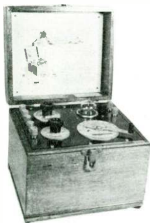
AERIOLA SR. RECEIVER REGENERATIVE USES WD11 MADE BY WESTINGHOUSE 1922 S.P. $65.00
