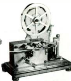
BRANLEY COHERER AND DECOHERER WITH KEY WIND TAPE PRINTER ABOUT 1902 TO 1905
