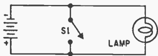
Fig. 3. This logic circuit for a demonstration of NEGATION or INVERSION is simple but not very practical—battery is shorted.
