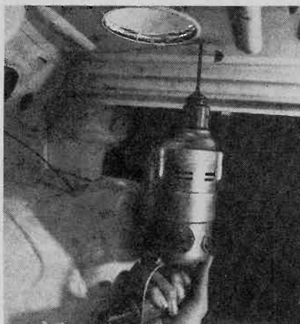
Fig. 7. Here's how it looks from inside the trunk. Note that in this car even the speaker mounting holes are pre-punched. Just drill through the rear deck cover from the trunk side. The metal tabs at the rear hold the speaker wires when they are bent upwards.
