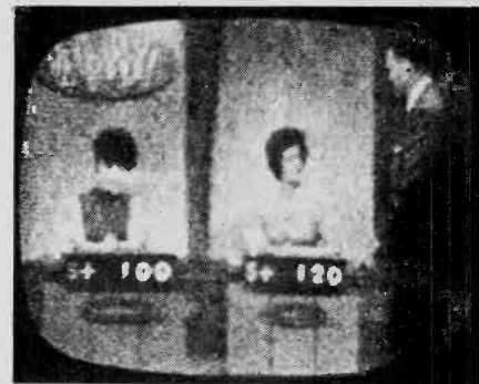
Fig. 3. Snow in the picture. Weak signal. This may indicate antenna trouble.
