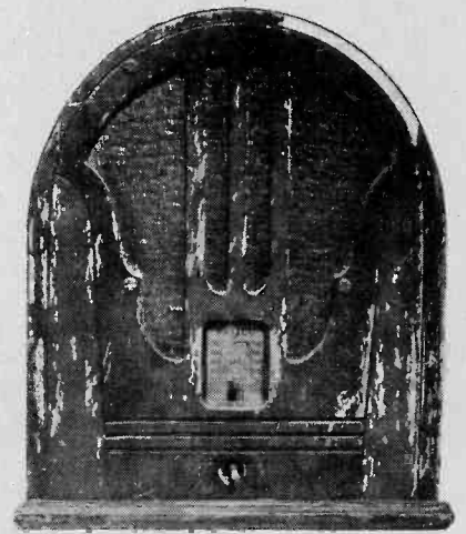
Fig. 2. This Philco cathedral radio came from a landfill. The veneer and finish have peeled, making it difficult to restore. Perhaps it will end up as a parts radio instead.
