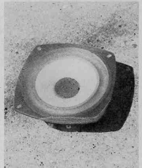
Fig. 5. If you cut and wrap the pantyhose carefully it should look like a factory installation.
