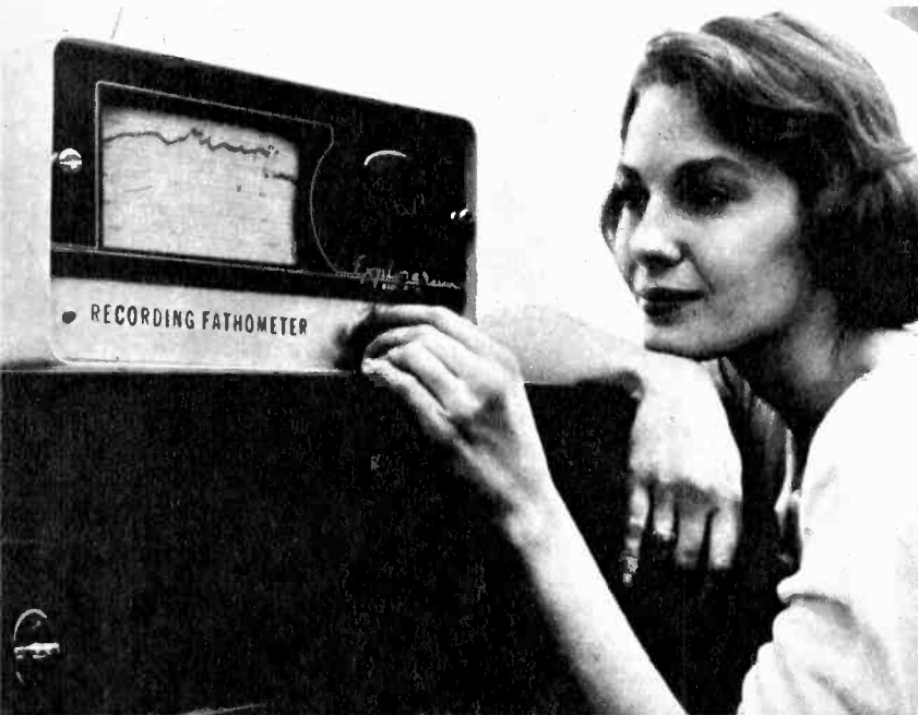
Recording Fathometer for small pleasure boats can tell operator at a glance the depth of water plus the contour of the bottom.
