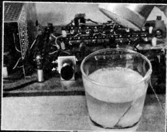
Detecting element (above) can be made by stripping the ends of a pair of wires, keeping them closely spaced.
