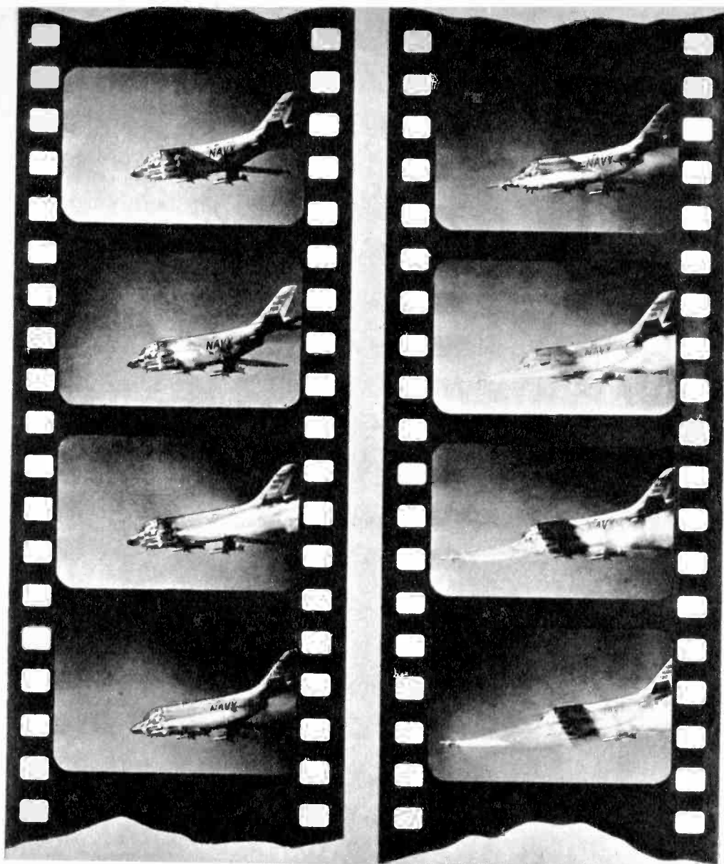
Rapid fire sequence shows Sparrow III, Navy air-to-air missile, being launched from F3H-2 Demon interceptor. Plane carries four missiles which are fired at target automatically when within range.
