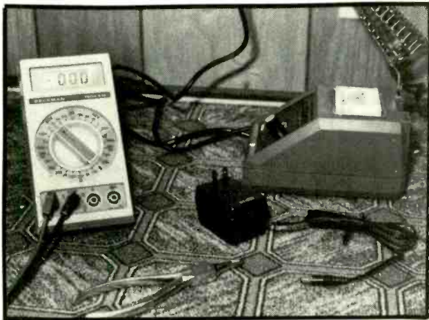
Figure 11. Inspect the cord and plug of the AC adapter for possible breaks or torn areas. Check for AC voltage at the plug end.
