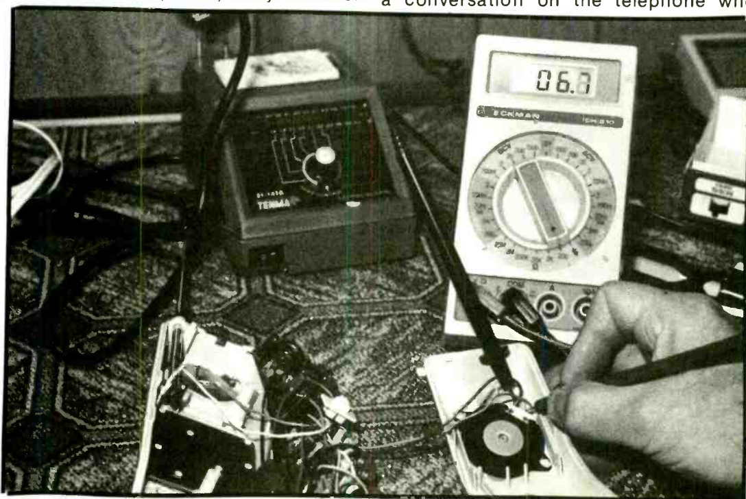
Figure 9. If the microphone is suspected, measure the resistance across the two terminals.
