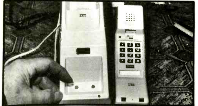
Figure 6. Clean off all charging contacts on the cordless phone and the base unit.
