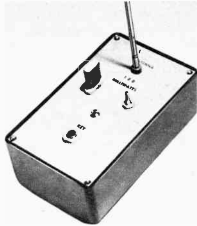
Transmitter is a neat package. Be sure antenna is extended fully before starting the tune-up.
