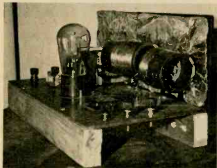
Breadboard AMer with 27 tube in place has tinfoil on rear of front panel to reduce capacitance effect of hand when you tune.
