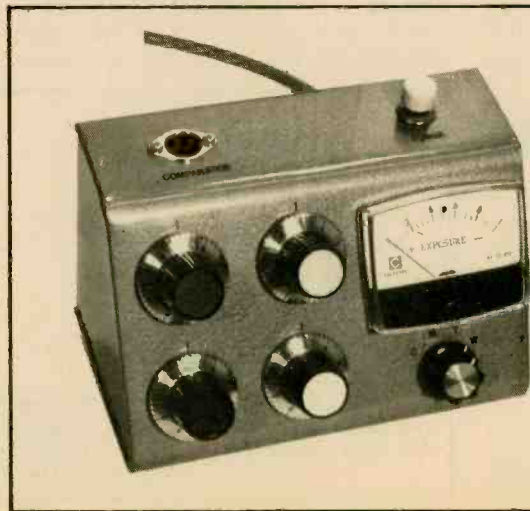
To avoid upsetting a control setting while groping for the on-off switch in the dark-room, mount switch S2 as far as possible from the controls.
