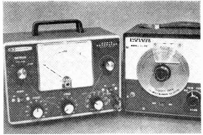
AUDIO GENERATORS You have a wide choice of audio generators. You can buy either wired units or kits, and sine-wave or sine-plus-square-wave generators. The instrument at left is the popular Heathkit IG-72 (kit and sine-wave) while the unit at right is the Lafayette TE-22 (wired and sine/square).
