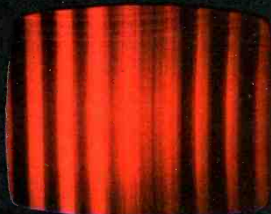
HUE CONTROL Proper setting blends sixth bar into background. Kill green and blue guns to obtain this display.
