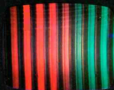
HUE CONTROL Proper setting blends sixth bar into background. Kill green and blue guns to obtain this display.
