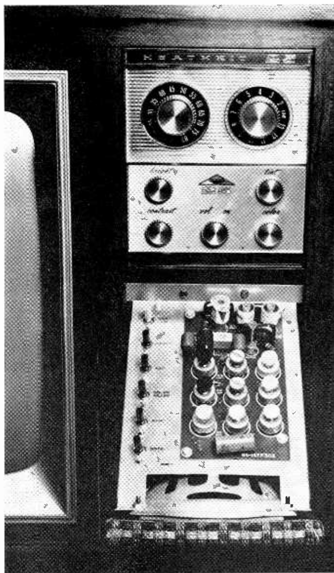
FRONT PANEL controls of a color set can be adjusted by a child; but once the convergence control board is unlocked, keep the children away. Up-front controls do away with mirrors. This Heathkit GR295 also has a built-in dot generator.
