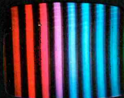
COLOR BAR PATTERN Normal display is indication of proper operation of phase, matrix, and other circuits.
