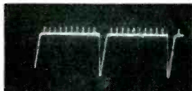
Complete absence of any back porch necessitates readjustment of brightness, contrast and fine tuning to obtain a usable pattern.
