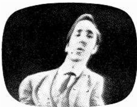
Fig. 13. The picture at left is weaving from side to side. On occasion hum bars may be visible. Check for grid defects in the r.f. and i.f. tubes, improper a.g.c. action, and anything that might upset the relationship between the amplitudes of the sync and video signals in the set.
