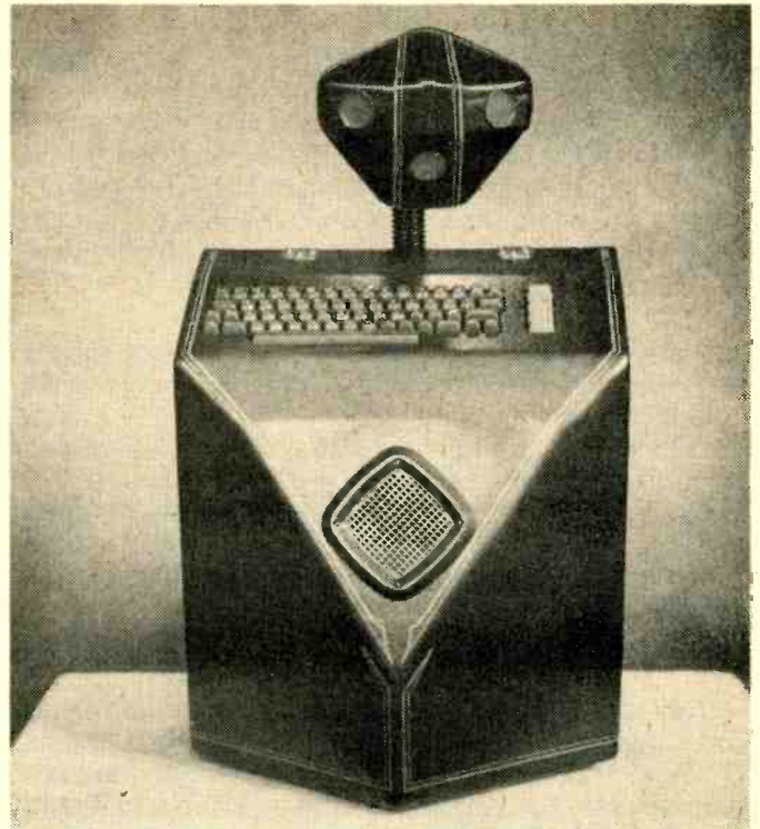
Robodroid (above) includes micro keyboard for programming moveable "head" which speaks and converses through speaker.
