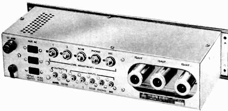
Fisher preamplifier is cut in the rear to allow easy changing of the three amplification tubes. Note the five inputs, each with its own level control, and the separate outputs to amplifier or tape recorder
