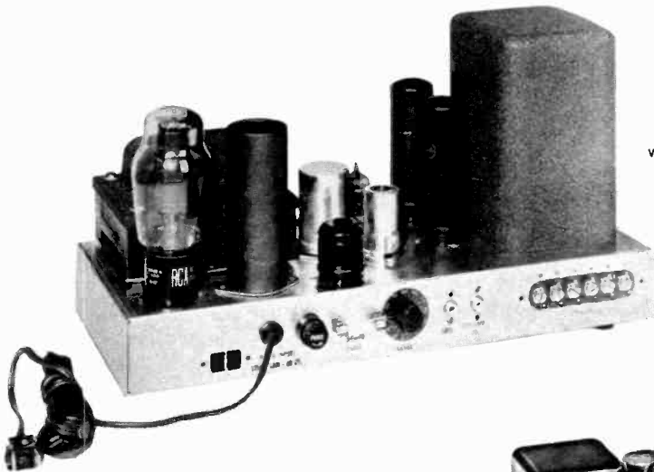
The Grommes 220BA, a 20-watt power amplifier, has a narrow chassis for easy installation. Cost is only $58, performance fine within stated limits
