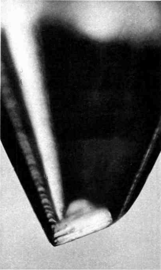
Sapphire stylus after 50 hours has lost its rounded tip and developed first tooth of its cutting edge. It will now damage records
