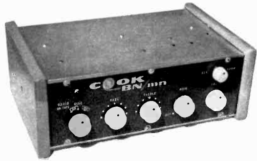
Cook binaural preamplifier requires two separate power amplifiers. It will also work—though very inflexibly—on ordinary monaural recordings
