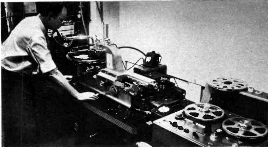
Another engineer supervises the cutting of a master record. Electrical impulses from the tape, when amplified, drive a chisel-shaped cutting stylus into the surface of a disc
