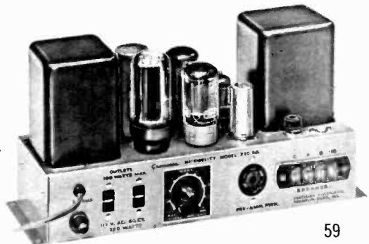
The Grommes 220BA, a 20-watt power amplifier, has a narrow chassis for easy installation. Cost is only $58, performance fine within stated limits
