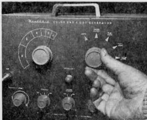
Fig. 11. Color generator is tuned to frequency of an empty channel and set to generate dots.
