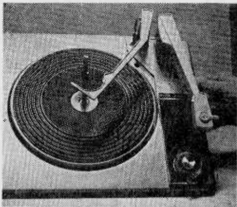
Fig. 19. Using a changer in "manual," be careful not to drop arm as record, stylus, and cartridge may be damaged.
