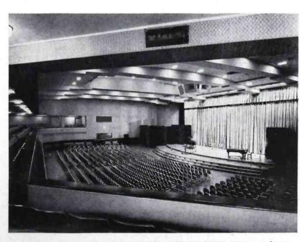
AUDITORIUM STUDIO (8 H) SHOWING RETRACTABLE STAGE AT RIGHT, UPPER AND LOWER CONTROL BOOTH IN LEFT CENTER, AND SPECTATORS' GALLERY AT EXTREME LEFT. WHEN THE SIZE OF THE PRESENTATIONS WILL PERMIT, SPECTATORS ARE ALSO SEATED IN THE PARQUET. OVERHEAD MAY BE SEEN THE SOUND RE-ENFORCING LOUDSPEAKERS WHICH PERMIT THE AUDIENCE TO HEAR THE SAME PROGRAM BALANCE (MIXTURE) AS THAT BEING PUT ON THE AIR
