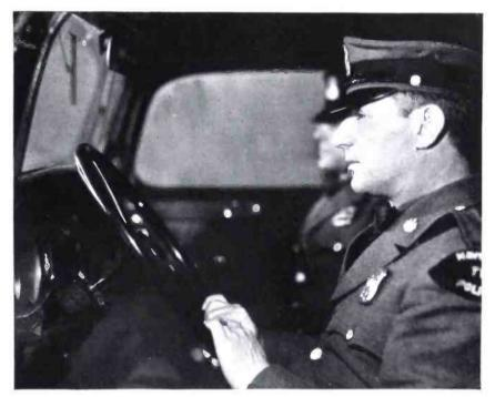
RCA VICTOR TERRA.WAVE POLICE RADIO INSTALLATION IN PATROL CAR OF THE HAVERFORD, PA., FORCE. CONTROLS ARE ON THE STEERING COLUMN
