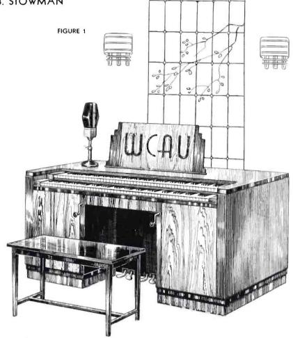
ty of the sound for each keyboard, in place of stops. The conventional bass organ pedals are omitted to alleviate bulkiness, and such notes are included in the full scale keyboards, so that a pianist, as well as an organist, can play the instrument without further training.
