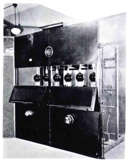
SIX TYPE UV-857 MERCURY VAPOR TUBES IN A TYPE 50.8 50 KW TRANSMITTER
