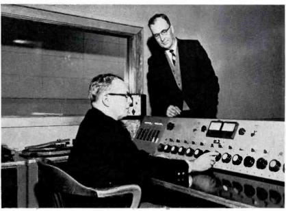
FIG. 16. WAVE-TV Chief Engineer Wilbur Hudson (standing) at audio console with Louis Lau, personnel supervisor. This dual console is one of a long list of equipments designed and constructed by the WAVE engineering department. Panel at left makes possible switching any one of six microphones to the input of each BA-21A program. The output of the mixers feed into BA-23A program amplifiers.
