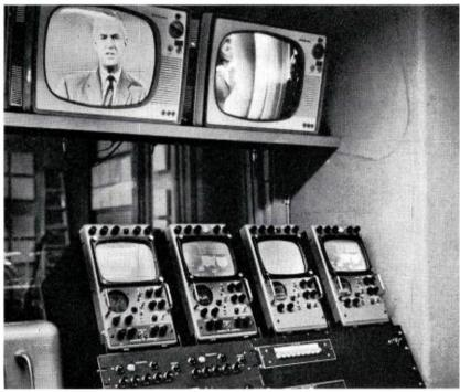
FIG. 7. Video control center, showing four TM-35 master monitors, controls for film system, and switcher-lader.
