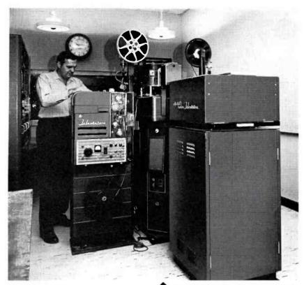
ing two outputs of the 12 by 6 relay switcher appear here. Also in the equipment area are the 6 black and white camera controls.
