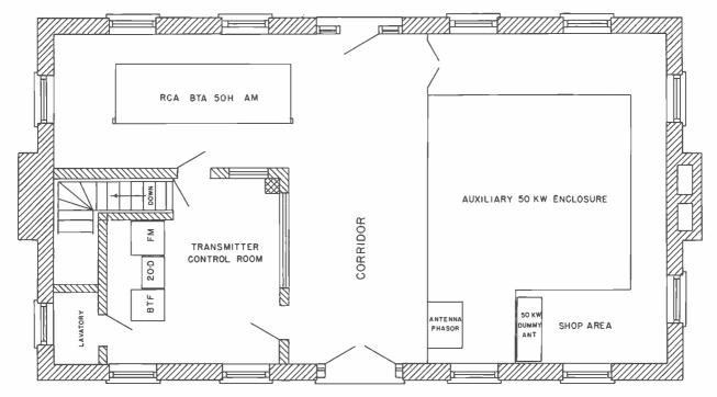
FIG. 5. WRVA-Radio transmitter building floor plan.
