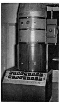
FIG. 13. One of the two r-1 power amplifiers located to the rear of the driver of the transmitter (see FIG. 10). Primary-power switching devices on rear wall.
