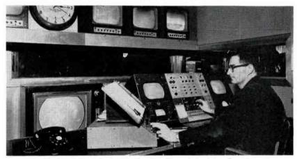
FIG. 22. WAVE-TV control booth, Robert Russell at video switcher. Panel between two TM-6 monitors contains controls for film and slide projectors. Other controls include genlock, network level, stab-amp, and video switcher outputs. Camera monitors are on overhead shelf. Narrow window allows vision into both studios 1 and 2 for director.
