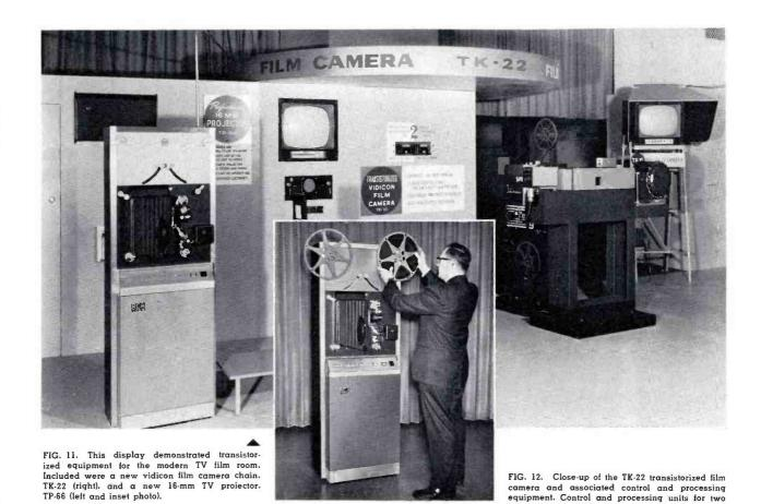
high level, the new camera is equipped with automatic sensitivity control to assure consistent quality in TV picture output in spite of variations in film density.
