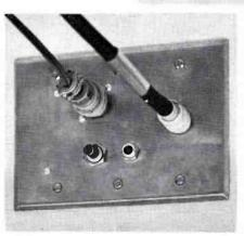
FIG. 12. Instructor's studio talk-back console, With this instrument the TV instructor can enable any viewing student to be in direct communication with the TV center.
