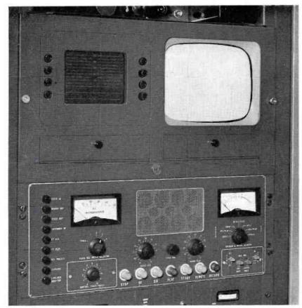
FIG. 8. An 8-inch picture monitor and 5-inch waveform monitor may be mounted immediately above the main control panel. These monitors are especially designed for tv tape recording applications—switching circuits for the monitors are built-in the basic recorder.
