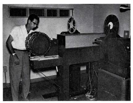
FIG. 8. WTVM film programming starts here. Herman Ragland loads the Type TP-7 Slide Projector which works into the TP-11 Film Multiplexer. The two 16-mm projectors are TP-18 units. The pickup is via RCA vidicon camera.
