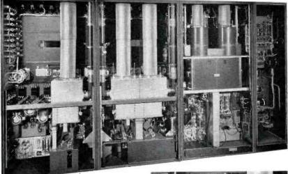
have to be replaced. This feature helps reduce operating costs and also reduces the possibility of lost air time. High-voltage transformer failures have resulted from mercury-vapor tube faults. This type of transformer failure is eliminated by the use of silicon diodes.
