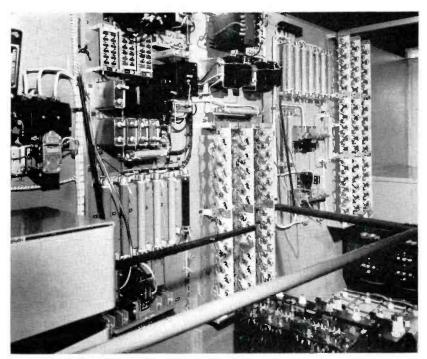
FIG. 4. The interior of the rear panel of the TT-25DH transmitter. Power components located on the floor; silicon rectifiers and other smaller components occupy the panel in full view.
