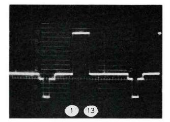
Thus, overshoots do not normally leave the control room. Since there is no energy in the edges of the window signal above 4.0 mc, any appreciable ringing occurring at the top left corner means there is in-band trouble and should be reported.
