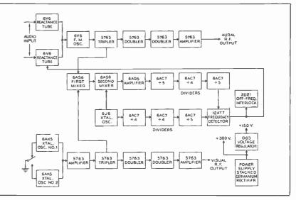
FIG. 7. Block diagram of the visual finals in the TT-25DH transmitter. Diplexing improves the reliability of the transmitter.
