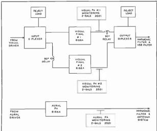
FIG. 12. Block diagram of the power-amplifier portion of the transmitter. Diplexed amplifiers increase transmitter reliability and betters overall transmitter performance.
