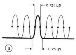
Although a sine-squared pulse could be produced this way, it is not practical from a design standpoint. Actually, it is produced by using a very narrow pulse which is widened and shaped by filters. Thus, one pulse and three sets of filters provide the  $\frac{1}{4}$ ,  $\frac{1}{8}$ ,  $\frac{1}{16}$  microsecond pulses.
