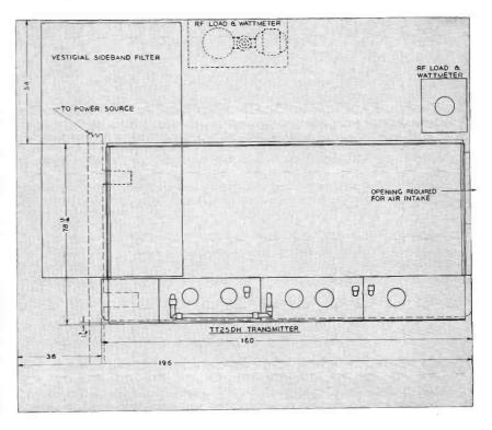
completely contained in one enclosure. There are no external transformers, blowers, or switchgear. This, of course, reduces the amount of interconnecting wire needed as well as eliminates many feet of wire trenches. Also, the walking space required around external components is eliminated; hence, it is possible to install two TT-25DH transmitters in the same area now occupied by most other 25-kw transmitters.
