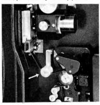
FIG. 6. Automatic lamp-change-mechanism places a new lamp into position within one second of lamp failure.
