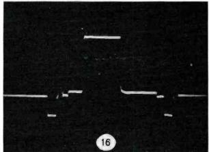
This slide (No. 16) shows the video round robin under average circumstances. The streaking as shown by the rounding of the corners can be more easily seen and photographed if the CRO is set on the IRE roll-off position. Note that the top left corner of the window is almost square but that there is some rounding of the bottom right corner. This is considered to be the present state of the art.
