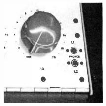
FIG. 13. Pair of phone jacks permit stereo monitoring of two outgoing lines.
