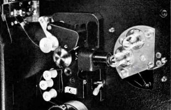
This is a solenoid operated device, which upon sensing that loop loss has occurred applies a force to the film that causes film slippage to occur at the gate between pulldowns. When sufficient film has been recovered from the top loop to establish optimum lower loop size, a second sensing switch de-energizes the solenoid, and the loop restorer arm is free to return to its normal position. Sufficient compliance has been provided to avoid any possible damage to the film during claw engagement.
