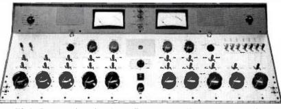
FIG. 3. Front view of consolette showing "human engineered" arrangement of controls.
