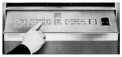
FIG. 10. Illuminated control buttons are arranged for easy identification and operation.
