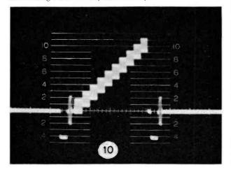
Taking waveform photos of the keyed-in test signals is no problem when using a CRO with a line selector, although it does take a little practice. However, photographing the keyed-in stairstep signal after it has gone through a high pass filter is another matter. One method which works fairly well is to use the sync output from a TA-9 stab amp and drive the CRO externally.
