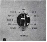
FIG. 12. Monitor phones selector switch.
