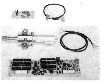
FIG. 5. Functioning elements of TVM-6A off-air monitoring system showing precision calibrated waveguide discriminator cavity (left center) and video component boards. Installation of the transmitter off-air monitor in a TVM-6A transmitter provides fully demodulated and restored signals. The monitor is a separate receiver within the transmitter.
