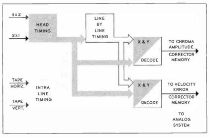
FIG. 12. Block diagram of digital switching system.
