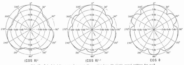
FIG. 10. Calculated three-panel array pattern using  $(\cos \theta)^p$  single panel pattern for a=8.
