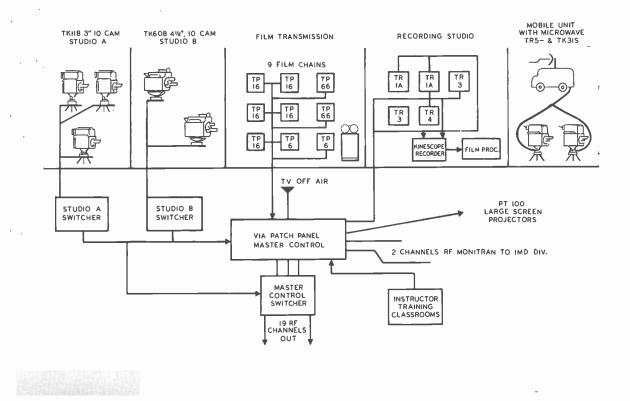
FIG. 27. Block diagram of WFM-TV technical facilities.
