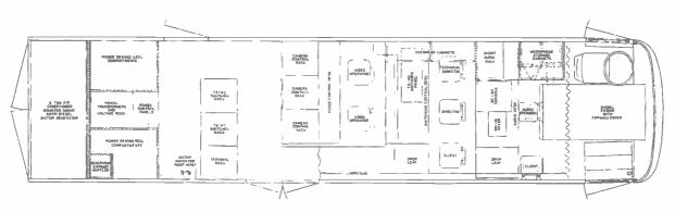
FLOOR PLAN . . . of WHDH-TV mobile bus now being built. Equipment for four TK-43 color cameras will be installed after the current baseball season.
