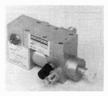
Two additional optional modules that may be used are the low power/low signal indicator that provides an indication of low received RF signal. The other is the video presence indicator, this unit senses the video signal at the receiver control nest.
