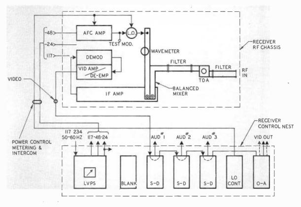
FIG. 10. TVM-6A receiver block diagram showing components in the RF chassis and control units.
