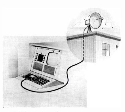
FIG. 3. TVM-6A control unit mounted in studio or transmitter console position providing flexibility for operator. Waveform and video monitors are provided in standard RCA console housing allowing utilization of TVM-6A off-air monitoring capability.
