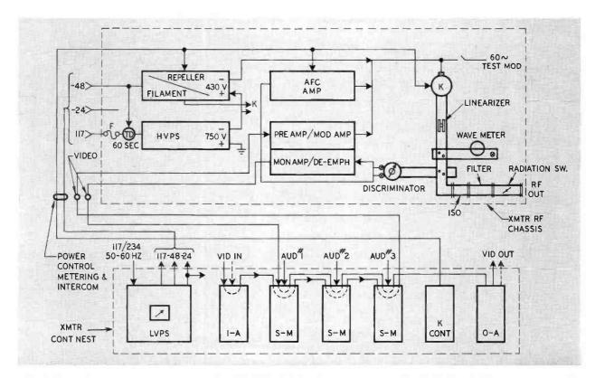
FIG. 7. Transmitter block diagram showing outline of both the RF chassis and the control units. Monitoring of all key program levels is provided by panel meter mounted on the LVPS. Control nest provides space for optional sound modulators or other accessories. Interconnecting cables between both units carry all power, control, metering and intercom circuits.
