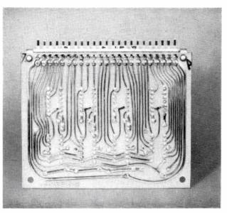
FIG. 7. Wiring interconnections on rear of circuit board.
