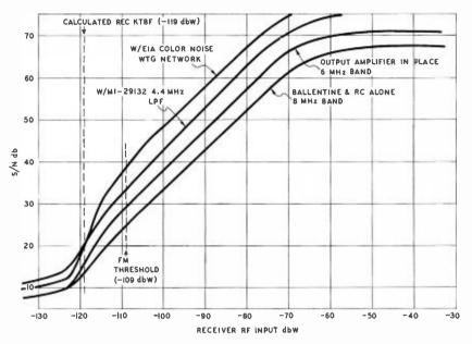
FIG. 12. Typical TVM-6A receiver signal-to-noise performance. Video S/N is in terms of peakto-peak signal to RMS noise. Receiver RF input is in terms of decibels below one Watt. This plot is highly useful in determining proper antenna alignment and for making periodic measurements of receiver sensitivity.
