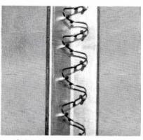
FIG. 8. Zee Panel bent into V-shape.
