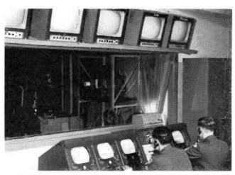
FIG. 23. Video engineers at control console observe pictures on camera controls and overhead monitors, perform switching.
