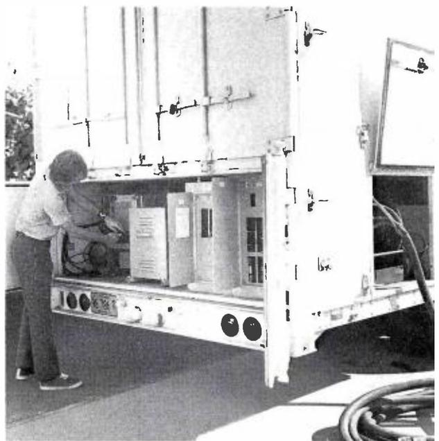
Mounted at the rear of the trailer, behind the video compartment is the power control equipment, including the power input panel; transformers and voltage regulators.
