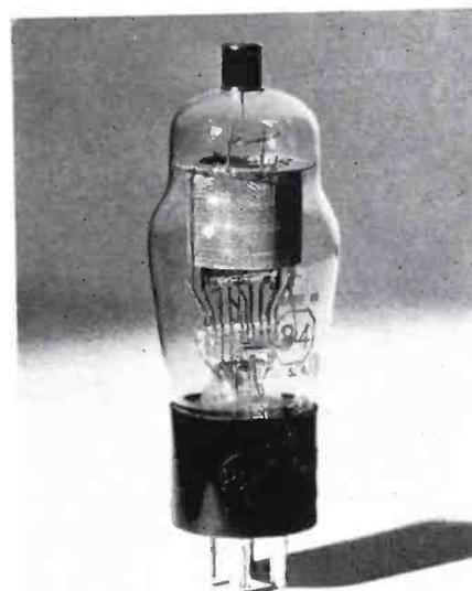
Figure 5. The shield grid tube.
