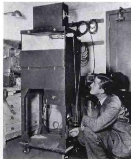
**Showers or deluges are readily supplied with this specially designed mechanism.**
