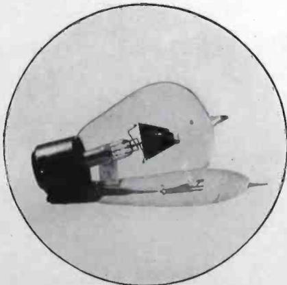
Guthrie found that at red heat an insulated iron ball would retain a charge of negative, but not positive electricity. This discovery brought about the Elster and Geitel experiments with an incandescent lamp having a filament and a plate, in 1880, three or four years before "Edison's Effect," which the latter made no attempt to explain at the time. That Elster and Geitel knew what it was about, is shown by their pointing out the valve effect of this combination in 1889.
