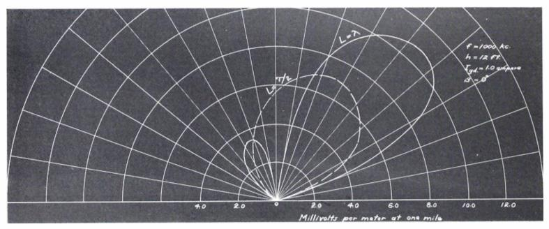
foot, for a number of transmission line heights, with  $I_{qd}$  equal to one ampere. We see that as the transmission line is placed closer to the earth, the current density increases directly below the line, but drops off quicker in a lateral direction.
