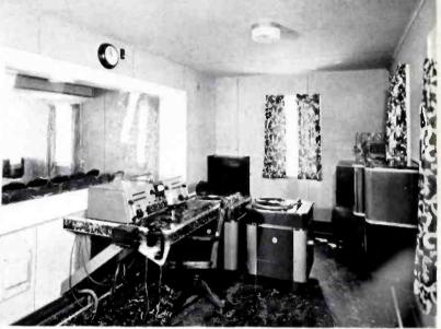
RCA 76 B Consolette, 70-C Turntables and 64-B Loudspeaker are combined to provide an efficient speech input system.
