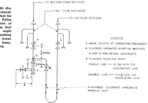
connected at junction "F" during foursection operation thus causes negligible change of input impedance and power loss. The input impedance to the antenna system is thereby maintained at very nearly 51.5 + jo ohms during four- or eight-
