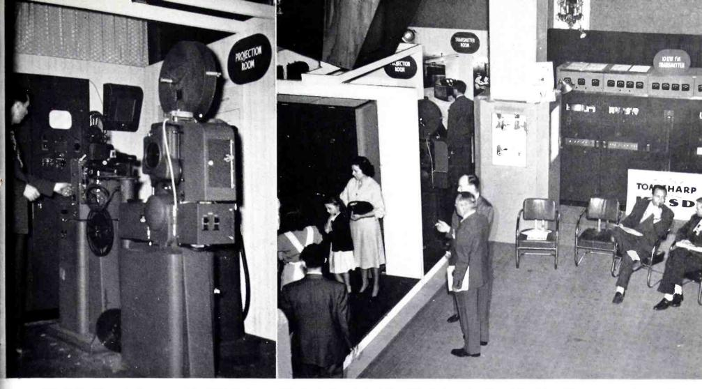
FIG. 6. The film projection room of the NAB display. In the foreground are 16mm and 35mm projectors. A multiplexer unit, between the projectors, allows the picture from either to be projected into the film camera (behind the 35mm projector in this view).
