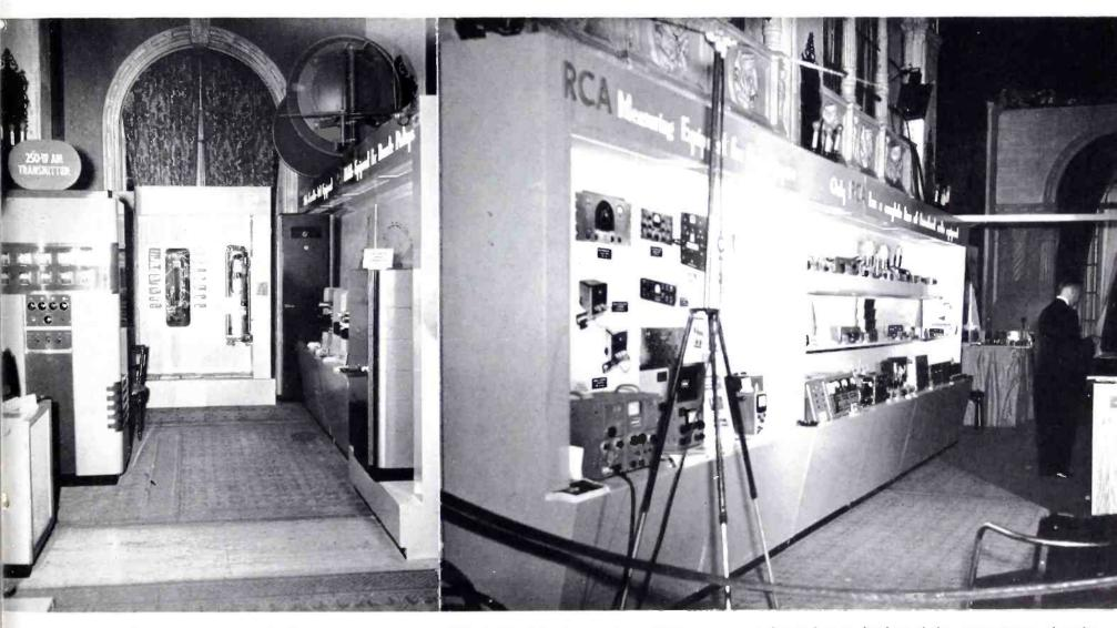
FIG. 8. Special transmitter displays occupied this wing of the exhibit space. Display in center illustrates operation of grounded-grid tank circuits used in RCA FM transmitters.
