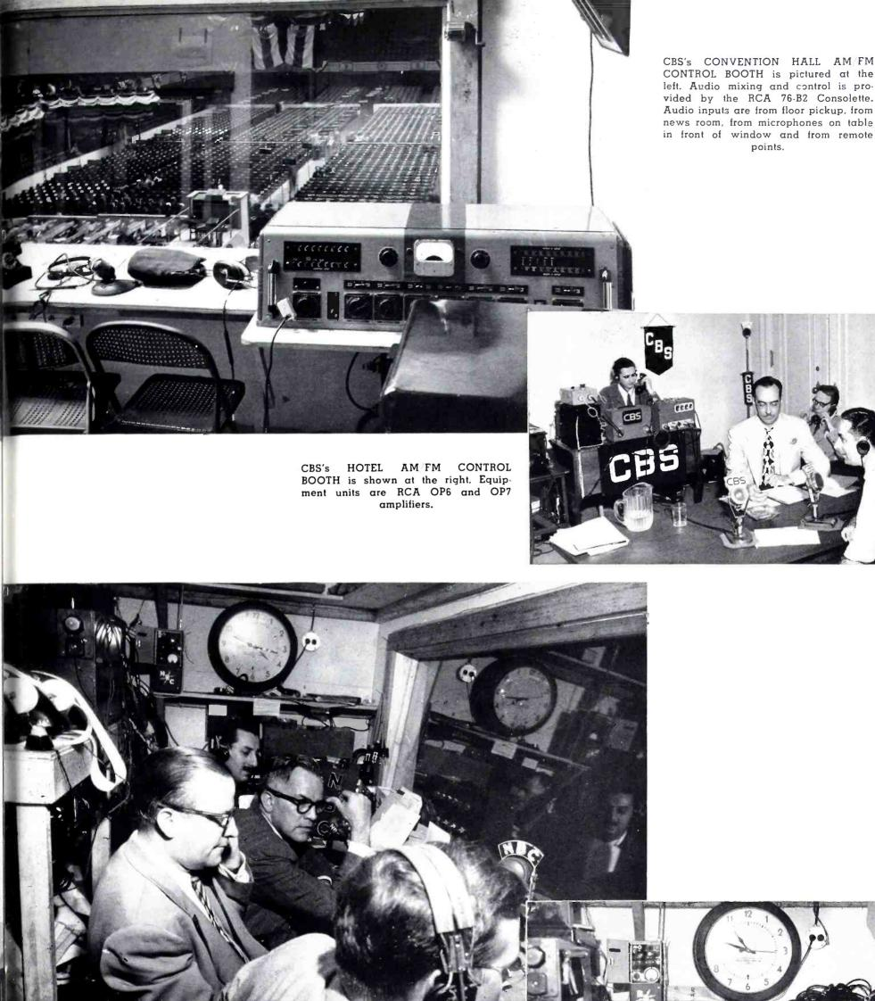
NBC's CONVENTION HALL AM/FM CONTROL BOOTH is shown above during actual operation. Announcers, analysts and news commentators sat along table in front of the window that looked out on the Convention Hall floor. Engineers position, at the far end in the view above, is shown closeup in the small illustration at the right. Portable equipment used by NBC are similar in general design to RCA OP.5A amplifier used by many stations.
