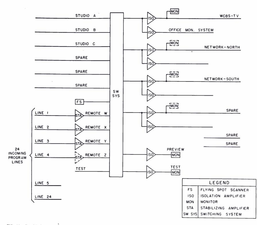
FIG. 11. Simplified block diagram of the video master switching arrangement. Provision of additional units is indicated by broken lines.
