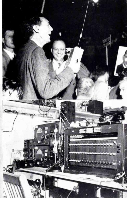
RECEIVING POSITION in NBC control room is shown here. Two communication type receivers were used to pick up 27 mc transmissions from the radio mikes on the Convention Hall floor,
