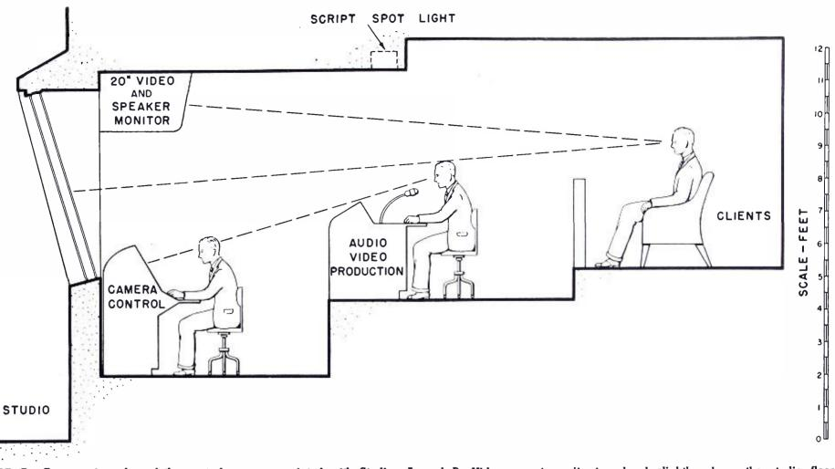
FIG. 7. Cross-section plan of the control rooms associated with Studios A and B. Video operators sit at a level slightly above the studio floor. Production director, switcher, and audio engineer on a second level, and clients at a third level. Broken lines indicate site lines.
