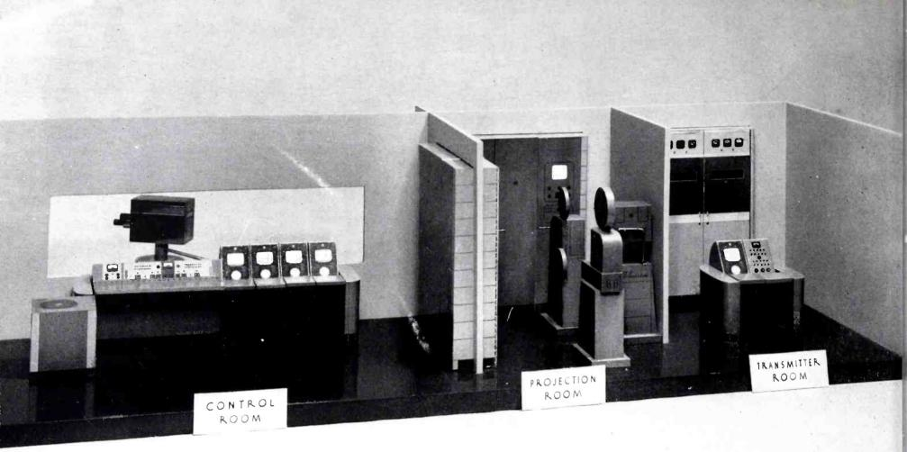
FIG. 1. This is a scale model of the "complete television station" displayed at the NAB Convention. Room at the left is a typical studio control room, room in the center is the film projection room and the room at the right, the transmitter room.
