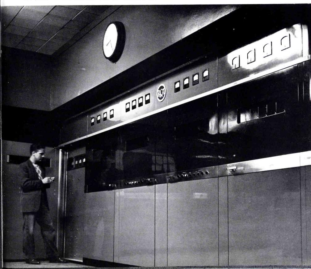
equipment. A complete custom-built recorder has been installed in the recording control room which has two type 73-B recorders mounted either side of a special switching turret that has incorporated in it switching facilities to permit the use of any of six incoming lines on either recorder or both at the same time. Either of the program busses on the cutting unit may be monitored during operation.
