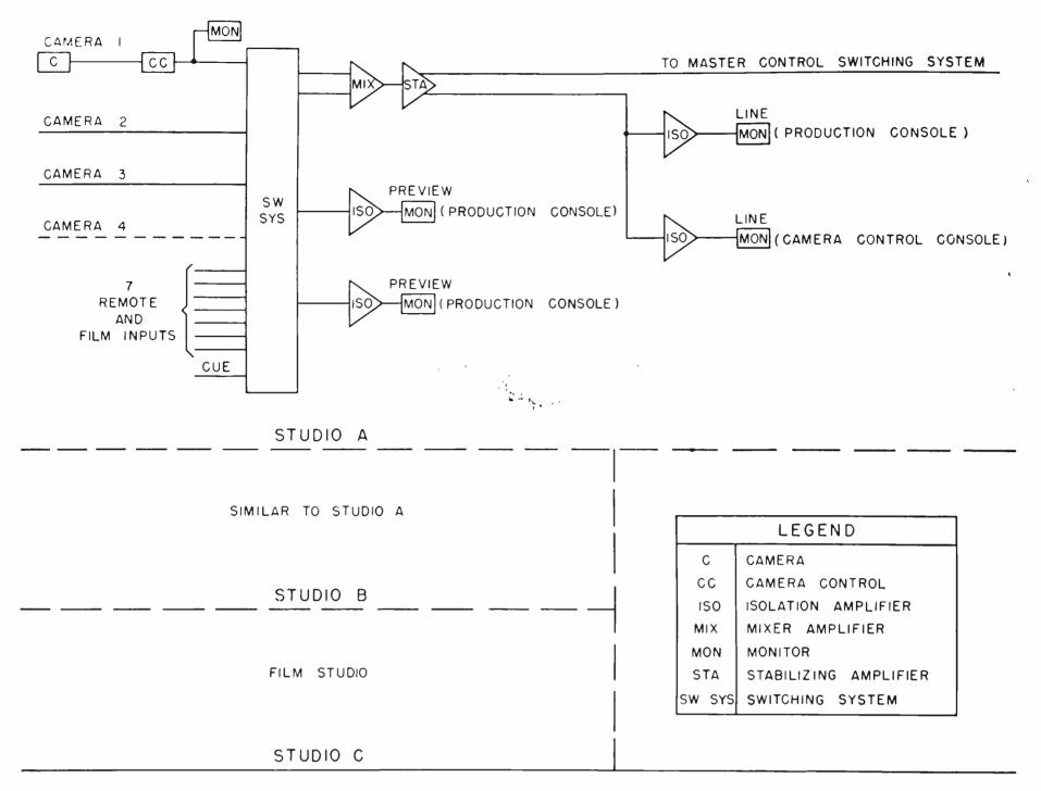
FIG. 8. Simplified block diagram of the video facilities for Studio A. Video units for Studios B and C are similar.
