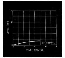
FIG. 6a. (Above) Continuous Application of Sine-Wave Signal Causes Some Increase in Recording Level at 1000-Cycles.
