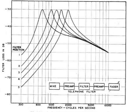
FIG. 6 (above). Typical telephone filter characteristics.
