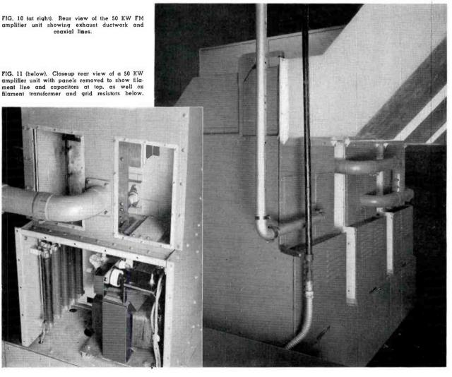
loaded three-quarter wave line, shorted at the input, is used for the filament circuit. This line is formed by the power-frequency filament buses which are folded over and pass down at the back of the plate line.
