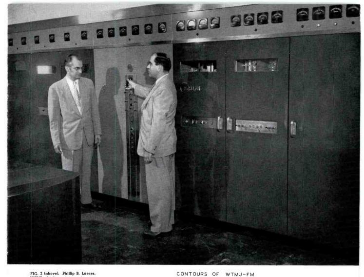
FIG. 2 (above). Phillip B. Laeser, WTMJ chief engineer, observes as W. B. Fletcher, RCA engineer, demonstrates ease of power cutback to 10 KW from 50 KW operation. All units of the RCA 50 KW FM transmitter are mounted behind a unified front panel providing a neat business-like arrangement with complete accessibility.
