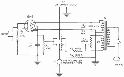
FIG. 14 (above). Schematic diagram for α diode rectifier for measuring AM hum and noise. Note that this equipment will give direct readings when used with any noise meter.
