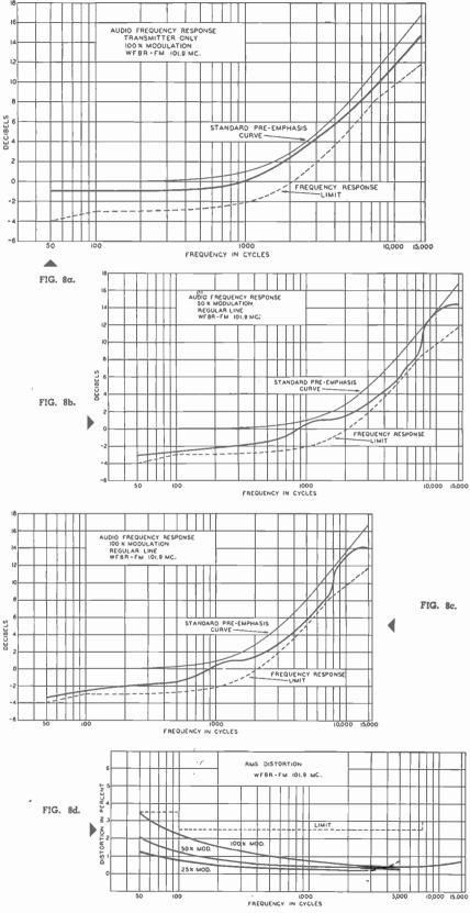
These input readings when subtracted from a suitable reference level should be compared with the standard pre-emphasis curve. To be within the FCC limits it should be possible to plot a curve from this data which, when referred to a suitable reference level, will fall between the standard curve and the lower limit curve shown in Fig. 8a.
