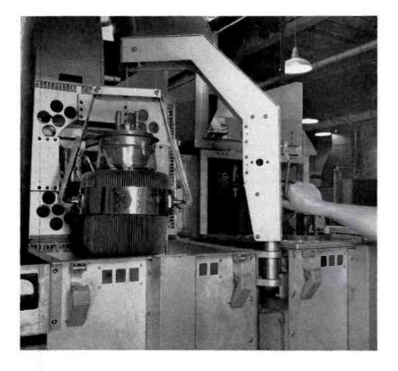
these amplifiers is unusual in that the outer conductor of the concentric plate line tank is square and forms the skeleton of the unit.
