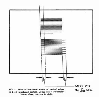
also increase to accommodate the greater resolution required in the horizontal direction. The present system employs 525 lines, a number arrived at after thorough consideration of the related questions of channel width and resolution by the N.T.S.C. and the R.T.P.B.
