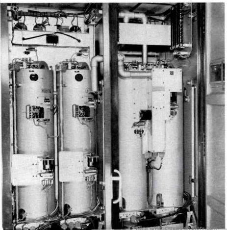
trol wiring was kept out of the r-f fields, and radar type plumbing was used in the r-f circuit.
