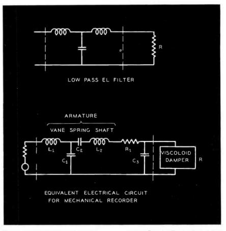
FIG. 2b. Equivalent Electrical Network for a Mechanical Becorder.
