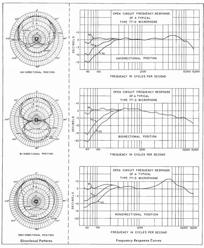
FIG. 5 (above). Directional patterns and frequency response curves for the RCA Type 77-D microphone.
