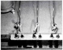
FIG. 5 (above). Closeup showing the output connections of phasing unit. Note linos run in duplicate and method of selection.
