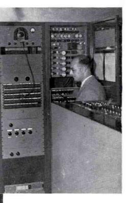
FIG. 10. Projection room facilities include two sets of 16mm projectors and two film cameras. One film camera is just visible in the photo. The projection monitor (upper 1eft) is a converted RCA TV receiver.
