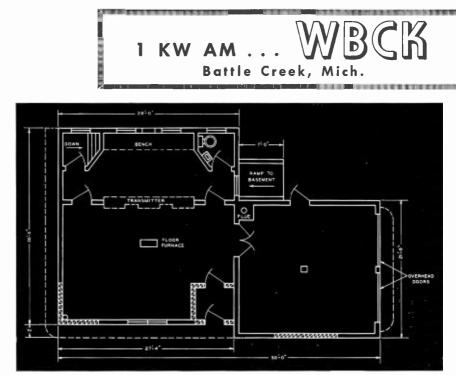
FIG. 2 (above). The floor plan illustrates how the BTA-IL is flush-mounted in one wall, with access doors provided at each side of transmitter.
