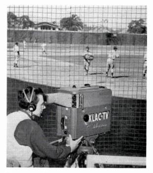
KLAC-TV's No. 1 Camera position is shown above. Here again the location is very low—only 5 feet off the ground. This has the disadvantage that players occasionally walk in front of it—but it gives an unusually dramatic picture of pitcher's delivery. It is even claimed that you can see the ball break on a curve. KLAC-TV's No. 2 Camera is higher—in the first tier at Hollywood, and in the second tier at Los Angeles. This is used for outfield shots.
