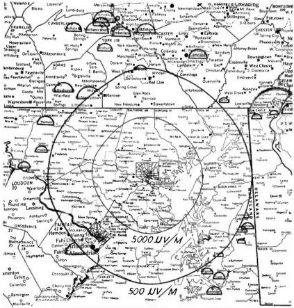
FIG. 17. 5.000 and 500 microvol/meter contour lines of WBAL-TV. Small semicircles indicate towns outside the 500 microvol/meter area reporting good reception.
