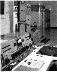
FIG. 3. The control console and transmitter are so placed that the operator can easily monitor all the equipment.
