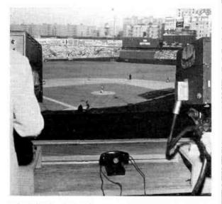
WABD's No. 2 and No. 3 Cameras are 40 feet high just a little to right of pitcher-batter line. Locating all three cameras at same horizontal helps orientation on fast camera switches.
