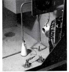
FIG. 6 (above). A coupling unit termination of transmission lines showing method of selecting the line desired.
