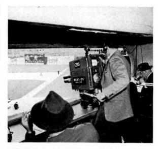
WCBS-TV's No. 1 and No. 2 Cameras are ideally located in booth directly behind homeplate. Position is low enough for good "cover" shot with relatively small-size lens.
