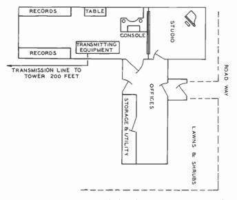
FIG. 2. Photo above shows a simple floor plan of Station KXLL. As can be seen in the plan, the operator at the control position has a good view of the studio and other office facilities.
