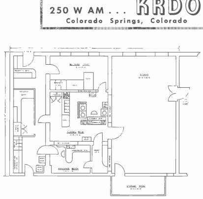
FIG. 4. The floor plan (above) shows the layout of station KRDO including the studios and transmitter located on the ground floor of the Alta Vista Hotel.
