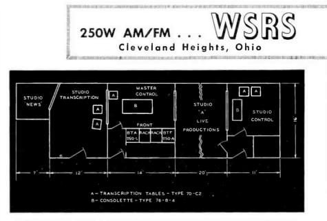
FIG. 5 (above). The WSRS single-floor station plan showing transmitter room and studio layout.
