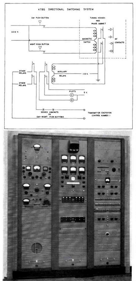
FIG. 12 (left). Simplified schematic of the KTBS directional switching system. Push buttons on the phasing cabinet operate contactors in the phasing cabinet and in the six antenna tuning houses. Back contacts operate signal lights in the transmitter room and prevent excitation from being applied until all contactors have closed.
