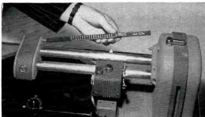
**CALIBRATED TIME SCALES** for 96, 104, 112, 120, 128, 136, 144 and 152 ("inside-out", "outside-in", at 33 $\frac{1}{3}$  or 78 RPM are provided. Here, proper scale to agree with "pitch" setting is inserted. When the fine groove kit MI-11882 is used the time scales are doubled.
