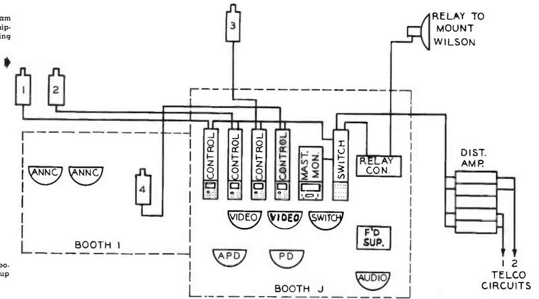
FIG. 12. Microphone positions and audio setup used at KECA-TV.
