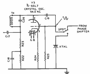
FIG. 6 (at right). All RCA sync generators at WPIX are modified so that the phase shifter can be substituted for the crystal.
