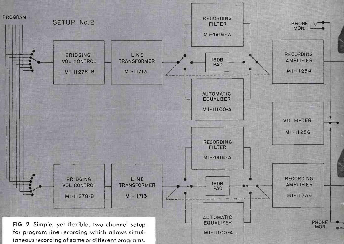
FIG. 2 Simple, yet flexible, two channel setup for program line recording which allows simultaneous recording of same or different programs.
