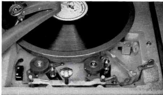
**OFF**—In the "OFF" position a brake shoe is applied to the turntable rim, and rubber idlers are moved away from both the drive wheel and turntable rim.
