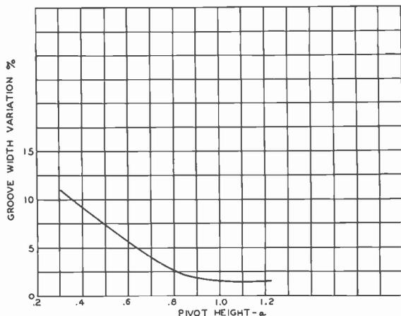
FIG. 13. Curve showing Groove Width Variation with Pivot Height.
