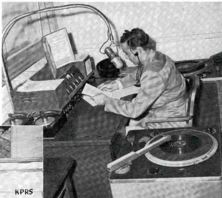
FIG. 4 (above). In the KPRS Studio Control Room are located two RCA 70-D Turntables, console and two 9Y RCA "45" record players.
