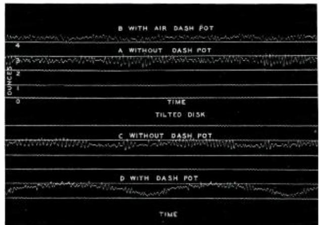
FIG. 10. Oscillograms showing cutter bounce and the improvement obtained with an air dash-pot.
