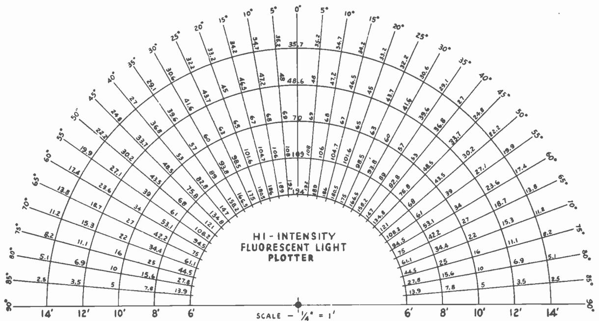
FIG. 2 (above). This light plotter can be used for checking the light output provided by fluorescents.
