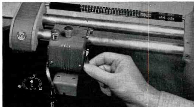
**RAISING AND LOWERING** the cutter head is easily done by this lever which permits raising the "to rest" position or a gentle lowering to the recording position. The "Flat" cutter and the mounting position minimize cutter bounce.
