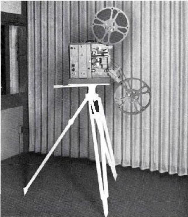
The new TP-10A Portable Projector (MI-26963) is intended for use in the production of remote television programs, or as an auxiliary to the film studio facilities. In either case, film commercials or other films of reasonably short duration can be inserted in the program with a minimum of time and facilities. The image orthicon studio or field type camera with a few simple modifications is ideal for use as a film camera when operated with the TP-10A Portable Projector.
