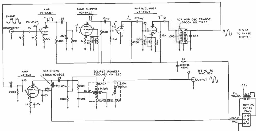
peak to peak video signal with negative sync across 75 ohms. See Fig. 7 for diagram.
