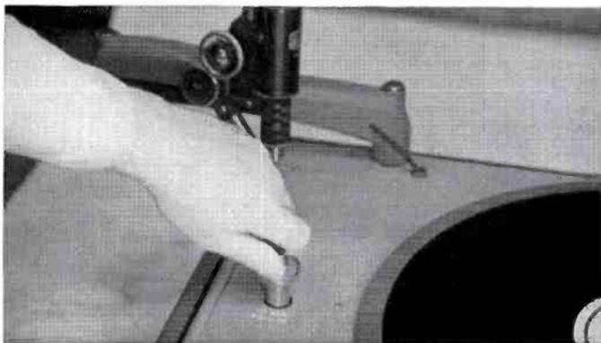
**SPEED-CHANGE** is simply accomplished by operating the control knob shown here. "UP" is  $33\frac{1}{2}$  RPM—"DOWN" is 78 RPM. With MI-11860 drive pulleys 45 RPM can be obtained—"DOWN" and  $33\frac{1}{2}$  RPM "UP". Or MI-11861 will provide 78 RPM—"DOWN" and 45 RPM "UP".
