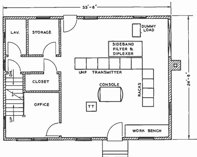
FIG. 2 (above). Floor plan layout of KC2XAK equipment. Though the building is quite small, there is adequate space for storage, office and lavatory facilities. There is also plenty of walk-around space in the transmitter room. The sideband filter and diplexer are actually mounted overhead behind the transmitter.
