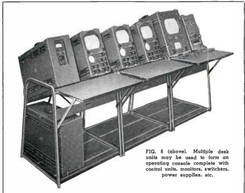
FIG. 8 (above). Multiple desk units may be used to form an operating console complete with control units, monitors, switchers, power supplies, etc.
