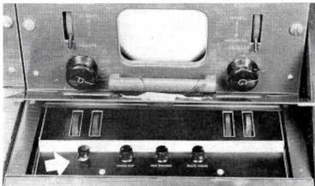
FIG. 3 (above). Hinged cover of Studio Camera Control is raised to show location of new target control key.
