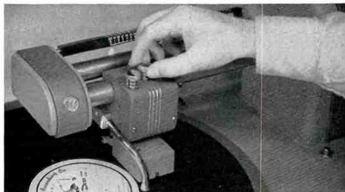
**ANGLE AND DEPTH OF CUT** are conveniently and precisely controlled by the two knobs atop the carriage. (In above, angle of cut is being adjusted.) The angle remains the same but the depth of cut is less for fine groove recording.
