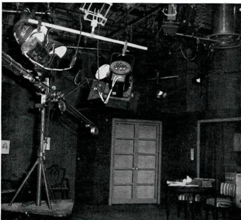
FIG. 15. A lighting arrangement in which frequent scenery changes and camera movements may require rapid manipulation of lights.
