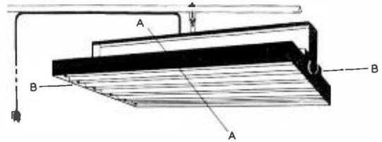
FIG. 8. Typical fluorescent floodlights (equipped with reflectors for four or six lamps) also produce wide, uniform distribution curves.
