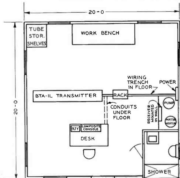
FIG. 2 (above). The transmitter building floor plan layout. A minimum space of approximately 20 feet by 20 feet accommodates the entire transmitter plant facilities.
