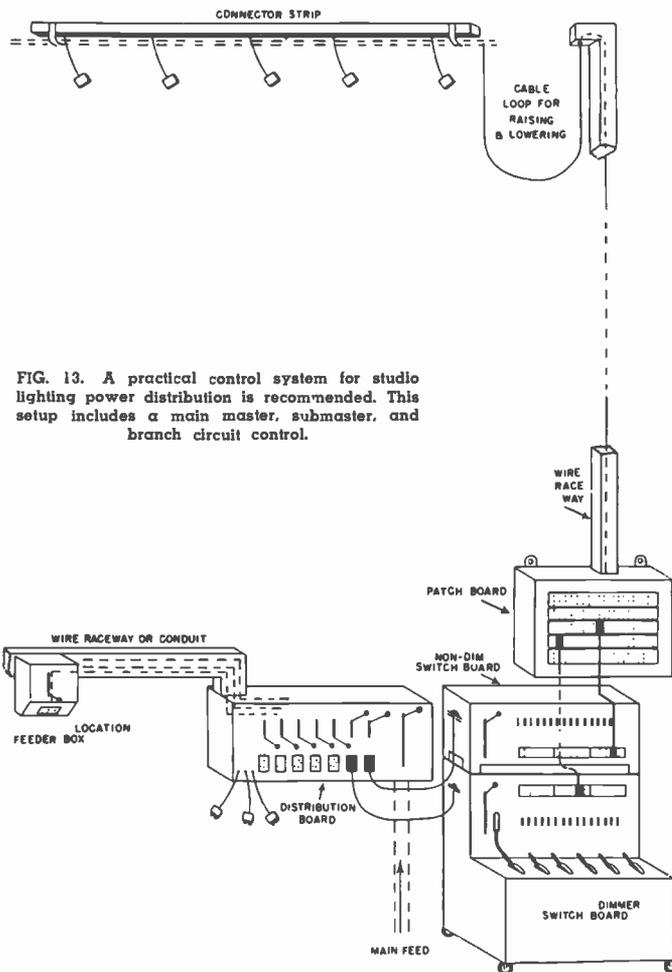
FIG. 13. A practical control system for studio lighting power distribution is recommended. This setup includes a main master, submaster, and branch circuit control.
