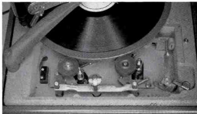
**ON**—In "ON" position, the brake shoe moves away from turntable rim and rim and rubber idlers are now in active contact with drive wheel and turntable rim.
