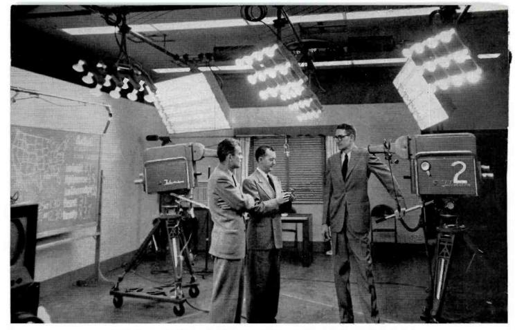
FIG. 1. Assistant Chief Engineer Scott N. Hagenau, center, uses a light meter to check the illumination in the WSBT-TV studio. Looking on are Robert J. Drain, Program Director, left, and Arthur R. O'Neil, right, Chief Engineer, Lighting is provided by banks of incandescent spot lights and high intensity fluorescent tubes.
