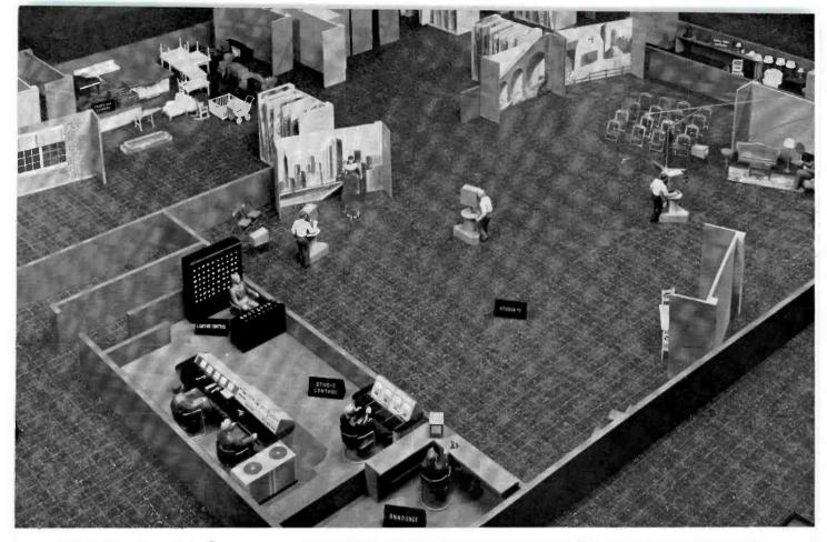
FIG. 52. View of large Studio #1, companion control room and the nearby "prop and scenery" storage area. Note that, in this setup which uses the TC-5A Program Director's Console, the video monitors have been located away from the control room window. The program director and audio operator are at a second level, with the lighting control operator and his equipment plus the video monitors at a lower level. (Actualy these camera controls could be located in a different room.)
