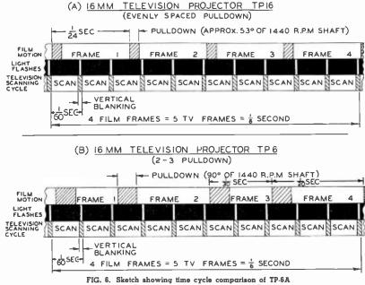
FIG. 6. Sketch showing time cycle comparison of IP-6A Professional Projector with that of the TP-16 Projector.
