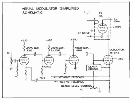
FIG. 7. Visual modulator simplified schematic.
