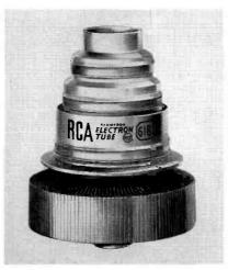
FIG. 12. 6181 tube used in both aural and visual outputs.
