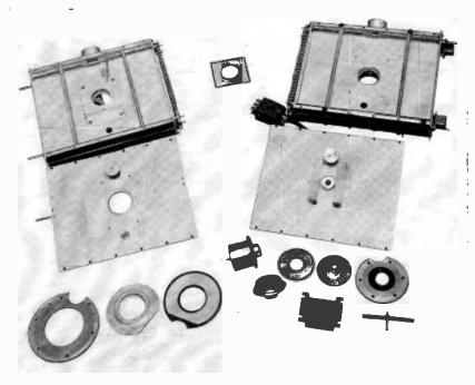
FIG. 9. Rectangular cavity for 6161 disassembled.
