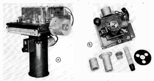
FIG. 10. Photo "A" (left) shows completely assembled PA cavity. Photo "B" (right) shows bottom view, partially disassembled.
