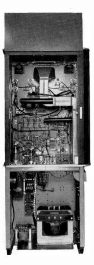
FIG. 3. Rear view of the visual transmitter shows the simplicity of construction and the ready accessibility of all components.
