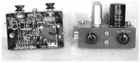
FIG. 12. Under-chassis view and front view of preamplifier chassis.
