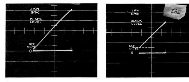
FIG. 13A (left) and FIG. 13B (right). Curves showing linearity of TTU-1B.
