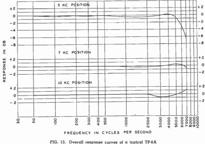
Projector using "SMPTE" multifrequency test film.
