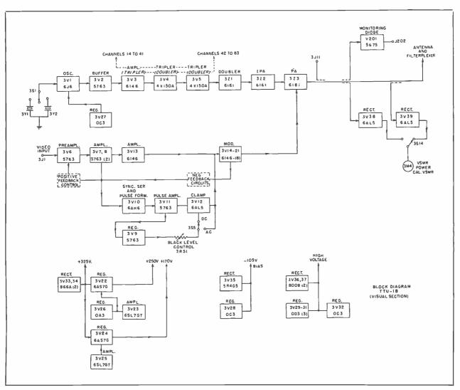
FIG. 5. Block diagram of TTU-1B visual transmitter.
