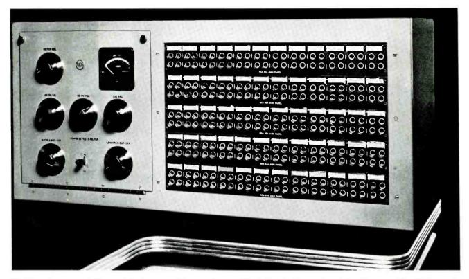
FIG. 6 (opposite page, top). Closeup of the front turret. Mixer controls are mounted on lower part of panel which is sloped at an angle of sixty degrees (from vertical) to provide maximum comfort for operator. VU meters, switches, masters and monitoring controls are on upper part of panel which is at fifteen degree angle for best observation of meters.
