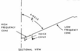
FIG. 2. The angle  $\phi_1$  into which the high-frequency cone feeds without the "domes" is relatively wide.
