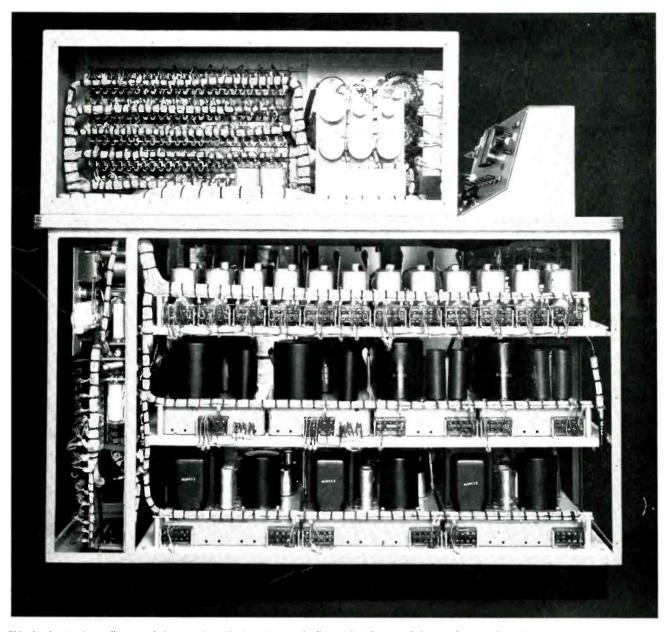
FIG. 5. A side (or end) view of the console with the side panels (lastened with concealed screws) removed to show arrangment of components in the pedestal and the side turret. The amplifiers (front view in Fig. 2) are all of the plug-in type so that they may be removed easily for servicing or replacement. The fact that all inter-unit wiring and complete check-out is done in the factory makes for fast, economical installation.
