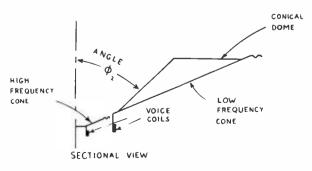
FIG. 3. When the "domes" are added the angle  $_{\Phi^2}$  is much smaller, thereby improving high-frequency efficiency.
