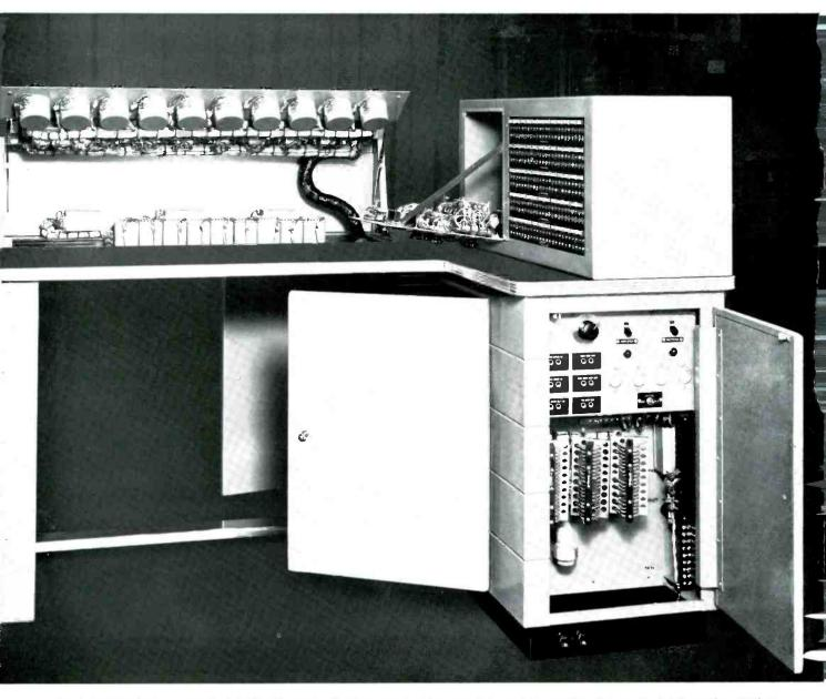
FIG. 4. Accessibility is a feature of the WBAP console. The front panel of the operating turret is hinged at the top so that it can be raised to provide quick access. The control section of the side turret is hinged at the bottom so that it can be lowered as shown in the view above. The amplifier and power control compartments in the pedestal have hinged doors.
