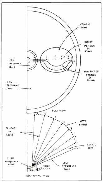
FIG. 4. Some of the sound emitted by the highfrequency cone is diffusely reflected by the "domes", thereby smoothing out response curve.
