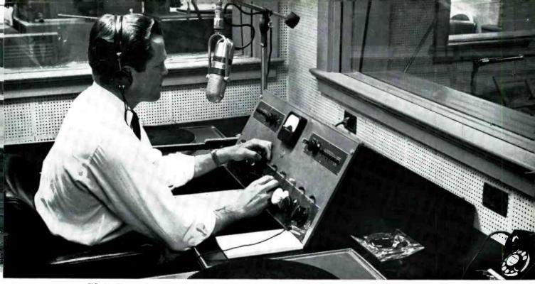
FIG. 8. "B" control room is, in effect, the center of operations, with its BC-2B consolette. Through the window to the right—partially visible—is the small speech studio and Control Room "C". Beyond the announcer is the recording room.
