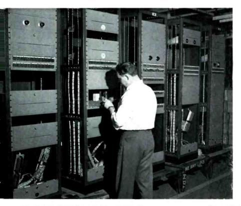
FIG. 8 (below). It is not feasible to take a complete "systems" test at the factory on a project of this size. However, the completed racks are usually "circuit checked" individucIly as shown here.
