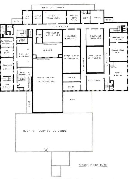
FIG. 7. Second floor plan of the WBAP building. Stairways at each corner of the main building, together with six main building entrances (three in front. and three in the rear) make it possible to enter any of the six sub-areas. from either the front or back of the building, without walking through any of the other sub-areas. Recently a 68 by 58-foot extension has been added to the left side of the Service Building to provide additional storage area.
