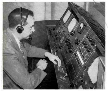
The RCA TS-5A Video Switcher is a flexible two-unit equipment designed to mount in a single standard console housing. The push-button and fader panel may be located as illustrated or in the upper face of the console. The TS-5A is designed for color use as well as for monochrome.
