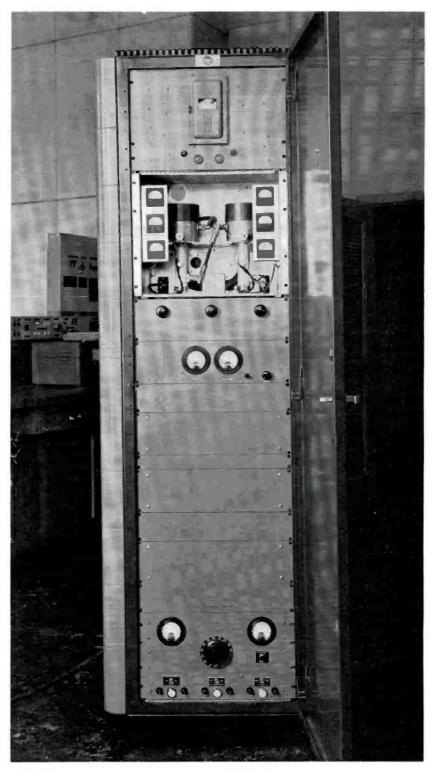
FIG. 10. The complete booster equipment is contained in the BR-84 rack shown above. Power supplies are at the bottom, voltage amplifiers and intermediate amplifiers just above. The final power amplifier uses two 4X150G in coaxial cavities which can be seen in this view.
