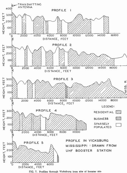
FIG. 7. Profiles through Vicksburg from site of booster station KK2XFI. Location of profiles is shown on map in Fig. 3.
