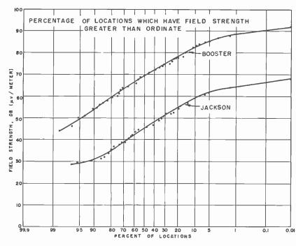
FIG. 5. Statistical analysis of field strengths received in Vicksburg area from booster station KK2XFI and originating station WJTV.
