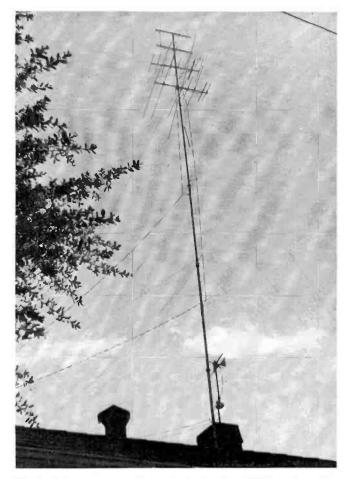
FIG. 2. Antenna array used by dealer in downtown Vicksburg to receive stations in Jackson. Bow-lie UHF antenna just above roof was installed for tests described here. It provided excellent reception of booster station signals.
