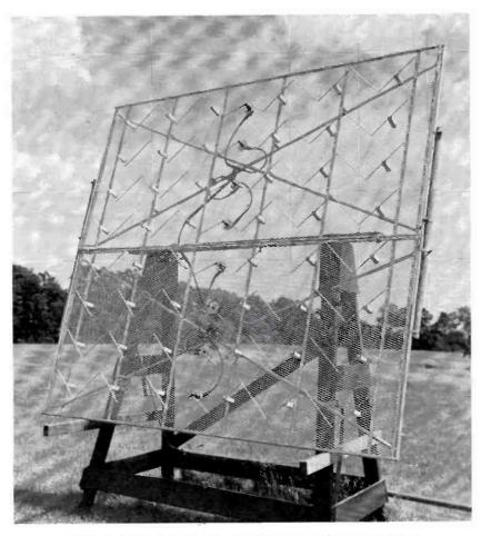
FIG. 12. This is a closeup view of the zig-zag receiving antenna before installation on the water tower shown in Fig. 2. It has a measured beam width of  $16^{\circ}$  (both vertical and horizontal) and a gain of 20.5 db.
