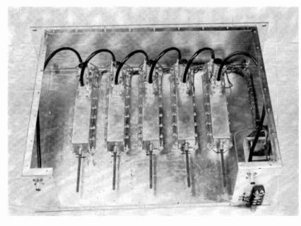
FIG. 9. This five-stage voltage amplifier is used to amplify the received carrier signal to the level necessary to drive the intermediate power amplifiers.
