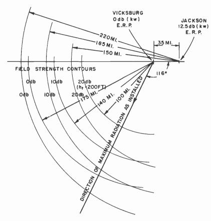
FIG. 8. Calculated field strength contours of booster station KK2XFI and originating station WJTV. Outer contours of KK2XFI lie well within those of WJTV, indicating booster operation will not increase interference to other stations on same channel.
