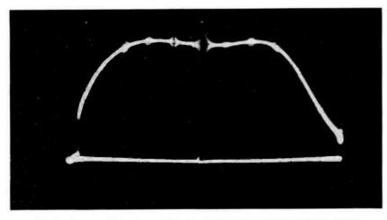
FIG. 11. The overall booster amplifier has a gain of the order of 100 db. and a bandwidth essentially flat over 6 megacycles. A typical response curve is shown above.
