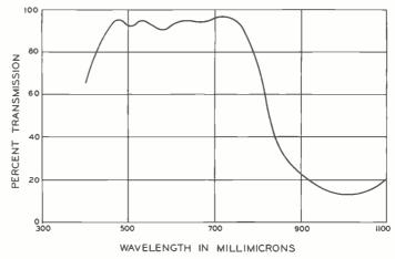
FIG. 4. Spectral transmission curve of Fish-Schurman Type XUR infrared deflector.
