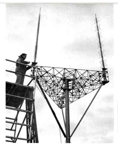
To acquire performance data on antennas mounted side-by-side in reasonably close proximity, working model antennas built to onetenth scale and operating in the region of 500 to 1500 mc. were used. The supporting triangular platform is also a scaled replica of the completed installation.
