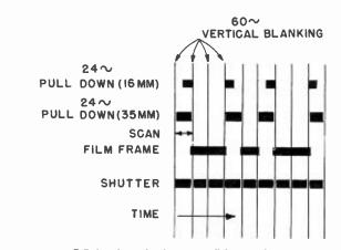
FIG. 2. Relationship between pull-down projectors, shutter, and scanning in prior television practice.
