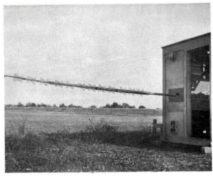
TF-6BM scale model on pattern test set-up.
