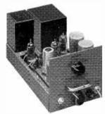
BA-23A PROGRAM AMPLIFIER ... A versatile high-fidelity amplifier using special highquality components and providing maximum accessibility. High gain and low distortion make it without equal as (1) program or line amplifier, (2) bridging amplifier, (3) isolation amplifier. Three BA-23A amplifiers can be mounted on BR-22A shelf with space for an additional amplifier.
