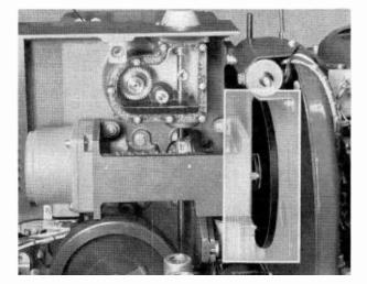
FIG. 8. Light-intensity control mounted in an RCA TP-SCC Projector.
