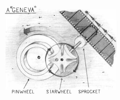
FIG. 4. Simplified diagram of a Geneva mechanism.
