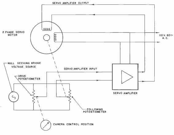
FIG. 3. Bridge circuit which drives the filter wedge.
