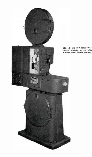
ducing head that is used with theater type projectors is a part of this projector. The complete machine is shown in Fig. 10.
