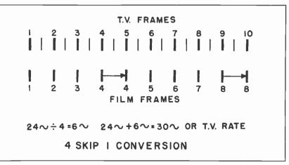
wheel one-half cycle later and advances the film to frame 3. Pin 2 advances the film to frame 4, and is withdrawn. Pin 1, now again extended, advances the film to frame 5 which is the beginning of a new sequence. Four frames of film have served for five frames of television information.
