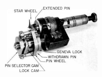
FIG. 6. Overall view of complete intermittent.
