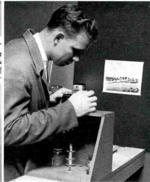
FIG. 24. Hot press . . . prints title cards for slides and opaques from regular printer's type quickly and efficiently.
