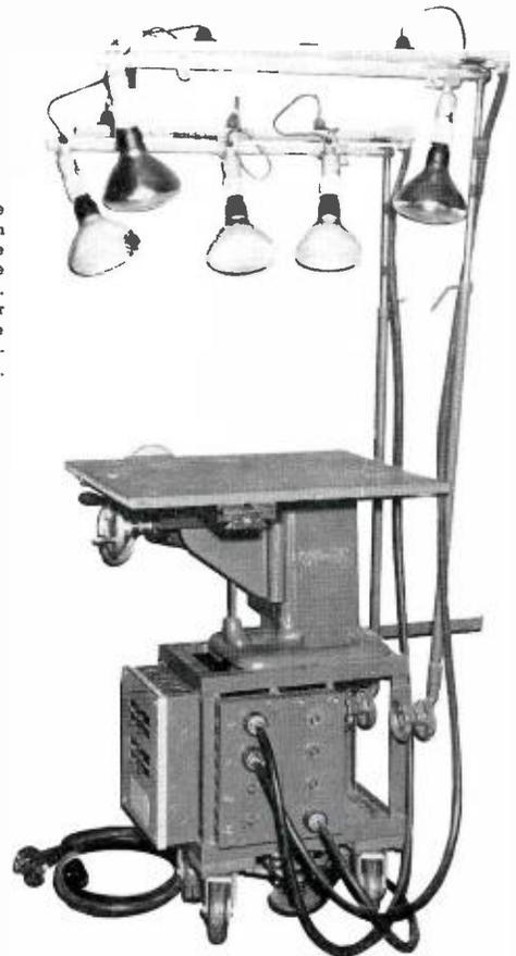
Mounted on the base of the milling machine is a lighting switch panel. This serves to distribute power to the three adjustable lighting booms, the light box, the turntable and two accessory outlets. The lighting booms were constructed from discarded music stands and are adjustable both in elevation and angular position. Plugmould outlets are fastened to the boom, providing ac facilities along the length of the boom. Clamp-on adjustable sockets serve as the spot and flood light holders.
