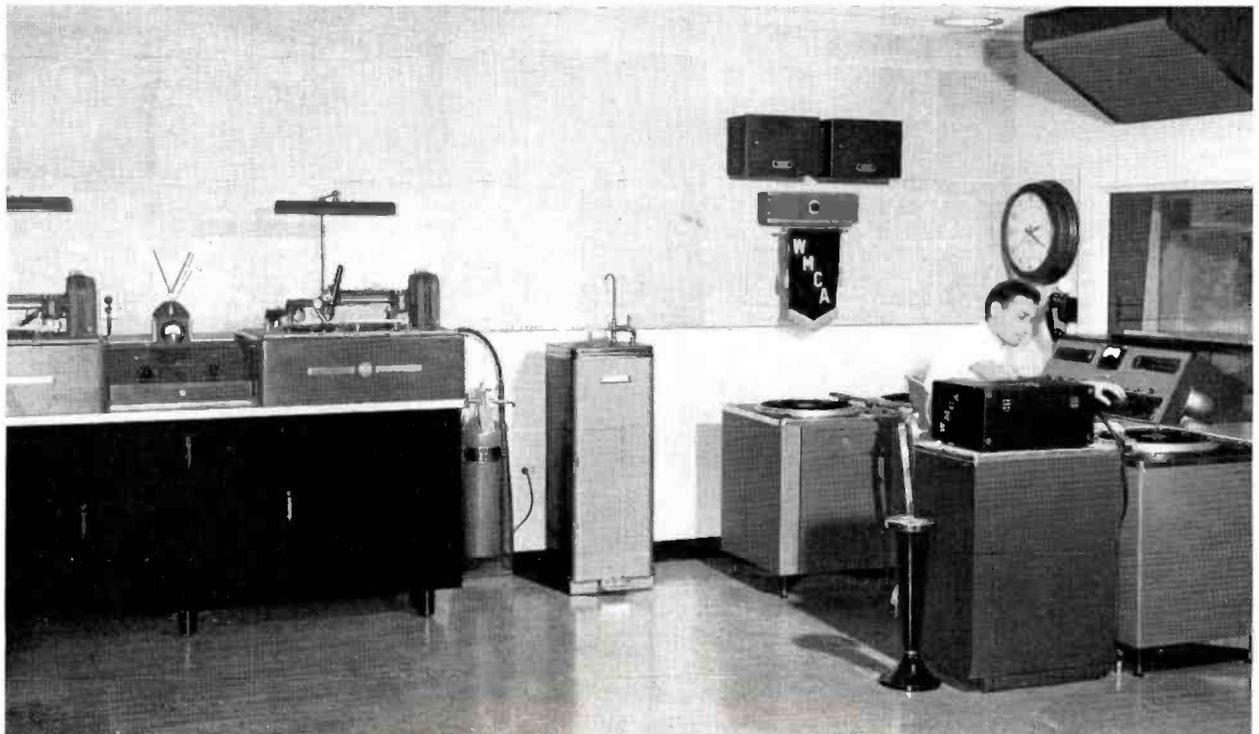
normal appearance of the RCA BC-2B console may notice a number of small holes in a plug (filling a hole normally used for warning or indicator lights) to the left of the VU meter. Behind this plug has been installed the mechanism of an RCA Aerodynamic microphone. The microphone is thus out of the way of the operator but is readily available to him.
