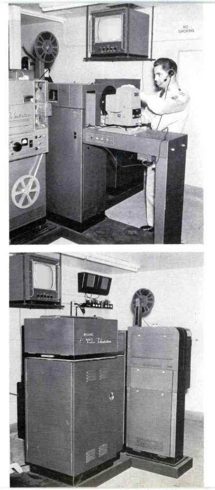
FIG. 13. Central film area in AFIP building serves the entire Walter Reed Army Medical Center. Operation can be controlled locally, or remotely from master control.
