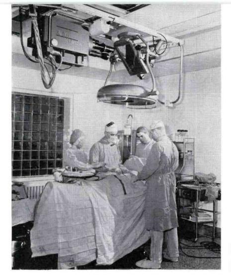
FIG. 9. Medical Color TV Camera is always focused on operating field by means of a mirror used in combination with a special ceiling light, which has a hole in center. Mirror movement and lens switching are remotely operated from the basement centrol room.
