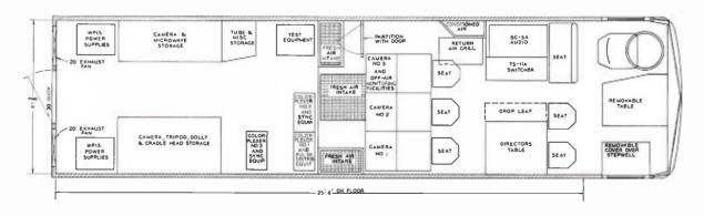
FIG. 1. Plan view of mobile control room.
