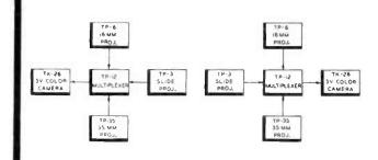
Will handle a large number of inputs and therefore provides maximum program protection. Two completely independent program channels provide the ultimate in reliability and assure continuous programming. Permits previewing in color.
