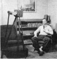
F.G. 9. Live weather casts originate from the engineers' lounge using a TK-21 camera mounted on a tripod.
