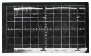
FIG. 5. Test pottern at the left represents a signal which is down 12 db. Input waveform to amplifier at -12 db is shown above as lower waveform on dual-trace scope. Waveform at top represents amplifier output at level of one volt—with each large scale division equal to  $\frac{1}{2}$  volt. In this case the amplifier has been adjusted for 12 db of reserve gain.
