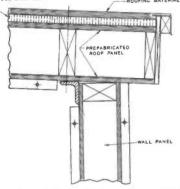
FIG. 15. Cross section of the transmitter house roof showing construction details.
