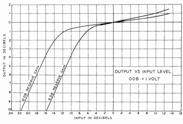
FIG. 4. Output-versus-input curves for 12 db and 6 db gains in the Video AGC Amplifier.
