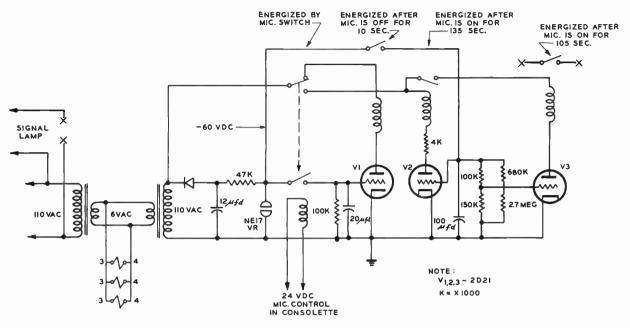
FIG. 3. Schematic diagram of automatic announcer timer used to limit announcing time at WGTO. The announcer timer is keyed when the microphone switch is thrown.
