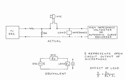
FIG. 4. Circuit used to measure the effect of load upon frequency response of a microphone. The actual circuit is shown at the lop and the equivalent circuit at the bottom.
