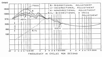
FIG. 3. Plot of output impedance versus frequency of a high-sensitivity ribbon microphone of 250 ohms nominal impedance.
