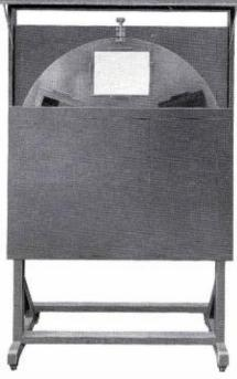
FIG. 5. Front view of television test chart transparency stand developed at NBC.
