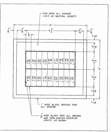
FIG. 4. Proposed RETMA 8 by 10 inch Logarithmic Transmission Transparency.
