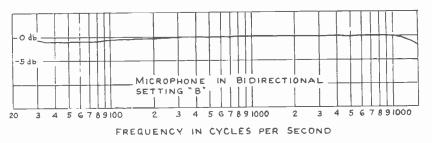
FIG. 5. Frequency response relative to no load with the microphone of Fig. 3 loaded by the preamplifier shown in Fig. 1.
