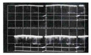
FIG. 6. The monoscope pattern at the left shows a normal one-volt signal at the AGC amplifier unit. Above, input and output waveforms are both at a level of one volt.
