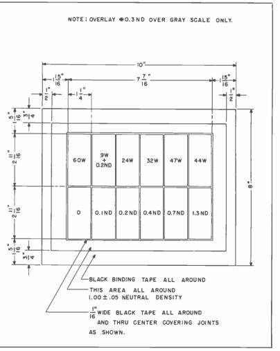
FIG. 7. NBC Color Bar Transparency is made up of pieces of Eastman Kodak Wratten filters.
