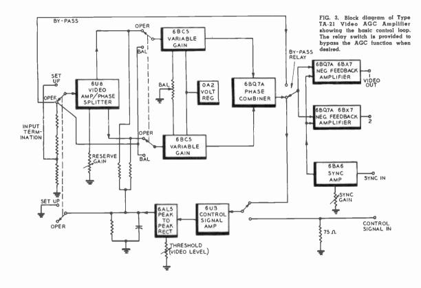
Most television stations, for one reason or another, are plagued with changes of video level. These changes usually occur suddenly and without warning. Manual correction is not fast enough. To fill the need for a fast automatic level-correcting device, RCA and NBC engineers\* have developed the TA-21 Video AGC Amplifier as shown in Fig. 1.
