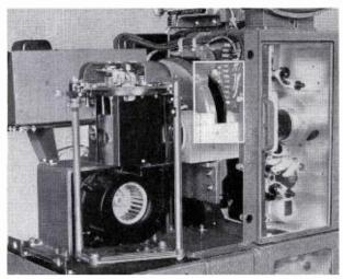
FIG. 7. Variable neutral density disk mounted in a TP-35CC Projector.
