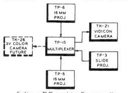
Combines a TK-21 monochrome film camera with projectors and multiplexing equipment, which are usable in color as well as monochrome. At any time a TK-26 color film camera can be odded, retaining the TK-21 for the monochrome channel.
