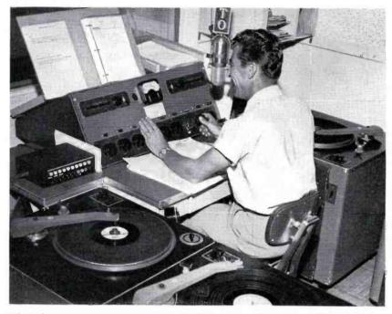
FIG. 5. Close-up view of studio control room BC-2B Consolette and turntables. A BA-12A Utility Amplifier is used as a booster amplifier in each turntable.
