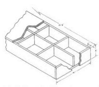
FIG. 14. Construction diagram of prefabricated plywood roof panels.
