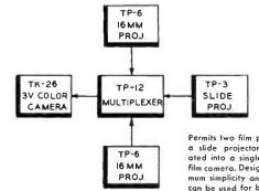
Permits two film projectors and a slide projector to be operated into a single TK-26 color film camera. Designed for maximum simplicity and economy, it can be used for both color and monochrome film.
