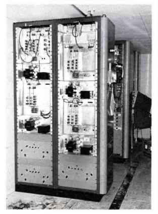
FIG. 15. Camera control room in AFIP building handles three studio cameras, the autopsy camera, and the film camera (also inputs from other areas to which studio cameras may be moved).
