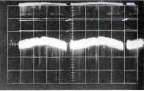
FIG. 7. The AGC amplifier has a signal pulldown range of about 12 db. A signal of +12 db is shown at the left. Above, the lower waveform shows the input signal and the upper waveform shows the one-volt output of the video AGC amplifier.
