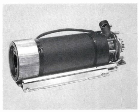
FIG. 9. Orbiting coil installed on the focus coil assembly. Note it is placed over the focus coil for use with latest model RCA monochrome cameras.
