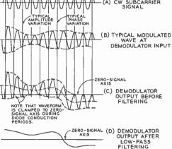
FIG. 10. Waveform sketches illustrating operation of the clamp-type demodulators used in the TM-21.
