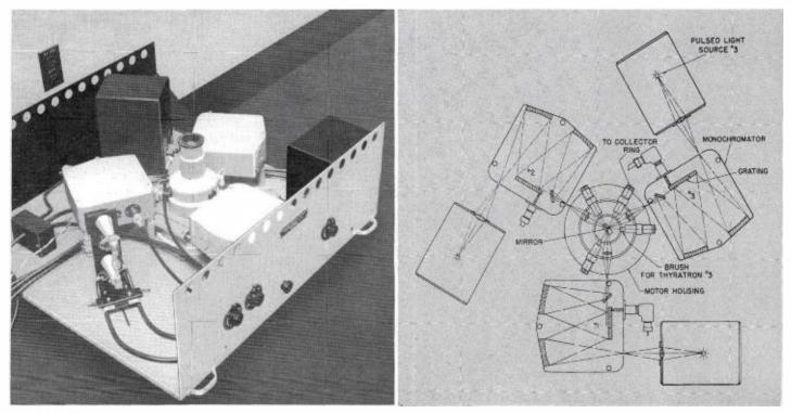
FIG. 4. Illuminating system for Ultraviolet Color-Translating Television Microscope.
