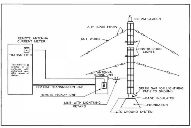
FIG. 19. This is a typical single tower system. Note how the remote antenna current is measured at the transmitter, also observe the position of the tower lights.
