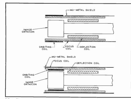
FIG. 6. Diagrams showing how electromagnetic orbiter is mounted on present (top) and earlier (bottom) models of RCA monochrome cameras.
