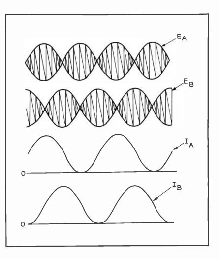
FIG. 11. Waveforms of stator output signals.
