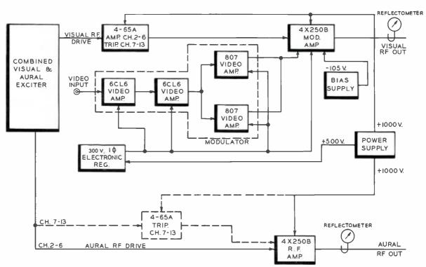
FIG. 2. Simplified block diagram of the TTL-100AL/AH Transmitter.
