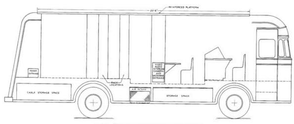
FIG. 6. Side elevation view of mobile control room.
