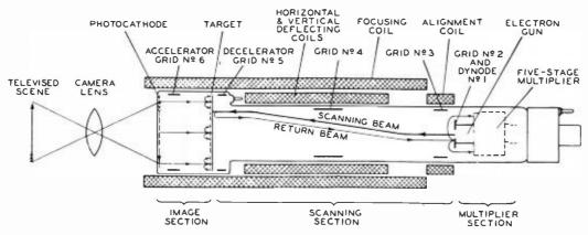
FIG. 5. Schematic diagram of the image orthicon tube showing focus and deflection coll assemblies.
