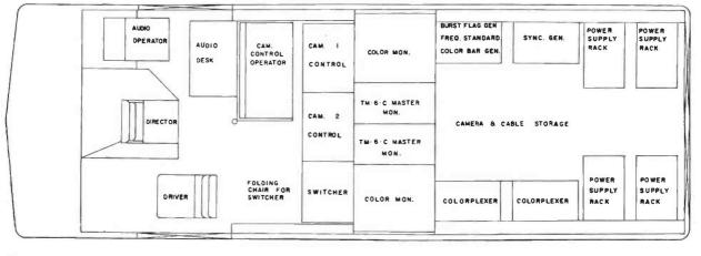
FIG. 18. Plan view of KHQ-TV color mobile unit.
