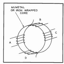
FIG. 7. Sketch showing quadrature windings on mumetal core.
