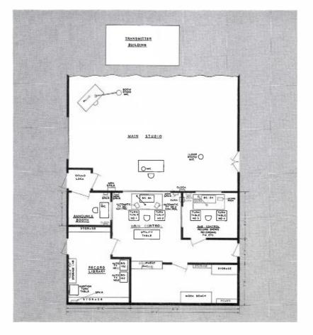
FIG. 3. Layout for Plan "C." Here the studio and transmitter are located in separate buildings. This is the studio plan (Fig. 6 shows the transmitter plan). This is a design for the larger, communitytype station.
