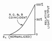
(D) NORMALIZED CURVES AFTER CORRECT ADJUSTMENTS
