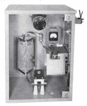
FIG. 21. This is an antenna tuning unit for a 1.KW station: it is usually located at the base of the tower. The lighting choke colls are shown in topcenter of cabinet.
