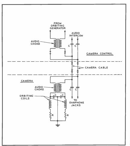
FIG. 13. Schematic diagram showing how the orbiter can be remotely controlled via audio intercom lines.
