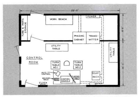
FIG. 5. The control room of Plan "B" is shown here with the phasing equipment added. (The phasing equipment is required for feeding a directional antenna system.)
