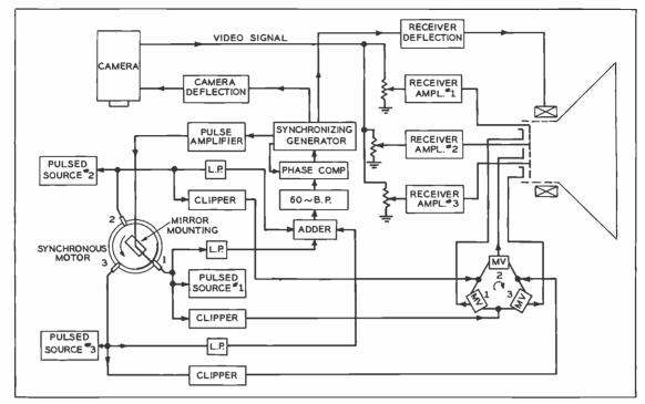
FIG. 3. Block diagram for Ultraviolet Color-Translating Television Microscope.
