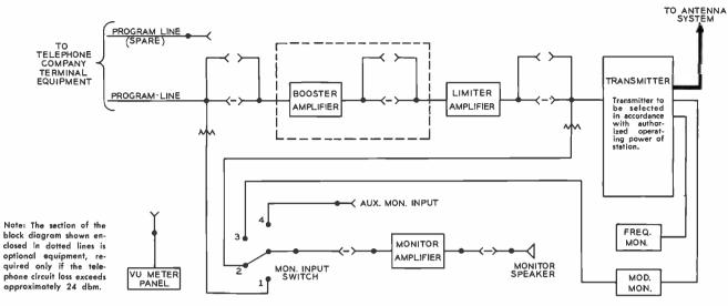
FIG. 9. This block diagram shows how the input and monitoring equipment are connected. The booster amplifier is necessary if line loss from the studio exceeds 24 dbm.
