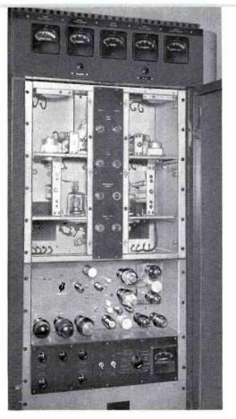
FIG. 3. Open view of the TTL-100AH VHF TV transmitter showing aural visual r-f cubicles, and modulator chassis and control panel mounted below.
