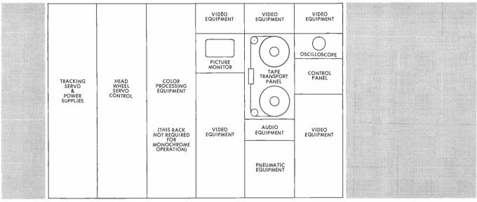
FIG. 5. Rack layout of the Color Video Tape Recorder. Only three racks (shown right) are required at the operating position. Remainder can be remotely located.
