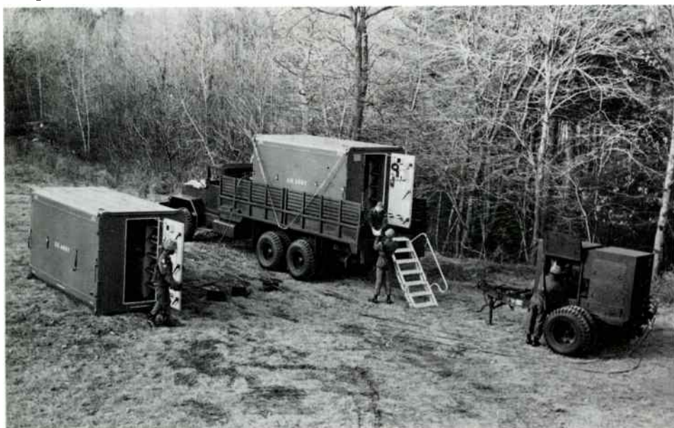
Missile components are tested automatically in the ATE's Land-Combat Support System.
