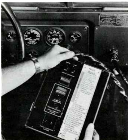
Vehicle readiness unit cuts time Army has to spend diagnosing vehicle problems.
