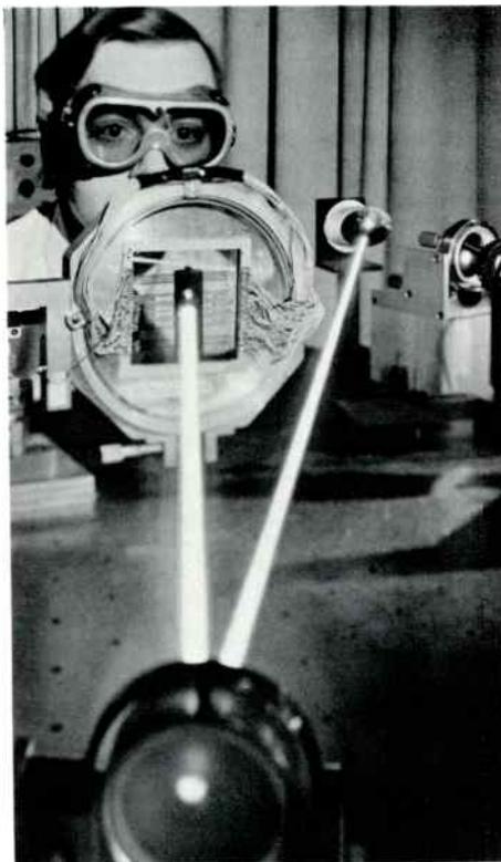
Dr. Wilber C. Stewart and an optical memory laser beam developed at Princeton that writes, stores, reads, and erases information.
