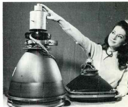
The shorter, lighter in-line tube (right) provides sharper color pictures.
