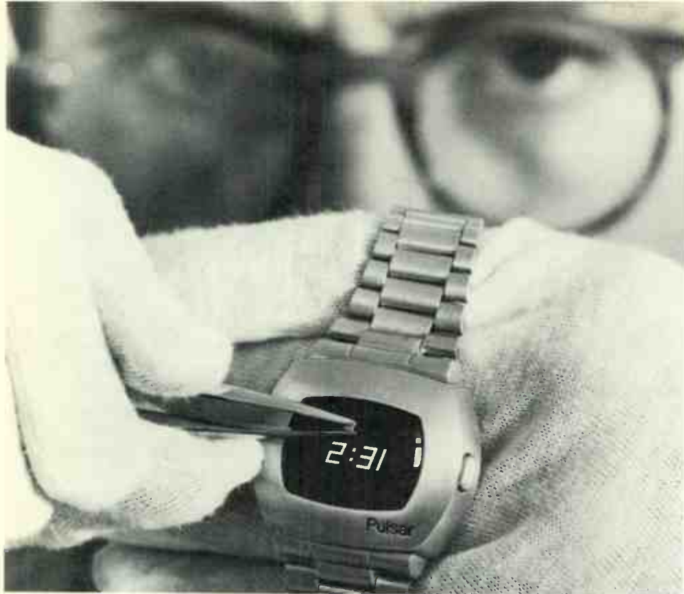
How many angels on the head of a pin? This solid state integrated circuit contains over 1,200 transistors, enabling an all-electronic wristwatch to keep time within a minute a year.
