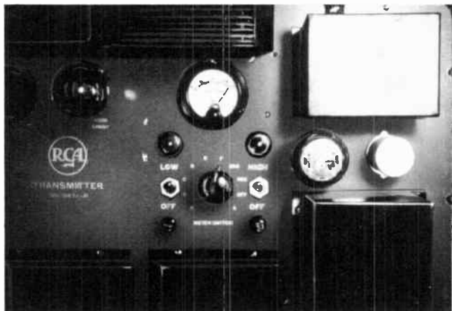
Fig. 8—View of RCA Microwave equipment showing the test switches and meter for voltage checks.
