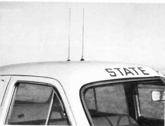
Directional antennas on mobile units and station towers provide effective coverage of turnpike with minimum "spill-over" into adjacent areas
