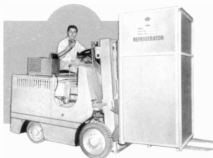
Semi-portable "Carfone" on Fork Lift keeps operator in touch with dispatcher
