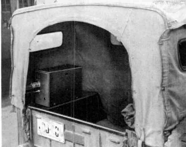
Mobile "Fleetfone" unit mounted in jeep truck
