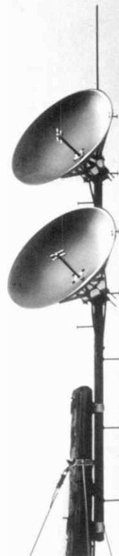
Fig. 4—Closeup of parabolic reflector antenna showing the polarization of the dipoles (top set vertical and bottom set horizontal). Note also the reflector dipoles at the outermost end of the focal support.
