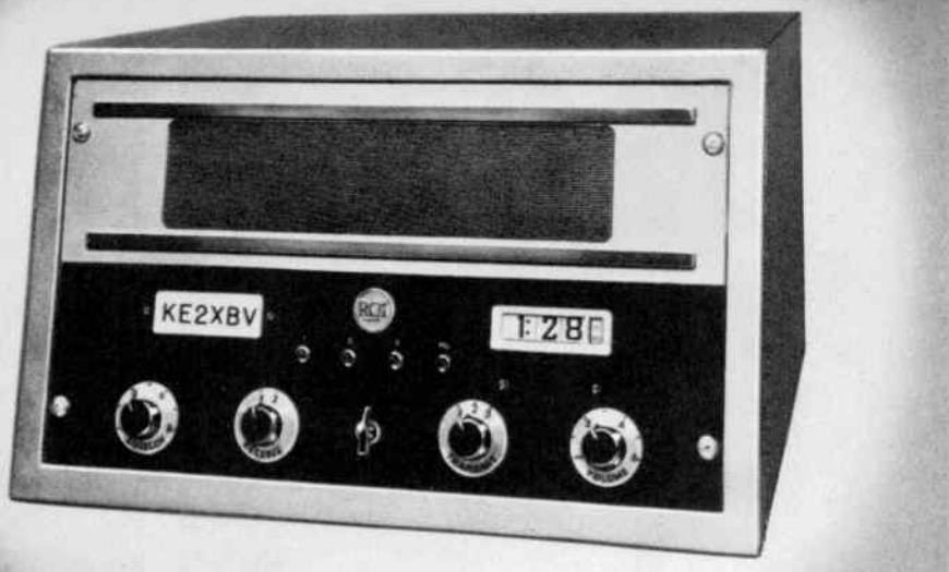
Front view of station console equipped for three transmitting and two receiving frequencies
