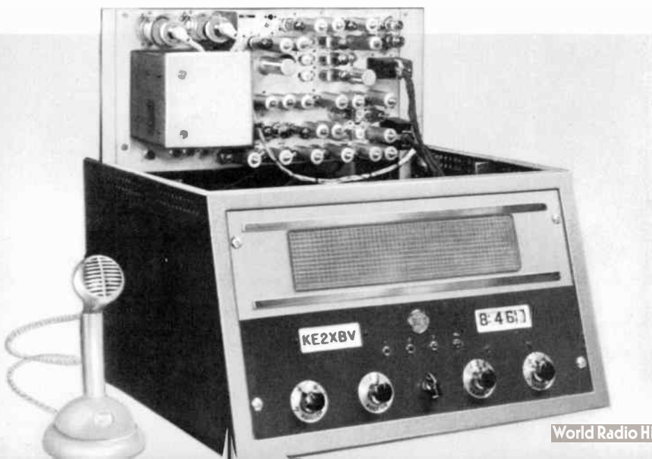
All important circuits can be serviced from front of chassis
