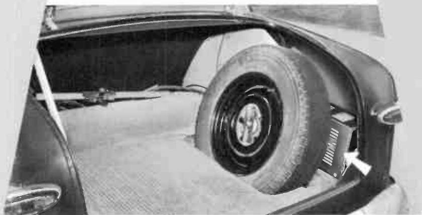
"Carfone" mobile radio fits easily behind the spare tire
