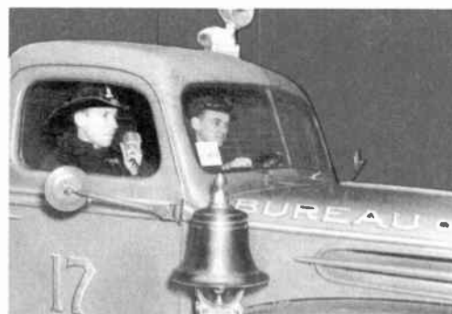
Pumper truck, one of 150 radio-equipped mobile units. Close-up shows RCA "Carfone"
