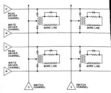
Fig. 7—Portion of the 32 x 32 bipolar matrix.
