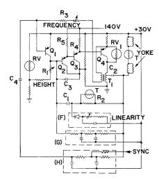
Fig. 4—Schematic diagram of complete TV vertical deflection circuit.
