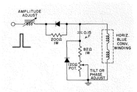
Fig. 12—Horizontal blue convergence circuit.
