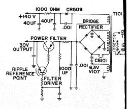
Fig. 3—Power supply, simplified schematic.
