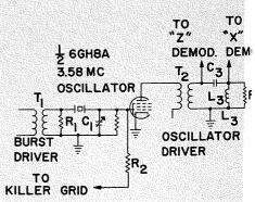
Fig. 3—Simplified 3.58-MHz oscillator circuit.
