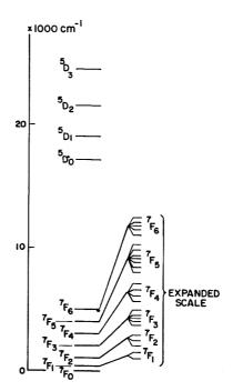
Fig. 6—Generalized energy level diagram for  $\mbox{Eu}^{+3}$  ion.
