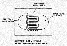
Fig. 2—Geometry of RCA 40235 silicon transistor.
