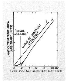
Fig. 3—The effect of voltage on efficiency which leads to the concept of "dead voltage."
