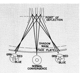
Fig. 3—Horizontal misconvergence; convergence errors due to horizontal deflection of electron beams.
