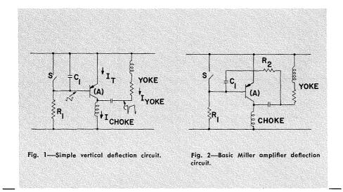
THE purpose of the vertical deflection circuit is to drive a 60-Hz (c/s) sawtooth current through the vertical yoke windings. In most transistor circuits this is done using a voltage sawtooth generator consisting of  $C_1$ ,  $R_1$ , and switch S (Fig. 1). Switch S is open during trace and closed during retrace; the resultant voltage is amplified by the transistor to provide the required current in the yoke.
