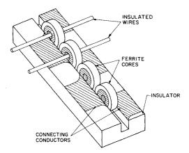
Fig. 4-Ferrite core strip.
