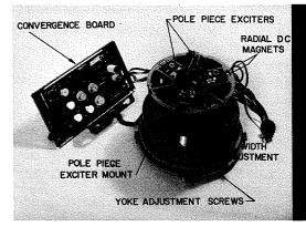
Fig. 11—Yoke mount and accompanying devices.
