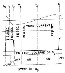
Fig. 2—Output-stage currents and voltages.
