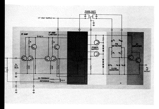
Fig. 1—Schematic diagram of integrated circuit chip used for intercarrier sound function in TV receivers.
