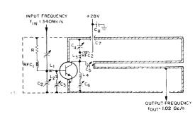
Fig. 6—RCA-2N4012 tripler circuit (340 MHz to 1.02 GHz).
