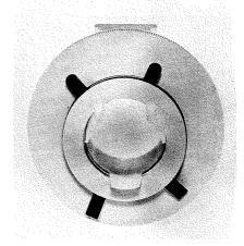
could be minimized if the pole pieces were not used. Consequently the guns for the new rectangular tubes were designed without internal lateral-converging pole pieces. The electron gun assemblies of the 25- and 19-inch tubes are identical. This electron-gun assembly is shown in Fig. 5. The gun assembly used in the 15-inch color picture tube is shown in Fig. 6, which reveals the differences between the Einzel-lens gun and the bipotential gun structure shown in Fig. 5.
