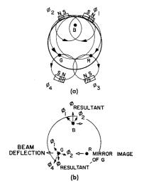
using an internal magnetic strap. This strap directed a magnetic flux field perpendicular to the blue electron beam and perpendicular to the horizontal center line of the tube. The magnetic field was supplied by a permanent magnet mounted on the neck of the tube adjacent to the strap; the blue beam could be moved horizontally by varying the effective strength of the magnet.
