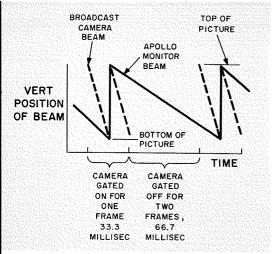
Fig. 4—Vertical deflection and camera beam timing.
