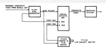
Fig. 6—Simplified diagram of genlock system.
