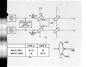
carry digit pulses and sense signals without distortion. The two-core-per-bit scheme of Fig. 1 uses paired digit lines. Since either of the two lines of a pair is always driven by a digit pulse, regardless of whether a I or a  $\theta$  is being written in, digit pulse propagation can be considered a superposition of a differential-mode component and a commonmode component (Fig. 2) with current amplitude one-half that of the digit pulse on each line.
