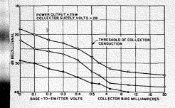
Fig. 5-Intermodulation distortion as a function of forward bias at peak envelope power of 25 watts.
