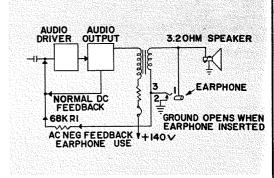
Fig. 2—Audio output with earphone operation, simplified schematic.
