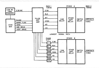
Fig. 2—Two-studio color plant timing. Studio A composite video output is the longest signal-path time of plant. Studio B composite video output must be made equal to Studio A in time by adding delays D1 through D5.
