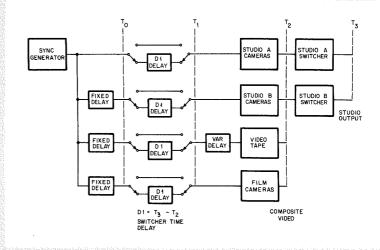
Fig. 4—Switchable pulse delays required for piggyback operation.
