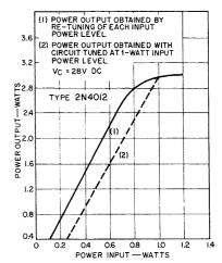
Fig. 7—Power output vs. power input; RCA-2N4012 tripler circuit (340 MHz to 1.02 GHz).
