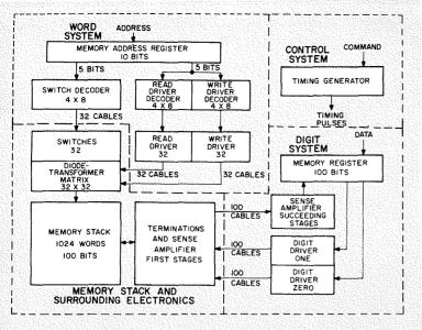
Fig. 6-Block diagram of the memory system.
