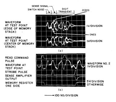
Fig. 11—Waveforms at sense amplifier test points: a) regeneration of 1's and 0's, and b) regeneration of 1's and 0's at 450-nsec cycle time.
