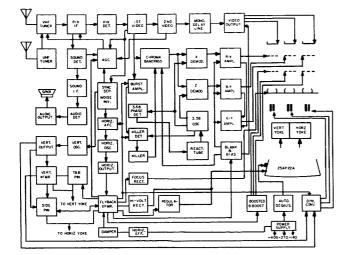
Fig. 1—Block diagram of main circuit stages of the CTC-17, 25-inch color TV receiver.
