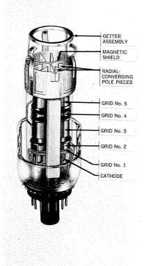
Fig. 6—Electron gun assembly of the 15-inch color picture tube.
