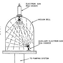
—Diagram showing location of master and auxiliary guns in high-vacuum-system chamber for maximum coverage of surface area.
