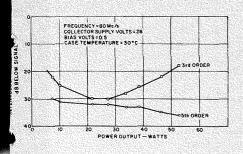
Fig. 4-Third- and fifthorder intermodulation distortion of RCA Dev. No. TA2656 as a function of output power at 80 MHz.
