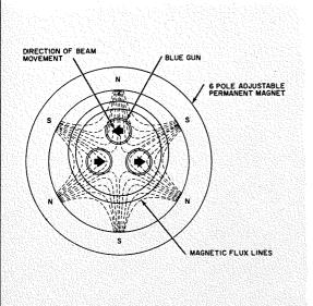
Fig. 8—Flux pattern of 6-pole lateral-converging assembly.
