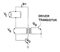
Fig. 13—Base voltage associated with basic blocking oscillator.
