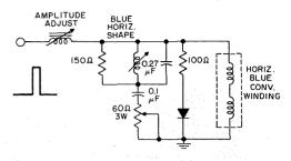
Fig. 11—Basic horizontal blue convergence circuit of RCA CTC-17.
