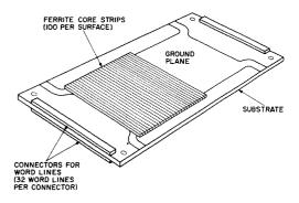
Fig. 5—Memory plane construction.
