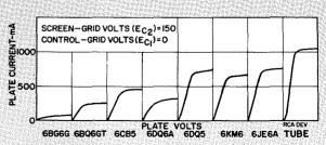
Fig. 2—Plate current as a function of plate voltage for typical horizontal-output tubes developed from 1946 to present, arranged in order of development.
