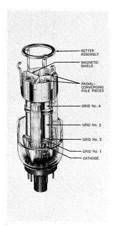
Fig. 5—Electron gun assembly of 19-inch and 25-inch color picture tubes.
