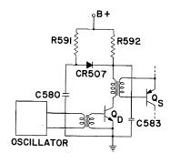
Fig. 9-Base-waveshaping circuit of driver.
