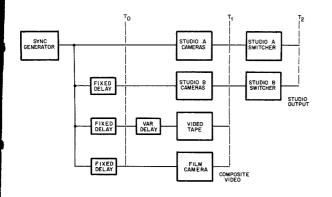
Fig. 3—Simplified version of two-studio TV plant with video tape and film facilities.
