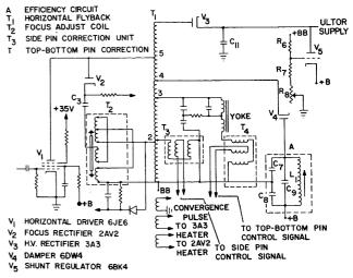
Fig. 2—CTC-17 horizontal and high-voltage circuit.
