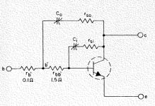
Fig. 5—Simplified circuit for varactor portion of PCA-2N4012
