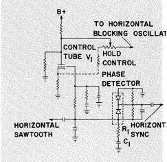
Fig. 2—Horizontal AFC circuit.
