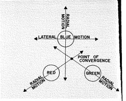
Fig. 4—Center convergence; radial motion accomplished by DC magnets in pole piece exciters, lateral motion accomplished by blue lateral device.
