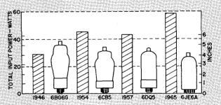
Fig. 1—Evolution of size and shape of horizontal-output tubes, together with increase in total power input from 1946 to 1965.
