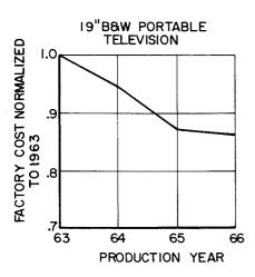
Fig. 1—Reduction in costs obtained in production of 19-inch, monochrome, portable TV receiver.
