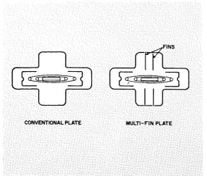
Fig. 5—Cross-sectional views illustrating conventional twopiece plate structure and the multi-fin plate structure.
