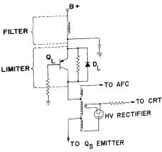
Fig. 4—Current-limiting circuit for output transistor protection.
