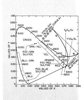
Fig. 7—Location on a chromaticity diagram of the emission colors of phosphors used in color TV. Also shown on the red-orange monochromatic locus are curves showing how the eye sensitivity and the broad-band emission of the red sulfide phosphor are mismatched.
