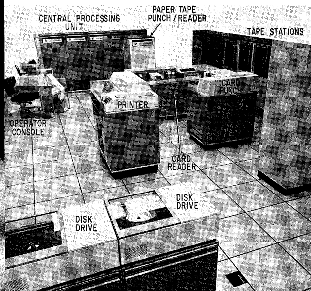
Fig. 1—Typical arrangement of equipment in a scientific computer center.
