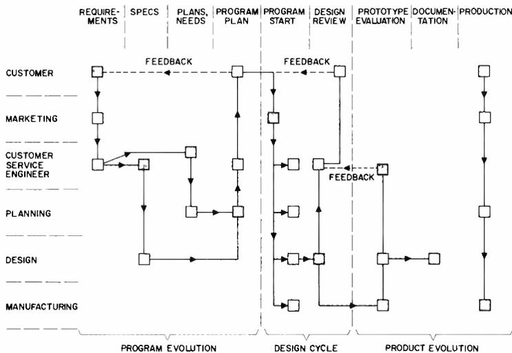
Fig. 6—Pencil-tube supplier-customer interaction.
