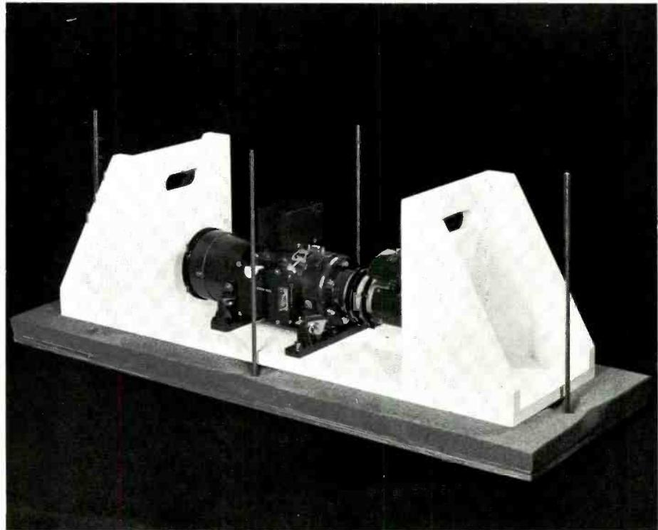
Fig. 3—A satellite camera mounted on the baseboard and lower cushioning material of the sandwich pack.
