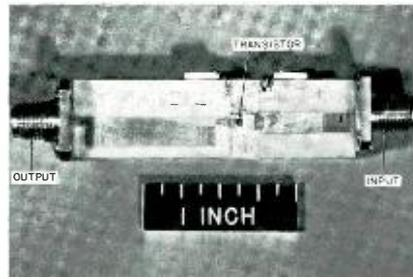
Fig. 4a—L-band transistor amplifier  $P_{in}=1$  watt;  $P_{out}=7$  watts; center frequency=1450-MHz; bandwidth=10%; efficiency=55% (courtesy Dr. D. Stevenson).
