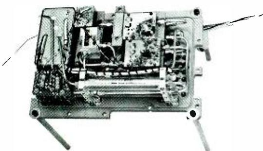
Fig. 5b—Electronically tunable missile local oscillator; photo and block diagram.
