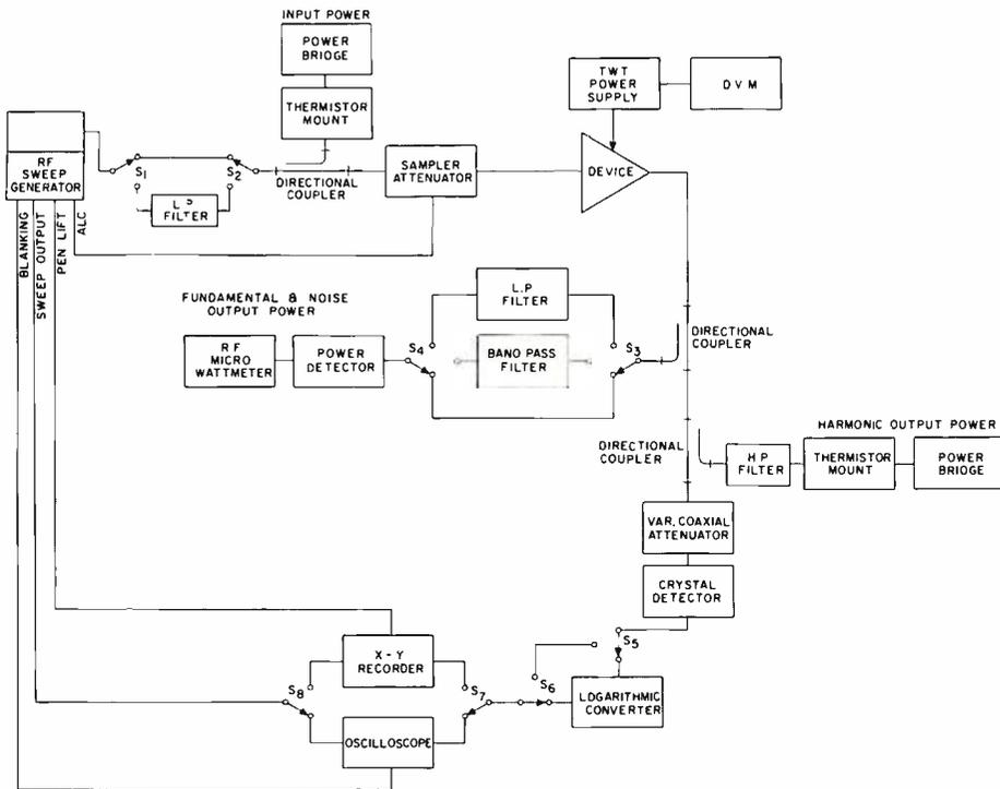
Fig. 1—Block diagram of TWT production test system.
