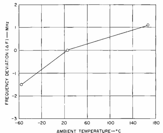
Fig. 7—Typical behavior of frequency stability as a function of ambient temperature.
