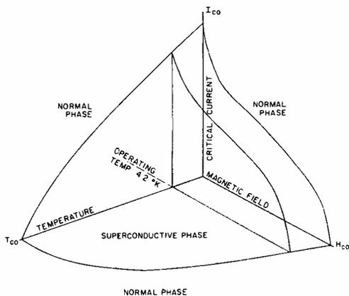
Fig. 1—The generalized critical surface of a high-field superconductor.
