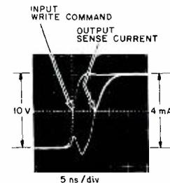
Fig. 3—Total delay from write command to sense current.
