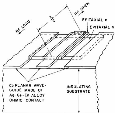
Fig. 6—Distributed oscillator (electromagnetic-wave wavelength,  $\lambda$ , based on dielectric constant on  $N$ -material, including electrons).
