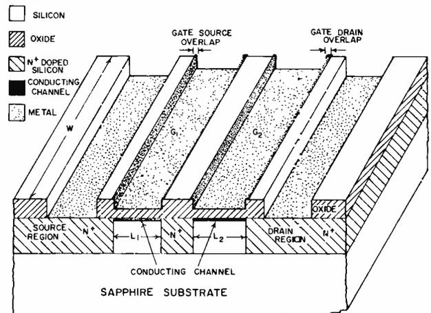
Fig. 4—Cross section of tetrode transistor.
