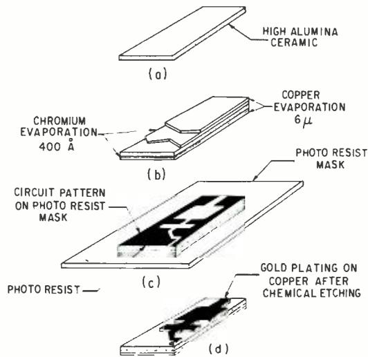
Fig. 3—Sequence of steps involved in making microstrip circuits; note that every step in the fabrication process lends itself to batch processing.
