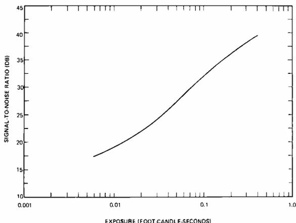
Fig. 5—S/N vs exposure for RBV camera.
