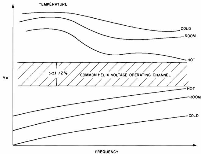
Fig. 9—Helix mode storage plot as a function of temperature.
