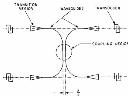
Fig. 8—Surface wave guiding and coupling experiment.
