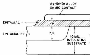
Fig. 4—Sandwich-type transferred-electron oscillator.
