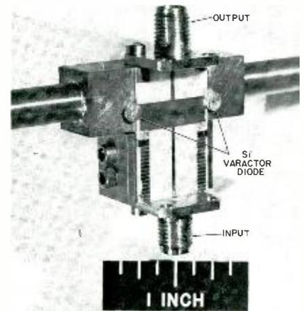
Fig. 4c—Balanced L- to C-band quadrupler: input frequency=1.9 GHz;  $P_{in}=8.4$  watts; efficiency=30% (courtesy Dr. W. W. Siekanowicz).
