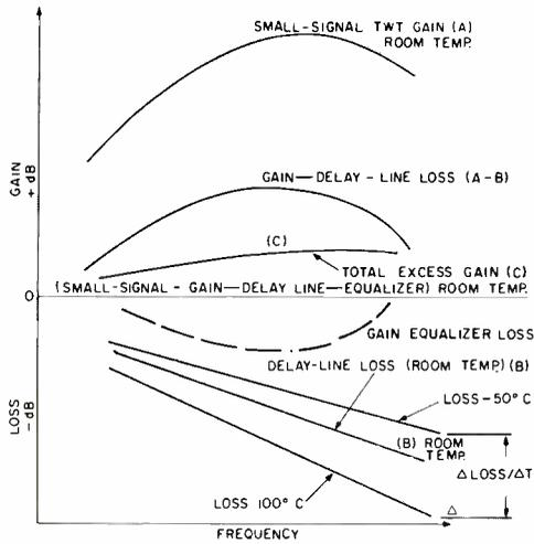
Fig. 8—Tube gain loop loss parameters as a function of frequency and temperature.
