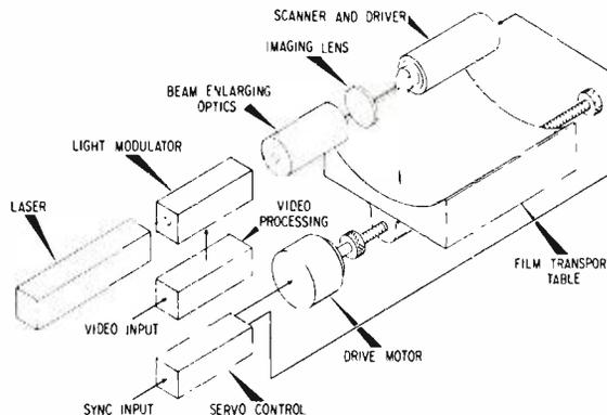
Fig. 7—Laser beam image reproducer.
