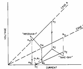
Fig. 3—Idealized voltage-current diagram for a composite superconductor.
