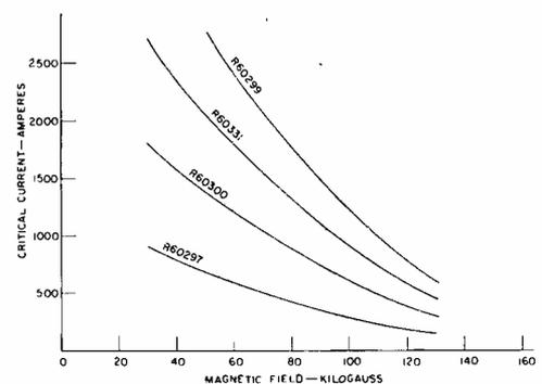
Fig. 6— $H_c-I_c$  characteristics of fully stabilized 1/2-inch wide ribbons.
