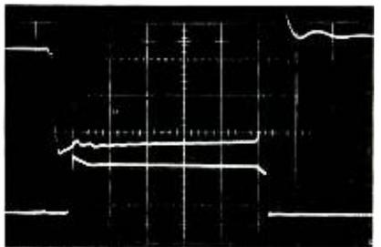
Fig. 6—Top, pulse current at 1 ampere/division; bottom, RF output power at 50 watts/division. Horizontal time scale is  $100\text{ ns}/\text{division}$ .
