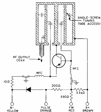
Fig. 4—Schematic diagram of S190 cavity oscillator.
