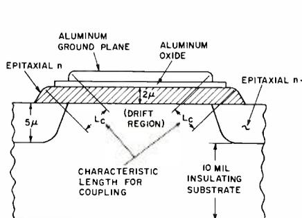
Fig. 8—Traveling-wave amplifier and voltage-controlled phase shifter.
