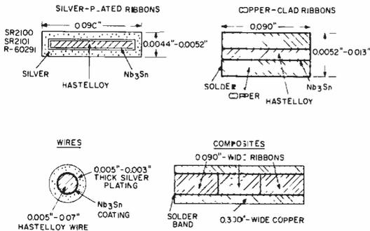
Fig. 8—Typical conductor cross-sections.
