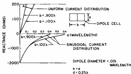
Fig. 4—Radiation reactance of uniform and sinusoidal current dipoles in infinite array;  $L = a$ ;  $d = 0.25$ .
