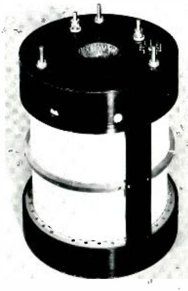
Fig. 11—Two-inch-bore, 100-kilogauss magnet.
