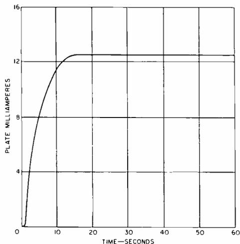
Fig. 2—Typical curve of plate current as a function of time.
