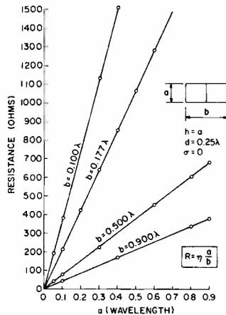
Fig. 2—Radiation resistance of uniform current dipole in infinite array;  $L = a$ ;  $d = 0.25$ ;  $\sigma = 0.001$ .
