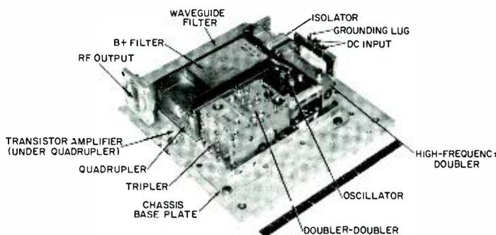
Fig. 5a—Microwave power source for the luna module; photo and block diagram.
