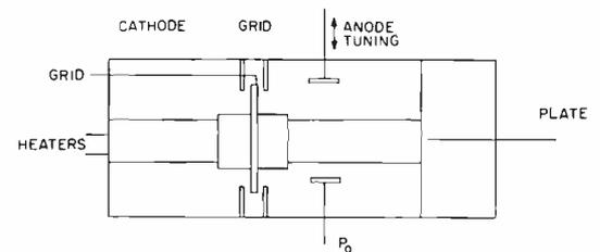
Fig. 6—Cross-section of an oscillator cavity.
