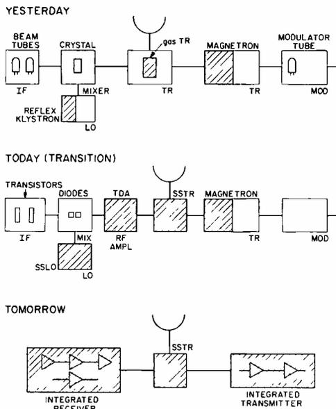
Fig. 2—Evolution of a radar system.
