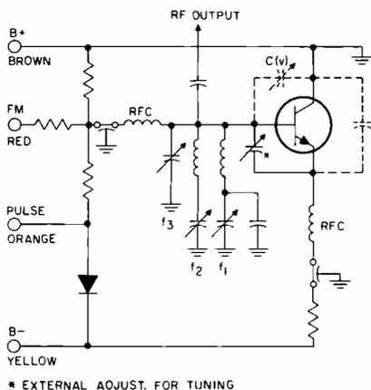
Fig. 1—At the frequency of oscillation (560 MHz) the transistor is terminated in a series resonant circuit. Another series resonant circuit is provided at the second harmonic (1120 MHz) of the frequency of oscillation to improve the efficiency; this is the idler circuit. An RF output greater than 200 mW is obtained at 1680 MHz, the third harmonic of the frequency of oscillation.
