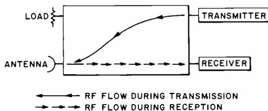
Fig. 1—Simplified schematic diagram of TR switch.
