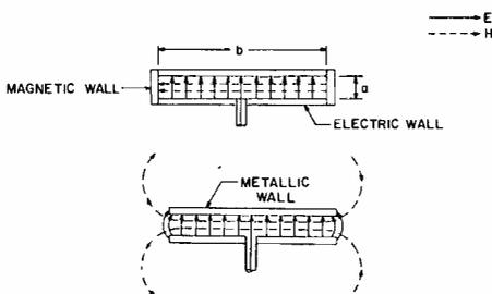
Fig. 6—(a) Electromagnetic field configuration in unit cell; (b) electromagnetic field configuration in single-element array simulator.
