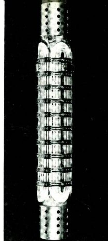
Fig. 15—Four-inch-bore quadrupole magnet.
