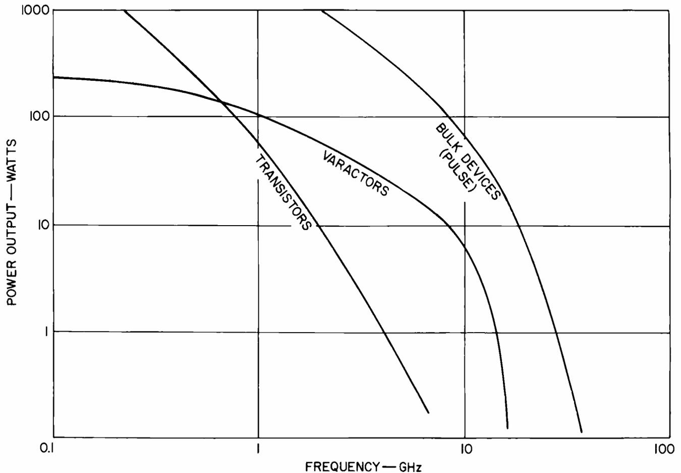
Fig. 1—State of the art in bulk devices compared with varactors and transistors.
