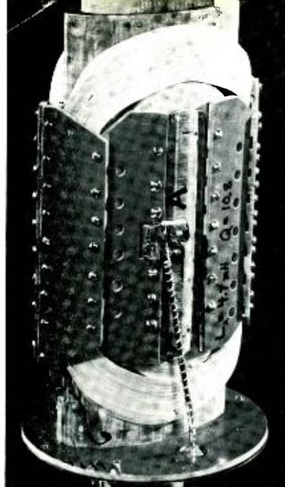
Fig. 14—Elliptical dipole magnet.
