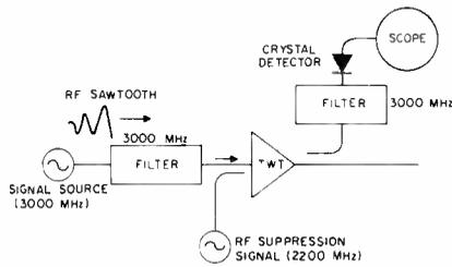
Fig. 7—Transfer characteristics of a traveling-wave tube in the presence of suppression signal at a fixed frequency.
