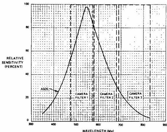
Fig. 4—Spectral sensitivity of ASOS photoconductor.
