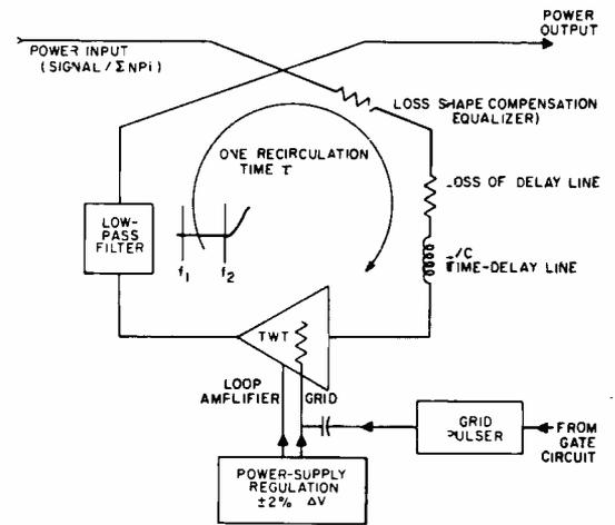
Fig. 4—Off-line recirculating RF memory subsystem.
