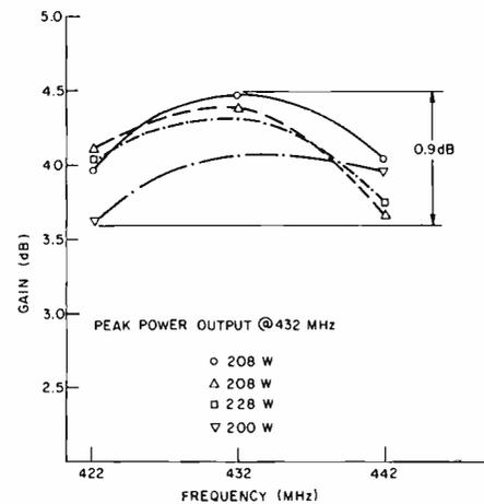
Fig. 6—Comparison of four amplifiers.
