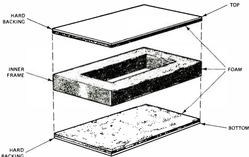
Fig. 1—The sandwich pack consists of three separate parts: cushioning material, rigid backing, and an inner frame.
