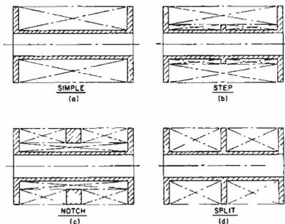
Fig. 9—Construction techniques used to achieve high homogeneity in magnets.
