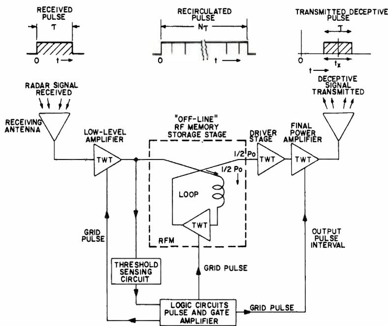
Fig. 1—ECM receiver/transmitter chain.
