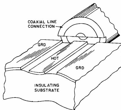
Fig. 2—Coplanar waveguide (after C.P. Wen).
