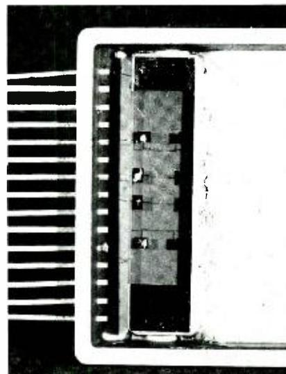
Fig. 3—An experimental acoustic surface-wave delay device employing single-pair transducers on  $LiNbO_3$  substrate. The device is mounted in an integrated-circuit flat pack, emphasizing the compatibility of surface-wave and microelectronic technology.
