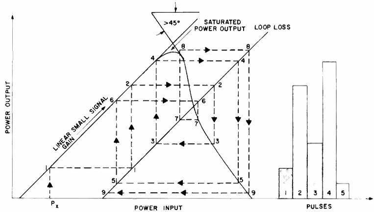
Fig. 6—Faulty (unstable) recirculation caused by poor overdrive slope.
