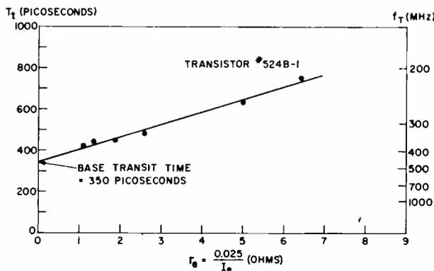
Fig. 7—High-frequency transistor measurements.
