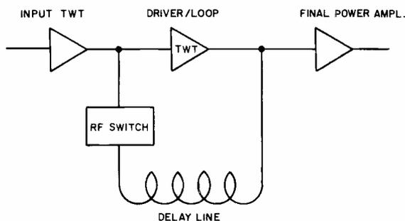
Fig. 11—In-line RF memory storage subsystem.
