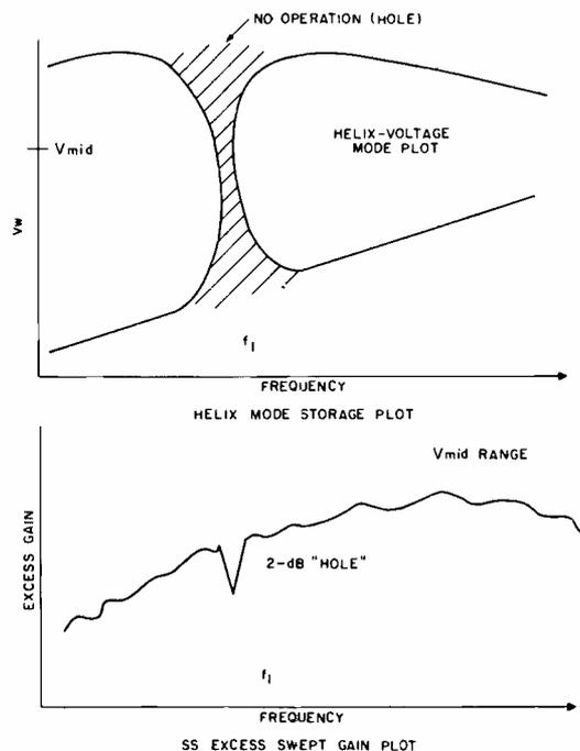
Fig. 10—Plots of helix mode storage (top) and small-signal excess swept gain (bottom).
