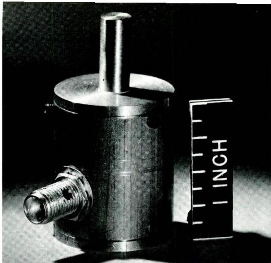
Fig. 9—Experimental X-band transferred-electron oscillator.
