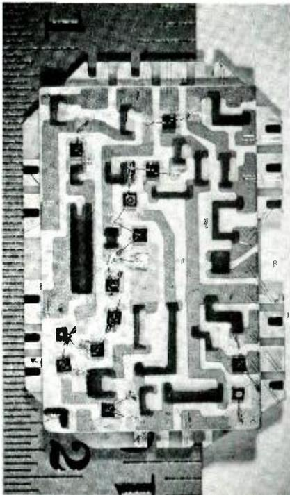
Fig. 8—Photograph of modulator-regulator circuit board.
