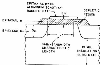
Fig. 7—Field-effect transistor.
