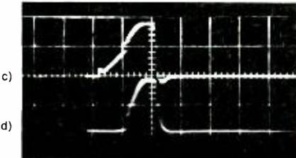
Fig. 5a—Pulse current at 5 amperes/division; b) Pulse voltage at 100 volts/division; c) same as a); and d) RF output power at 150 watts/division. Horizontal time scale for all four tracings is  $0.5\mu\text{s}/\text{division}$ .
