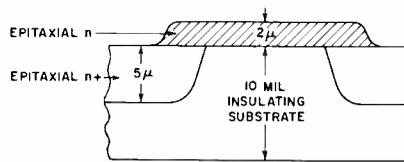
Fig. 5—Coplanar-type transferred-electron oscillator.
