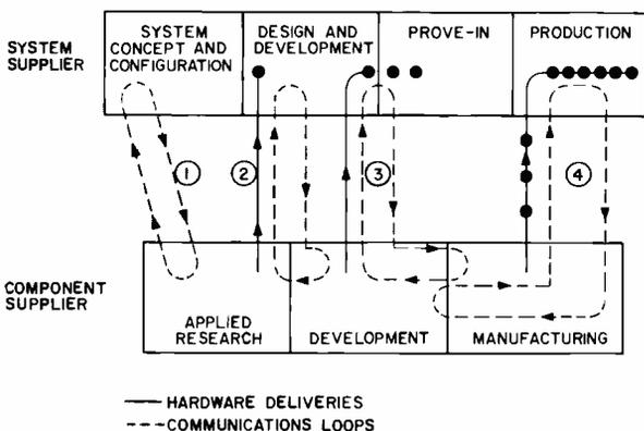
Fig. 3—Interplay between system and component supplier: 1) systems concept and early design; 2) development of subsystems prototype; 3) development of final subsystem; 4) production of final subsystem.
