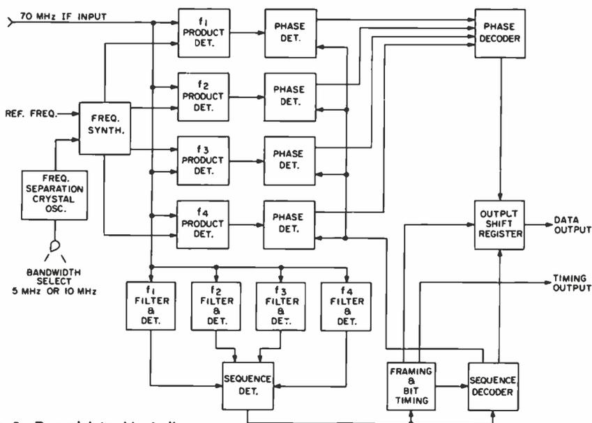
Fig. 2—Demodulator block diagram.
