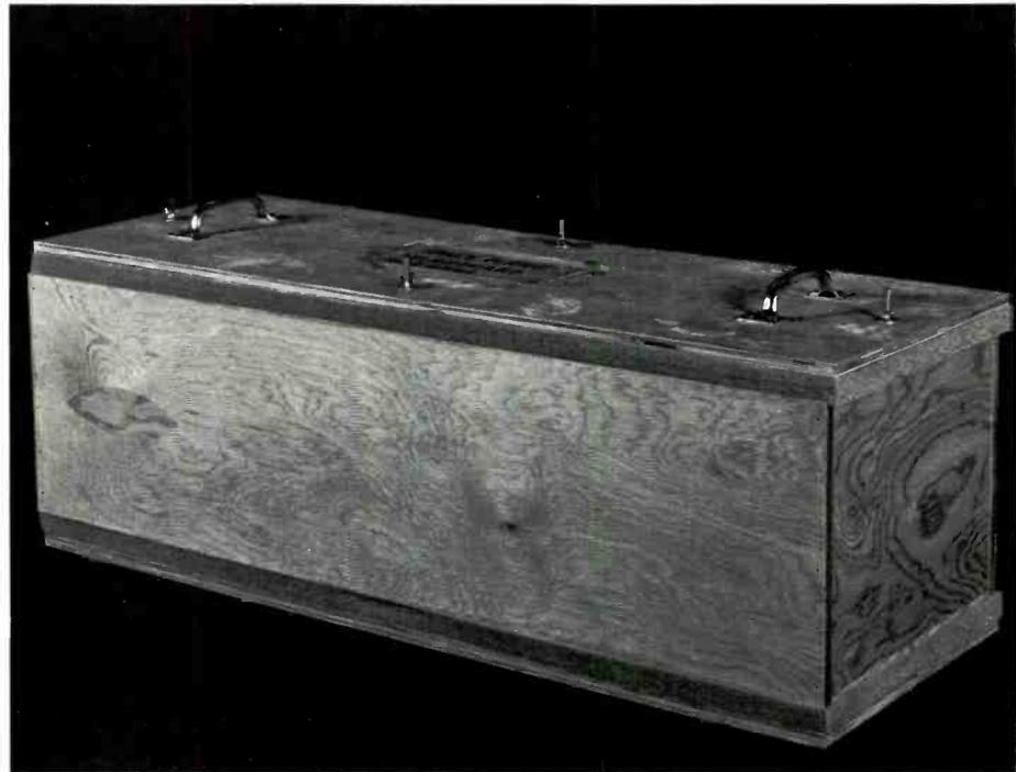
Fig. 4—The inner frame and plywood top and sides are added to the frame shown in Fig. 3 to form a complete shipping container.
