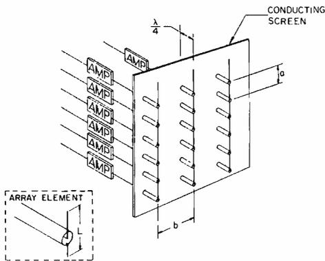
Fig. 1—RF power combination in free space using an array of individually fed, closely spaced dipoles.
