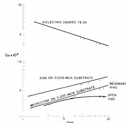
Fig. 1— $Q_u$  of resonators compatible with microwave integrated circuit for alumina dielectric.
