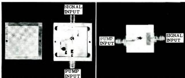
Fig. 1—1.8-GHz amplifier; noise figure = 1.3dB; 3-dB bandwidth = 50 MHz; gain = 16dB; pump frequency = 8.5 GHz; pump power = 5mW.
