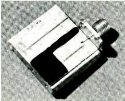
Fig. 3—Sample of open-end microstrip resonator on 0.025-inch-thick alumina substrate.
