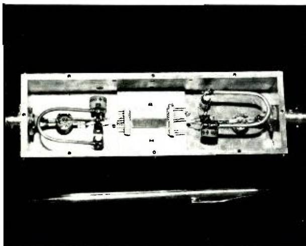
Fig. 6—The 425 MHz delay device.
