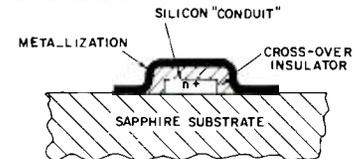
Fig. 2b—Cross section of cross-over technique.
