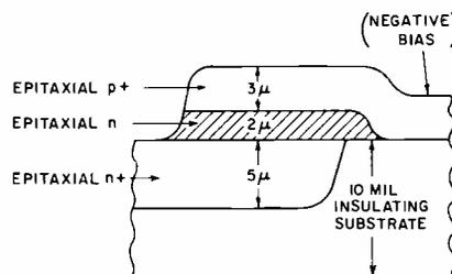
Fig. 3—Varactor diode or avalanche diode oscillator.
