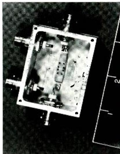
Fig. 2—Acoustic surface-wave delay device employing single-pair transducers on  $ZnO$ .
