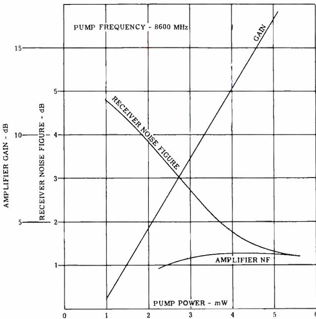
Fig. 5—Gain and noise figure of 1.8-GHz amplifier.
