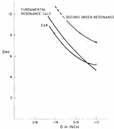
Fig. 4—Resonances of a disk on a 0.025-inch alumina substrate.
