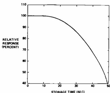
Fig. 3—2-inch RBV storage characteristics.
