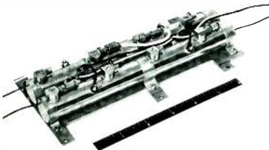
Fig. 7—Transponder package including pencil tubes and cavities.
