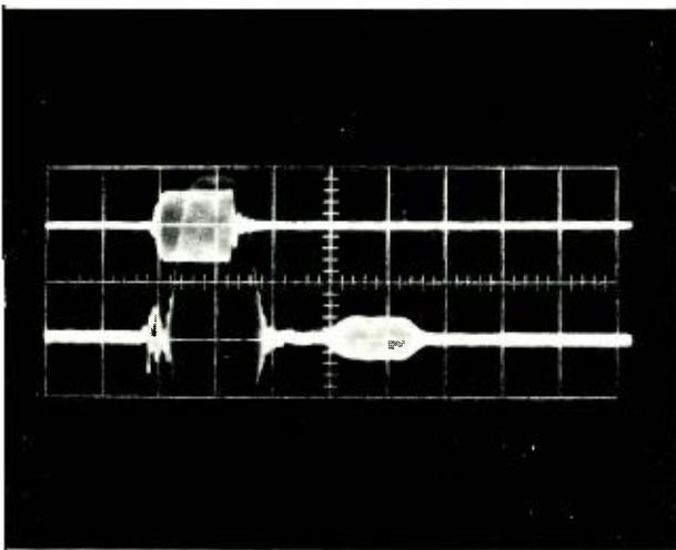
Fig. 5—Measurements of time delay—input signals on upper traces and output signals on lower traces.
