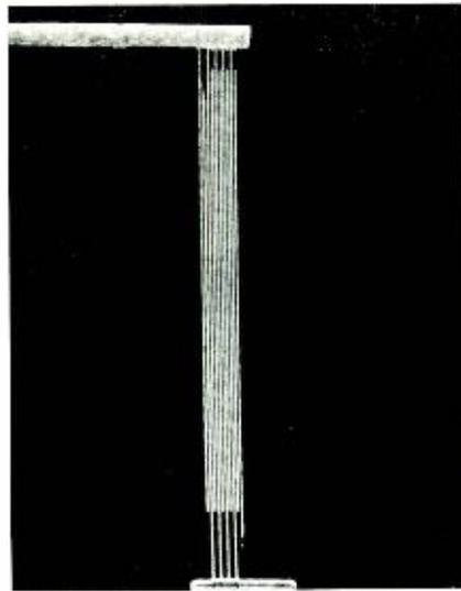
Fig. 7—Transducer pattern formed in photoresist by scanning electron microscope. The lines are 0.34 micron wide placed on 0.68 micron centers.
