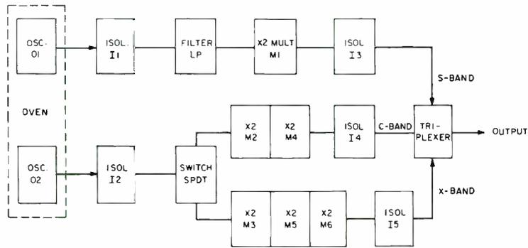
Fig. 1—Block Diagram of solid-state local oscillator.
