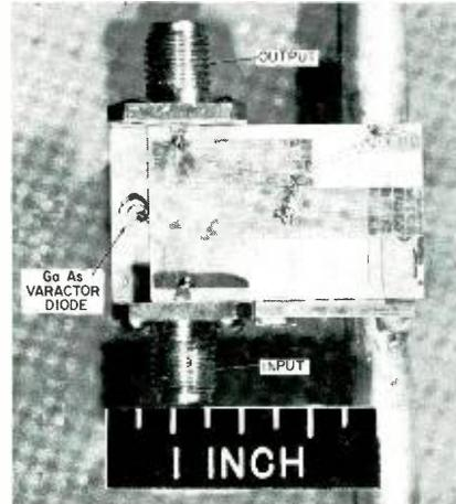
Fig. 4b—Single-ended L- to S-band varactor doubler: center input frequency=1.6 GHz; bandwidth=10%;  $P_{in}=10$  watts; efficiency=53% (courtesy A. Rosen).
