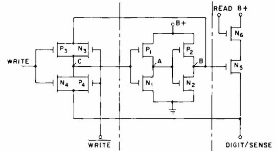
Fig. 1a—Electrical circuit of memory cell.
