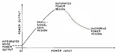
Fig. 3—Power output as a function of power input for a typical traveling-wave tube.
