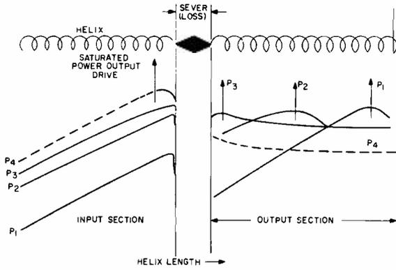
Fig. 2—Saturation position and power output as a function of input drive.
