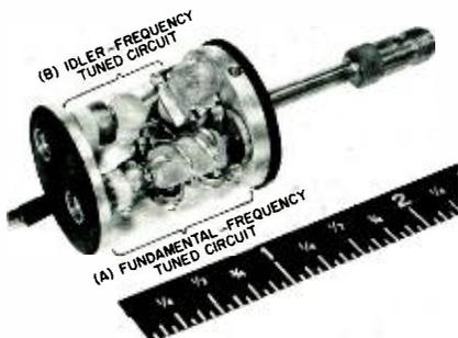
Fig. 2—S170 lumped-circuit transistor/oscillator/multiplier with cover removed to show lumped-circuit elements.
