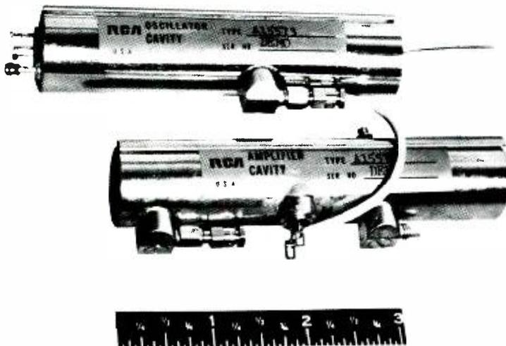
Fig. 8—A typical transmitter chain for Air Traffic Control Beacon Systems.
