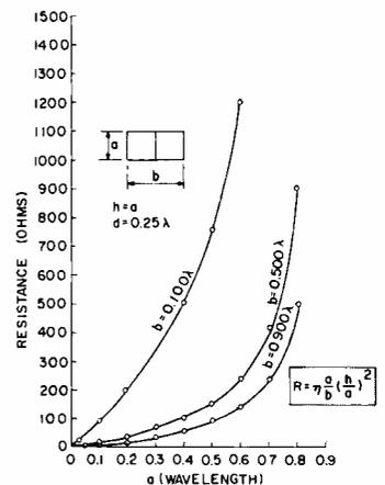
Fig. 3—Radiation resistance of sinusoidal current dipole in infinite array;  $L = a$ ;  $d = 0.25$ .
