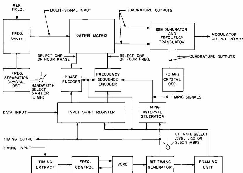
Fig. 1—Modulator block diagram.
