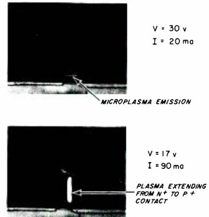
Fig. 9—Microplasma and extended plasma light emission.
