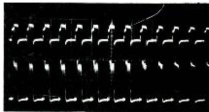
Fig. 8—Multiple pulse bursts: top, pulse current at 5 amperes/division; bottom, RF output power at 150 watts/division. Horizontal time scale is  $2\mu\text{s}/\text{division}$ .
