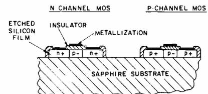
Fig. 2a—Cross section of complementary MOS transistors.
