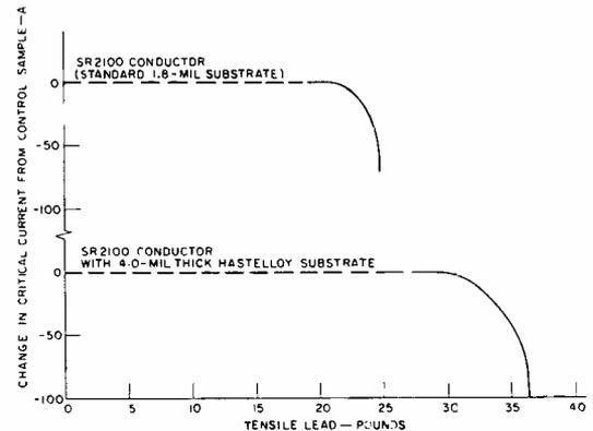
Fig. 4—Critical current of two superconductors as a function of tensile load.
