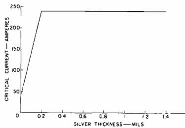
Fig. 7—Effect of silver-plating thickness on short-sample  $I_c$ .
