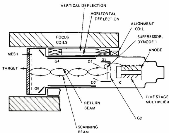
Fig. 2—Return beam vidicon (RBV) schematic diagram.
