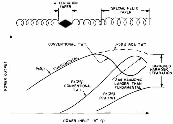
Fig. 3—Fundamental and second-harmonic power output as a function of power-input drive for conventional and improved RCA TWT's.
