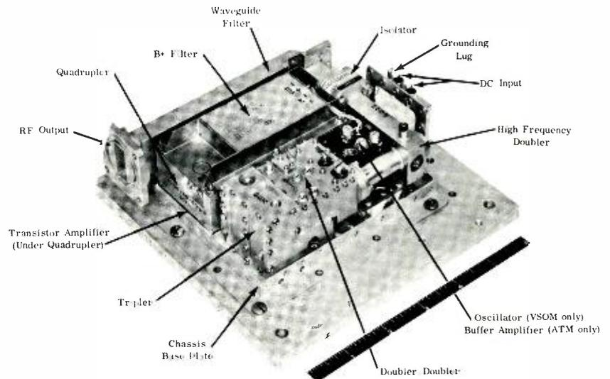
Fig. 5—LM frequency multiplier with chassis cover removed.
