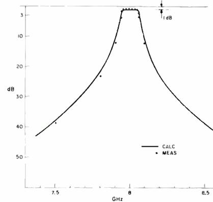
Fig. 8—Response of two-resonator iris-coupled dielectric-loaded waveguide filter.
