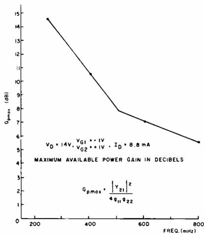
Fig. 5—High-frequency measurements of tetrede.
