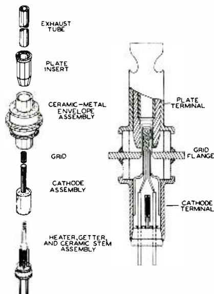
Fig. 1—Basic construction of the pencil tube.
