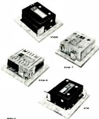
Fig. 4—LM frequency-multiplier subassemblies.
