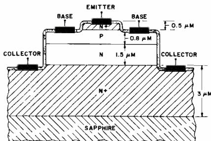
Fig. 6—Cross section through all-epitaxial thin-film bipolar transistor.
