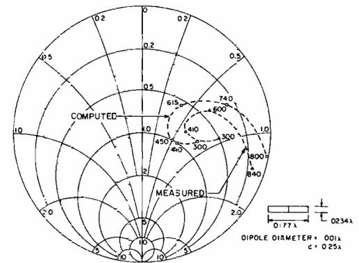
Fig. 8—Impedance of single element array simulator.
