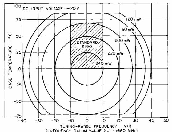
Fig. 5—Minimum power-output capability as a function of case temperature and tuning range for S190 variant.
