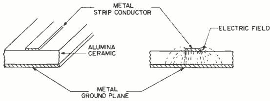
Fig. 2—Section of a microstrip transmission line. In a typical transmission line, the thickness of the ceramic is in the range of 0.02 to 0.05 inch.
