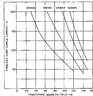
Fig. 5— $H_c-I_c$  characteristics of fully stabilized 90-mil ribbons.
