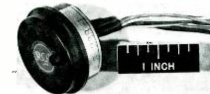
Fig. 4e—Packaged version of oscillator shown in Fig. 4d (courtesy A. Presser).
