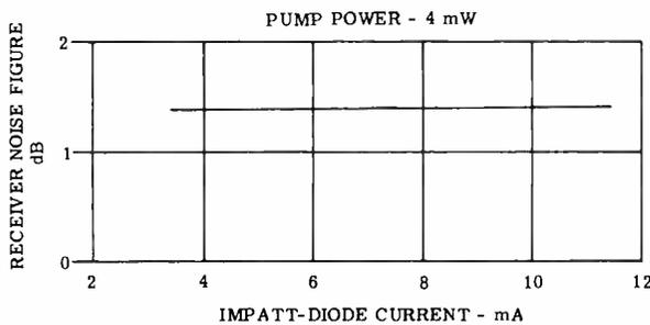
Fig. 6—Noise figure as a function of IMPATT current.
