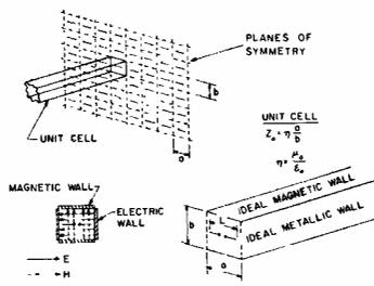
Fig. 5—Unit cell of dipole array.
