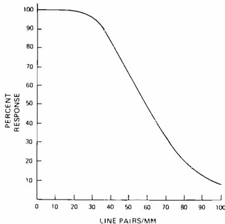
Fig. 6—Modulation transfer function of RBV including lens.
