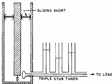
Fig. 3—Coaxial cavity with loop coupling.
