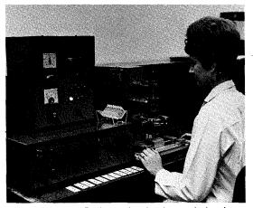
Fig. 5-Resistor trimming by sand abrasion.
