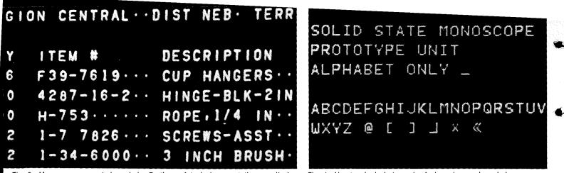
Fig. 2-Monoscope-generated symbols. Portions of typical presentation on display screen. RCA 70/752 Video Data Terminal).
