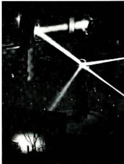
Fig. 8—Photograph showing actual reconstruction of a fixed hologram in  $LiNbO_3$ .
