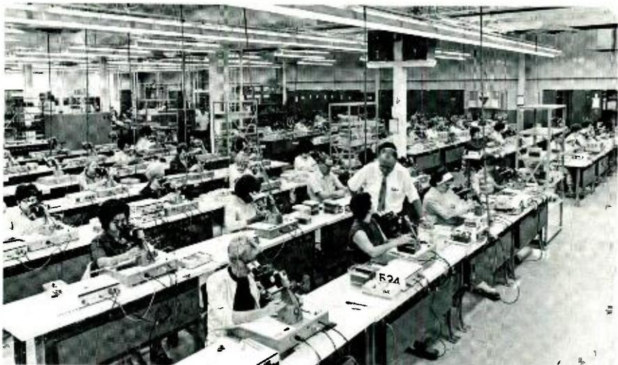
Ultrasonic bonding area for integrated circuit production at Solid State Division plant in Findlay, Ohio.
