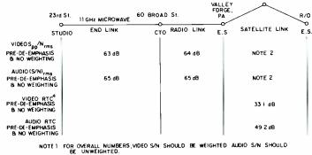
NOTE: FOR THE SATELITE LINK SAN CONFRTC AS FUNCTION OF RAIN CLIMATE NOTE: FOR THE SATELITE LINK SAN CONFRTC AS FUNCTION OF RAIN CLIMATE NOTE: ADD 3dB FOR WEIGHTED VIDEO S/N NOTE: RTCRECEIVER TRANSFER CONSTANT
