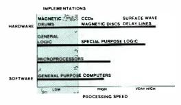
Fig. 3 — Hardware vs. software trade-offs to be evaluated when choosing an implementation approach.
