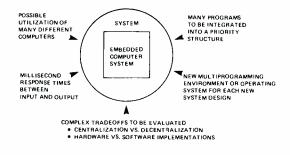
Fig. 1 -- Characterization of real-time systems.
