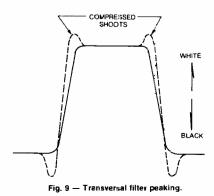
and D2 shown in Fig. 7, the peaking can be compressed in the white direction to prevent spot blooming of the kinescope while still maintaining an enhanced risetime of transitions. Fig. 9 shows the idealized effects of the peaking on a video transition.
