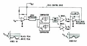
Fig. 1 - Circuit used to establish black level automatically.
