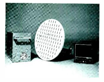
Fig. 4 — PriMUS-20 WXD, a lightweight digital weather radar used by light twin-engine aircraft in the general aviation market.
