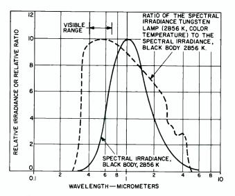
Fig. 1 — Relative spectral irradiance from a black body at 2856 K and the ratio of the spectral irradiance from a tungsten lamp operated at 2856-K color temperature to the spectral irradiance from a black body at 2856 K. Note that in the visible range, 0.4 to 0.7 micrometers, the spectral irradiance from the tungsten lamp closely matches that of a black body.
