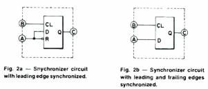
The synchronizer circuit may be implemented in a number of ways, such as with *nor* ot *nand* gates or with a D flip-flop, as shown in Fig. 2(a). While it is necessary that the circuit synchronize the leading edge of the signal at A with the signal at B, it is not necessary that the trailing edge be synchronized. Fig. 2(b) is an example of a synchronizer in which both the leading and trailing edges of the signal at A are synchronized with the signal at B.
