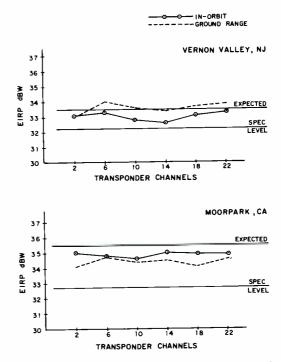
Fig. 2 — Typical EIRP performance (transponders 2, 6, 10, 14, 18, 22).
