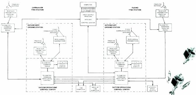
Fig. 8 — RCA Satcom mission operations complex.
