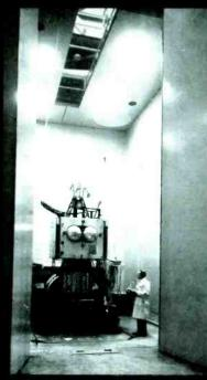
Dick Hartenbaum, AED engineer, ischecking the preparation of the satellite for exposure ic high-level acoustic energy (i.e. noise) simulating the launch environment
