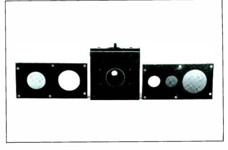
Fig. 2 — Silicon photocell housing and the sliders with color filters used in the tungsten tamp calibration. From the left, the filters shown are: green (photopic match), infrared absorbing, open aperture, red, and blue. The small light circle which may be observed in the center of the housing is the front surface of the silicon cell shown through a 1/2 in. aperture.
