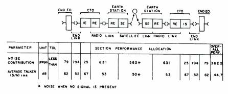
Fig. 11 - Transmission performance objectives for a private line voice channel (SCPC).
