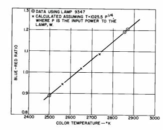
Fig. 5 — Blue-red ratio as a function of the lamp (NBS 9347) color temperature. The circled points are the blue-red value for NBS calibration temperatures. The crossed points were measured blue-red for temperature calculated from the input power to the lamp, assuming that  $T = 102.5 P^{1/4}$ , where P is the input power to the lamp, and the constant was selected for agreement with the NBS data at 2856 K.
