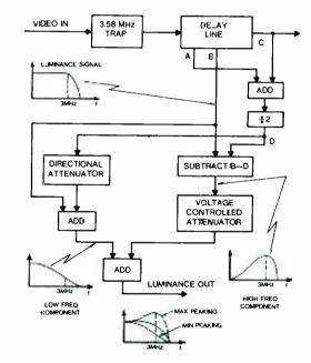
Fig. 8 — Transversal filter peaking.
