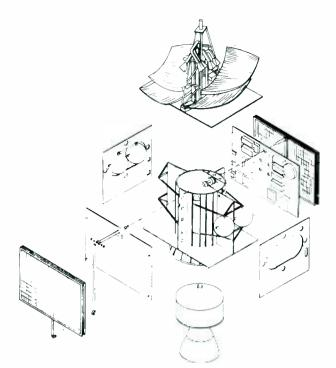
Fig. 5 - Exploded view of spacecraft.
