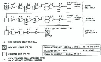
Fig. 7 — Adder hybrid measured performance.
