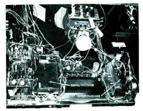
Fig. 1b - CTC-81 ColorTrak Instrument with chassis in service position.
