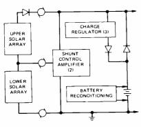
Fig. 3 — Power supply subsystem.
