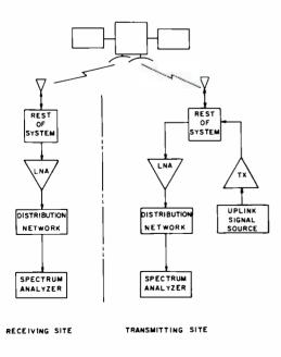
Fig. 6 — Cross polarization isolation test setup.
