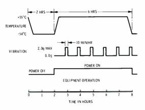
Fig. 3 --- Reliablility Growth Program test cycle.
