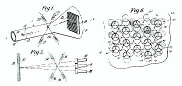
Selected figures showing three beams deflected by a single deflection yoke and the relative arrangement of mask apertures and phosphor dots that produces a nested phosphor-dot screen.
