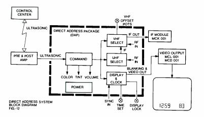
Fig. 12 — Direct address system block diagram.
