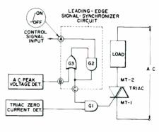
Fig. 1 — AC power control system.
